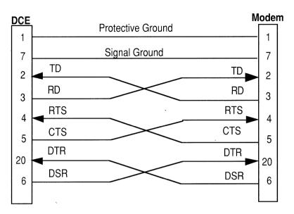
Figure B-2. Asynchronous Modified RS-232 Cable Diagram
