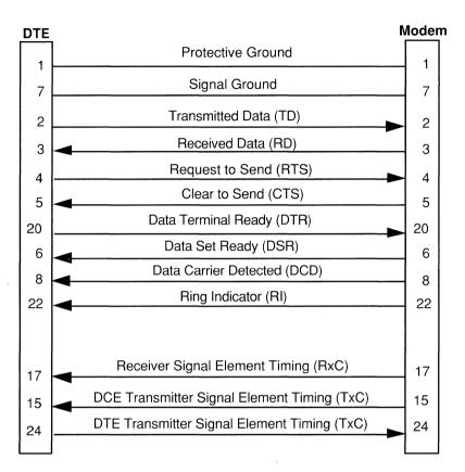
Figure B-3. Synchronous RS-232 Cable Diagram
