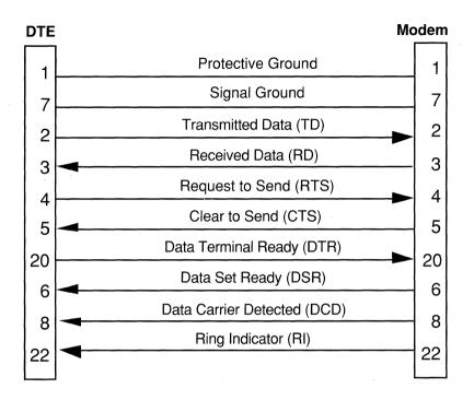
Figure B-1. Asynchronous RS-232 Cable Diagram
