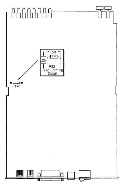
Figure C-1. Resistor R32.
