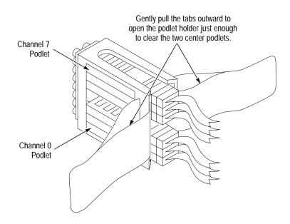
Figure C-2: Ganging the 8-channel Probe Podlets Together
