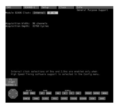
Figure 3–7: The Clock Menu with Internal Clock Window Displayed
