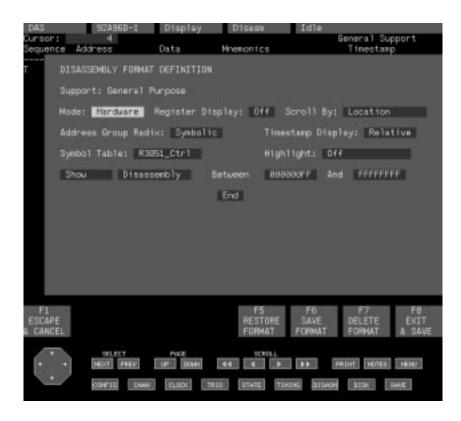
Figure 3–47: Disassembly Format Definition Overlay
