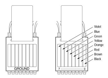
Figure 1–3: Probe Channel Color and Labels on an 8-Channel Probe
