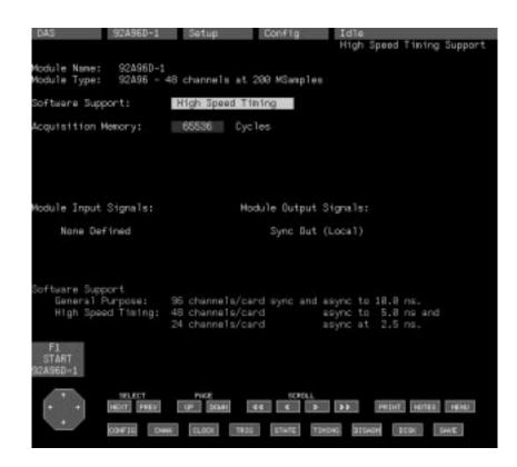
Figure 3–53: High-Speed Timing Support Is Selected In the Config Menu
