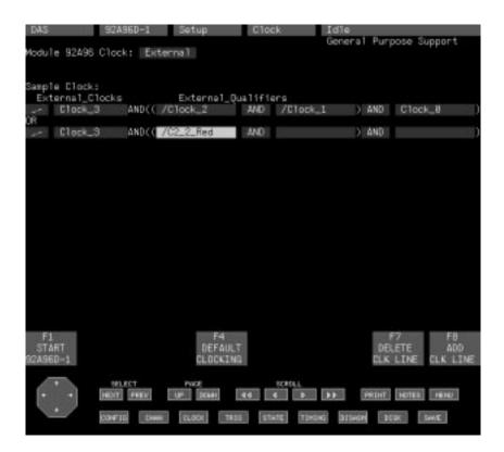
Figure 3–8: The Clock Menu with External Clock Window Displayed
