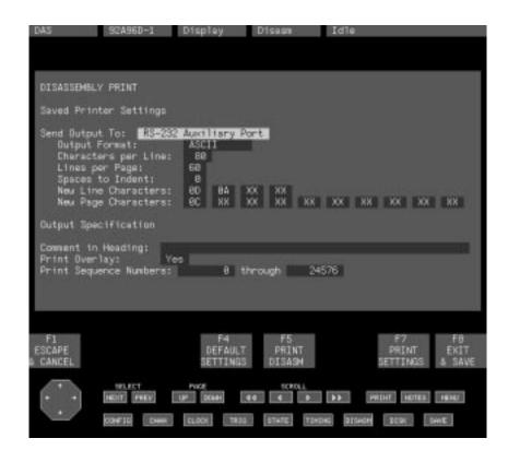
Figure 3–49: Disassembly Print Overlay
