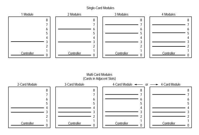
Figure 1–1: Card Placement Guidelines for Optimum Cooling
