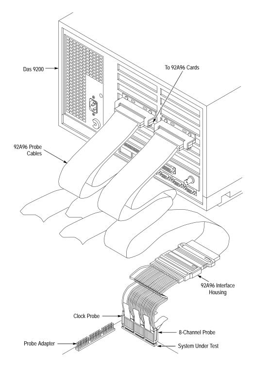
Figure 1–2: Connections to the System Under Test
