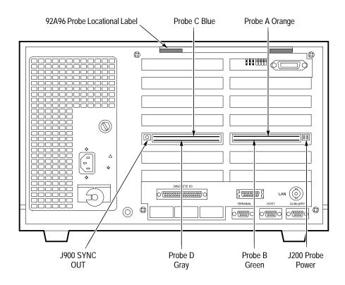
Figure 1–5: Probe Connector Locations
