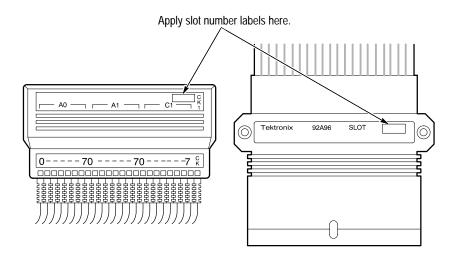
Figure 1–4: Applying Slot Number Labels
