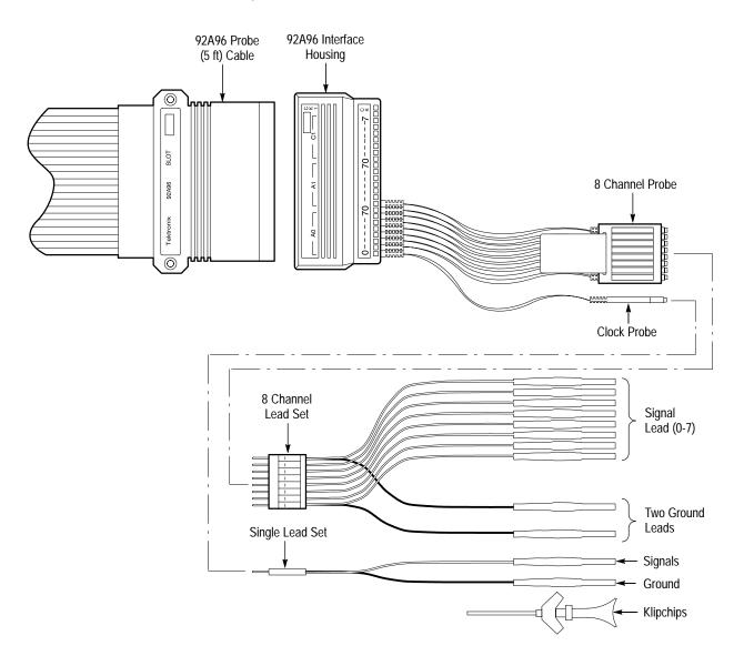
Figure 1–7: A 92A96 Probe Assembly and Lead Sets
