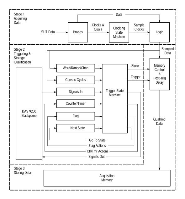
Figure 2–1: Block Diagram of 92A96 Module Acquisition and Storage
