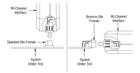
Figure 1–9: Installing a DIN Connector in your System Under Test
