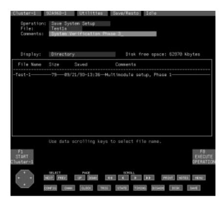
Figure 3–11: Save/Restore Menu: Save Setup Operations
