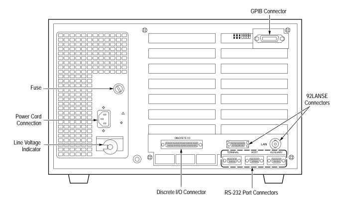
Figure 2–2: Rear View of the DAS Master Mainframe
