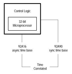
Figure 3-7: Time Correlation Between Two Acquisition Modules in a Cluster
