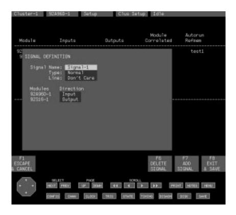
Figure 3–5: Signal Definition Overlay
