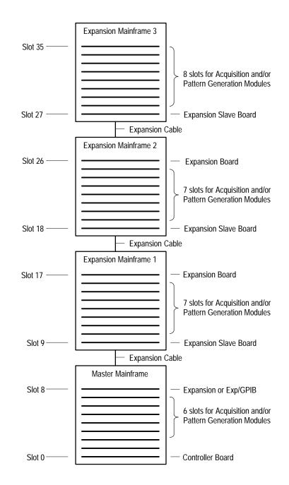
Figure 1–1: Master Mainframe and Expansion Mainframes
