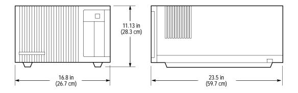
Figure A-1: Mainframe Unit Dimensions
