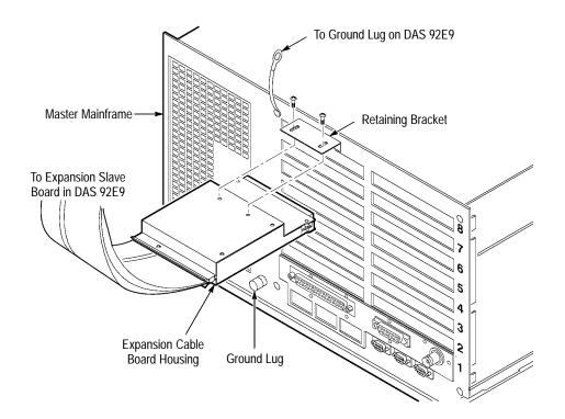
Figure 1–3: Master and Expansion Mainframe Connections
