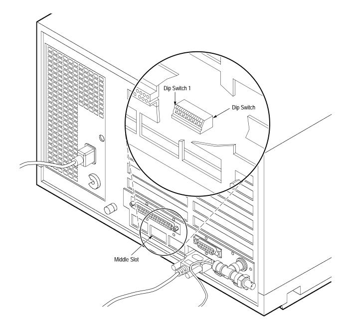
Figure D–1: DIP Switch Location
