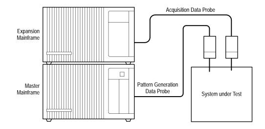
Figure 1–2: Expansion Mainframe Stacked on Master Mainframe
