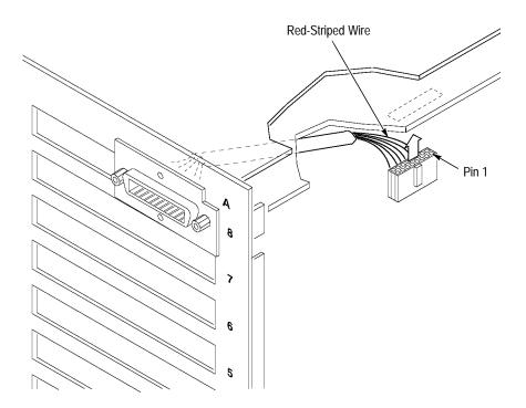
Figure F-5: Installing the GPIB Connector
