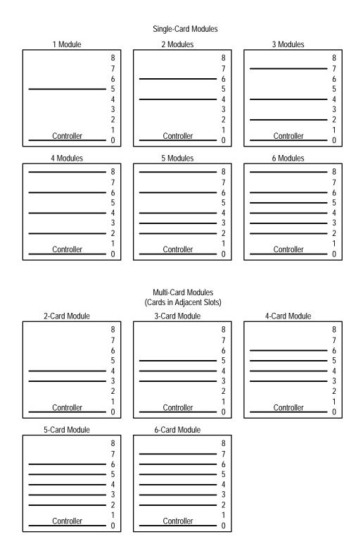
Figure F-1: Module Placement in the Master Mainframe
