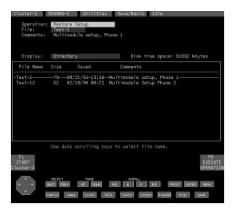
Figure 3–13: Save/Restore Menu: Restore Setup Operations
