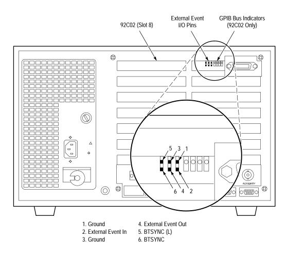
Figure 3–6: 92C02 Module External Event Pins
