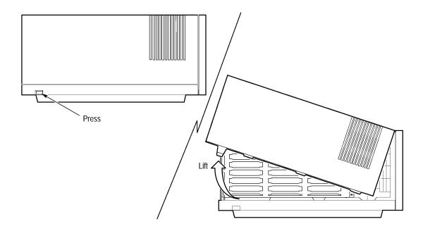
Figure F–3: Removing the Mainframe Top Cover
