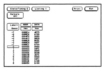
Figure 3 - 6. State Listing Menu with Off-screen Data
