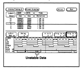
Figure 12-20. Mixed Mode Display with Unstable Data
