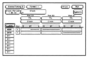
Figure 8-8. Format Specification with Bits Assigned
