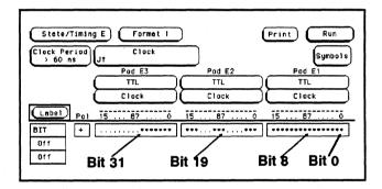
Figure 5-10. Numbering of Assigned Bits
