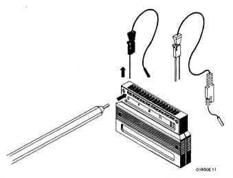
Figure 2-8. Disconnecting Probes from Pods
