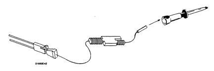
Figure 2-9. Connecting Grabbers to Probes
