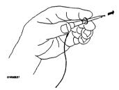
Figure 2-10. Connecting Grabbers to Test Points
