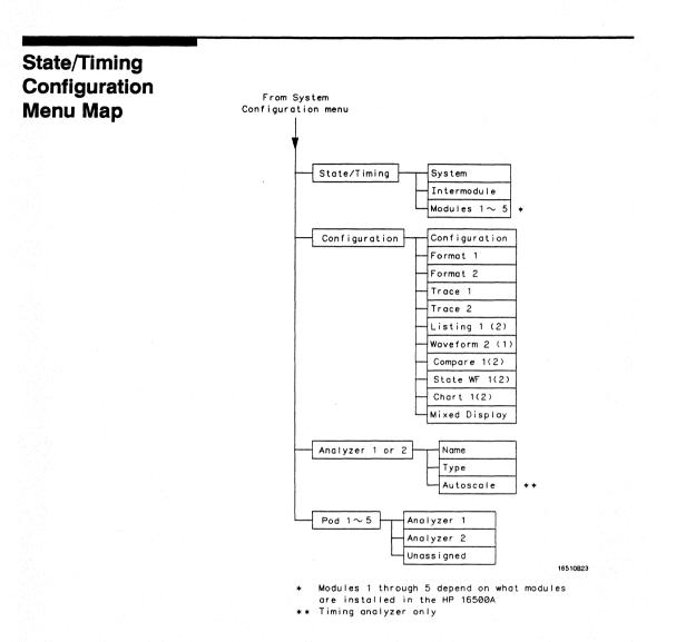
Figure 4-1. State/Timing Configuration Menu
