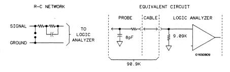
Figure 2-5. Probe Input Circuit
