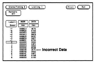
Figure 8-23. State Listing showing Incorrect Data
