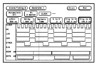
Figure 6-9. Trigger and Trace Points
