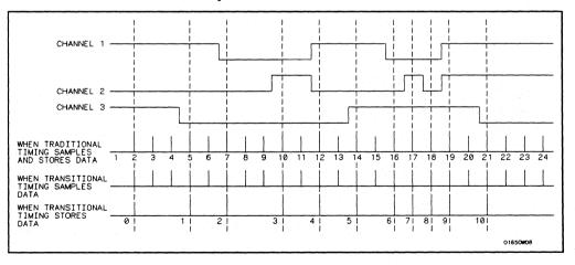
Figure 5-32. Transitional Timing vs. Traditional Timing
