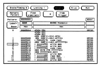
Figure 14-2. Inverse Assemble Field
