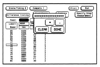
Figure 9-2. Bit Masking Fields
