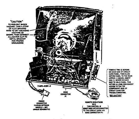
Figure 4. Circuit Card Troubleshooting from Component Side
