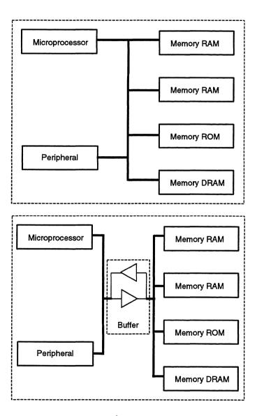
Figure 2-1 Dividing a long bus and adding buffers
