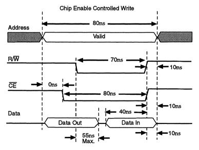
Figure 6-1 NetROM write-timing diagram
