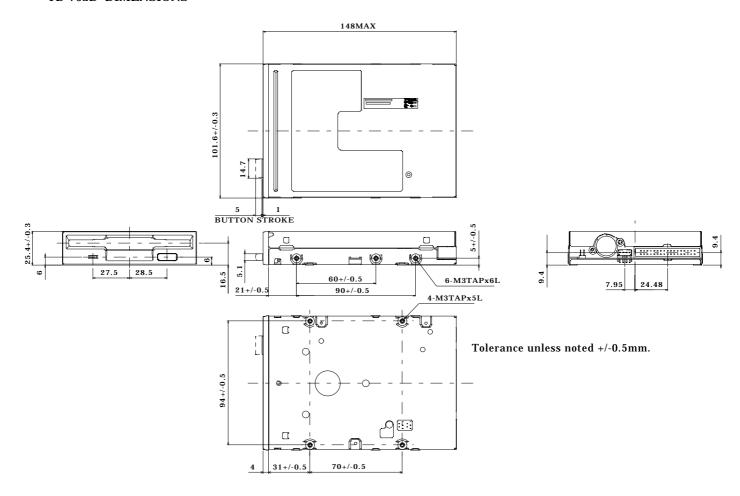
Fig.5.1 Mechanical Dimensions
