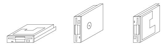
Recommended angle of the drive when the drive is installed is less than +30 degrees. Fig. 5.2 Recommended Mounting
