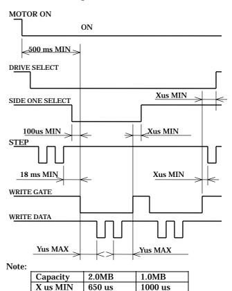
Fig.3.12 Write Timing
