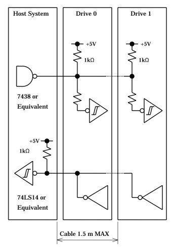
Fig.3.7 Interface Circuit
