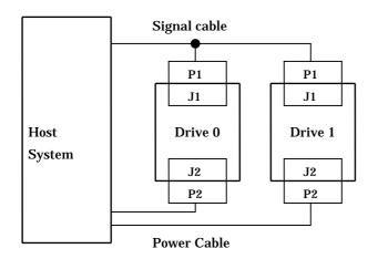
Fig.4.1 Cable Connections
