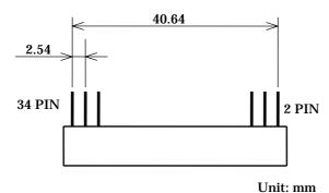
Fig.4.2 J1 Connector Dimensions
