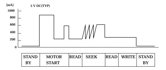
Fig 3.13 Current Waveform
