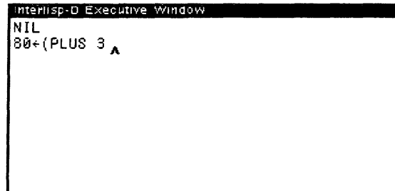
Figure 1.2. The caret is to the right of the number 3. When a character is typed at the keyboard, it will appear at the caret
