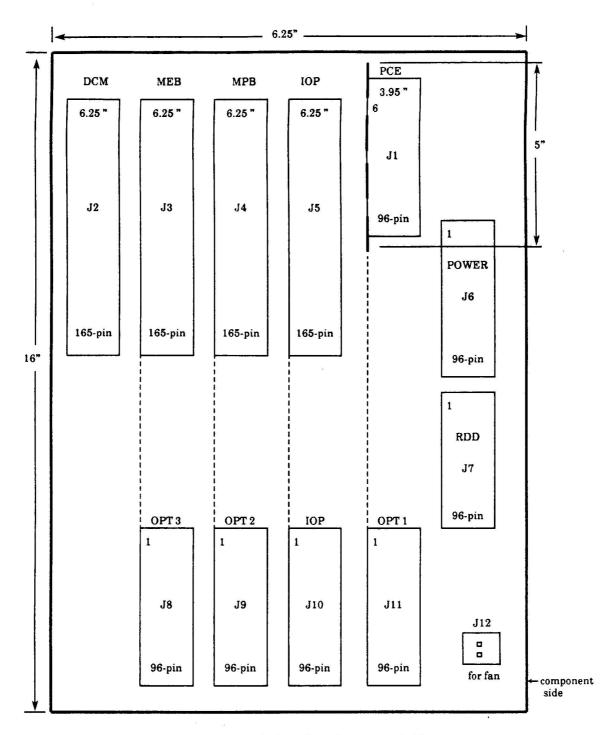
Figure 1.2. Backplane from logic board side
