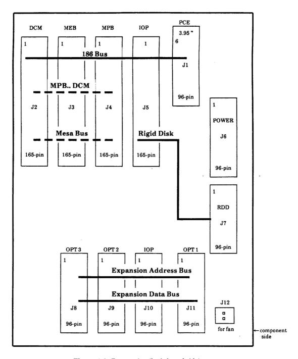
Figure 1.3. Bus routing (logic board side)
