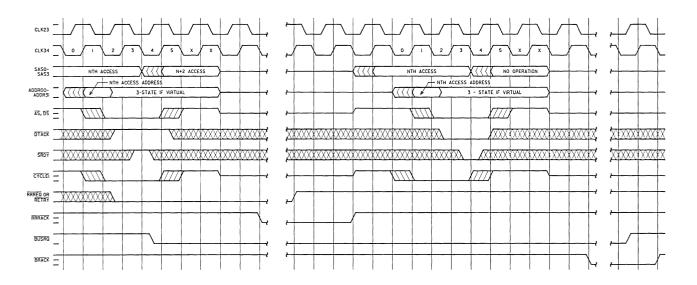
Note: The same protocol diagram applies for retry and bus arbitration except that the address bus, data bus, and control signals are not 3-stated during the time  $\overline{\text{RETRY}}$  is active and  $\overline{\text{RRRACK}}$  is not issued.
