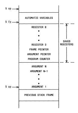
Figure 5-3. Typical Stack Frame for a Function Call
