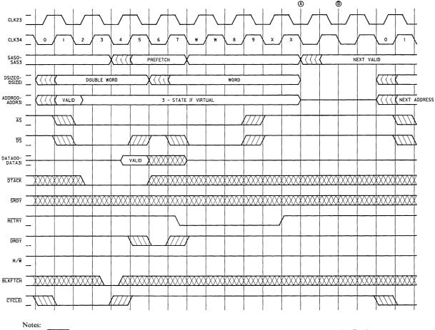
1. On <u>RRREQ</u>, the following pins are 3-stated between points A and B. ADDR00- ADDR31, DATA00-DATA32, AS, <u>CYCLEI</u>, <u>DRDY</u>, <u>DS</u>, DSIZE0-DSIZE1, R/W, SAS0-SAS3.
