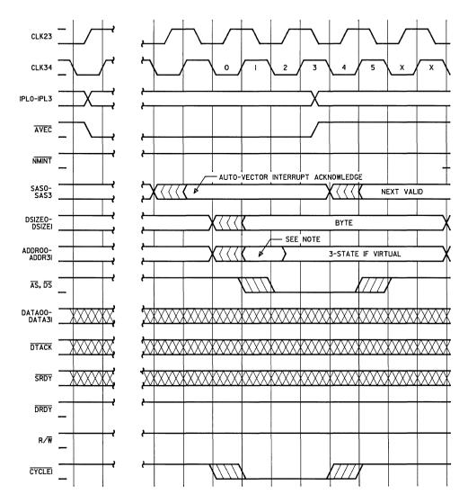
Note: During the interrupt acknowledge the address bus (ADDR00-ADDR31) contains the following data.
