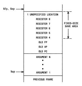
Figure 5-5. Stack Frame After Three Registers are Saved
