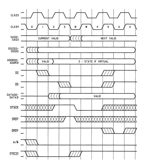
Figure 2-14. Write Transaction With One Wait Cycle (Using DTACK)
