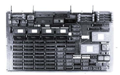
Figure 1-3. WE 321EB Microprocessor Evaluation Board
