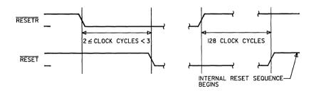
Note: RESETR must be asserted for at least two clock cycles to be recognized. RESET is negated 128 clock cycles after negation of RESETR.
