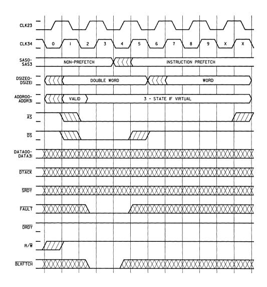
Figure 2-25. Fault on First Word of Blockfetch Transaction With Access Status Code (Not Instruction Prefetch)
