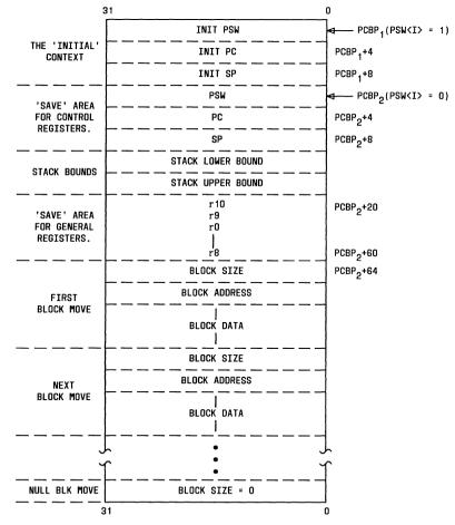
Figure 4-1. A Typical Process Control Block
