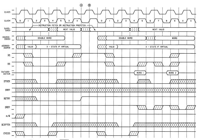
Note: If RRREQ is asserted instead of RETRY, the CPU 3-states the bus at A and asserts RRRACK one clock cycle later at B.
