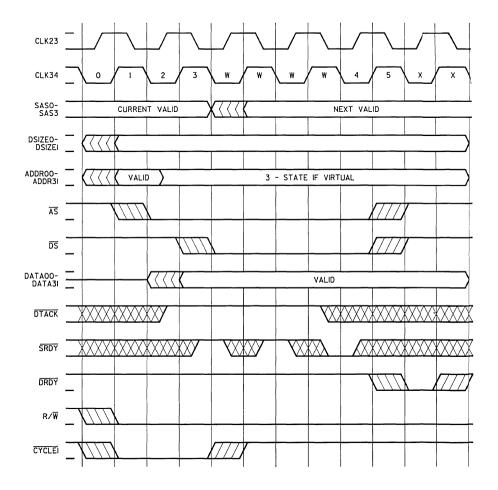
Figure 2-13. Write Transaction With Two Wait Cycles (Using SRDY)
