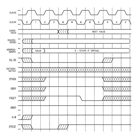
Figure 2-20. Asynchronous Fault Without DTACK and SRDY (Read Transaction)
