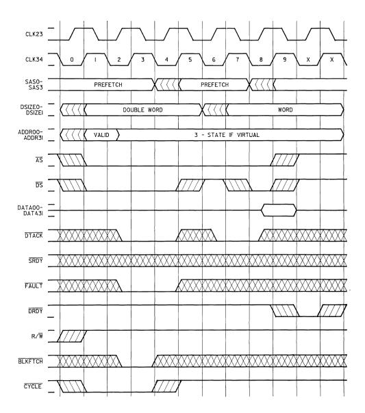
Figure 2-26. Fault on First Word of Blockfetch Transaction With Access Status Code of Prefetch
