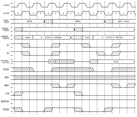
Figure 2-45. Read Transaction Followed by a Write Transaction (Using DTACK)
