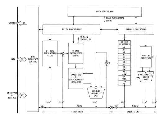
Figure 2-1. WE 32100 Microprocessor Block Diagram
