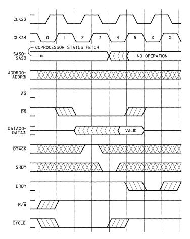
Note: Coprocessor status fetch begins approximately two clock cycles after the microprocessor's processor done input  $(\overline{DONE})$  has been driven low.
