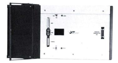
Figure 1-2. WE 321AP Microprocessor Analysis Pod
