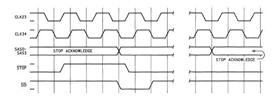
Note:  $\overline{BARB} = 0$  and  $\overline{BRACK} = 1$  in order to see stop acknowledge access status code.
