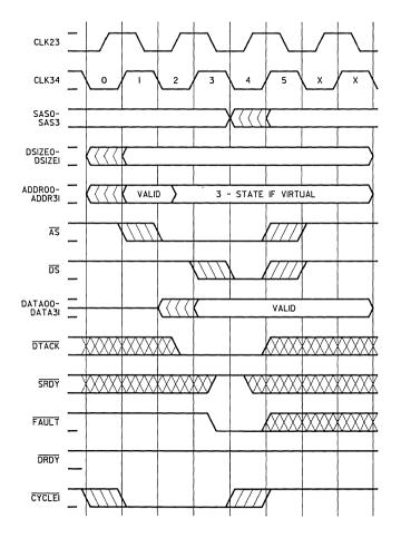
Note:  $\overline{FAULT}$  must meet setup time with respect to CLK34 edge after assertion of  $\overline{DTACK}$ .
