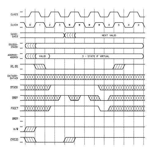
Figure 2-21. Fault with Synchronous Ready (SRDY); i.e., Synchronous Fault
