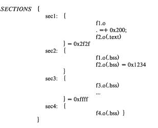
In this example, the 0x200 byte hole in section sec1 is filled with WAIT instructions (0x2f2f). In the section sec2, fl.o(.bss) is initialized to the default fill value of 0x00, and f2.o(.bss) is initialized to 0x1234. All **.bss** sections within sec3 as well as holes are initialized to 0xffff. Section sec4 is not initialized (i.e., no data are written to the object file for sec4).
