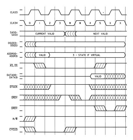
Figure 2-9. Read Transaction With One Wait Cycle (Using SRDY)
