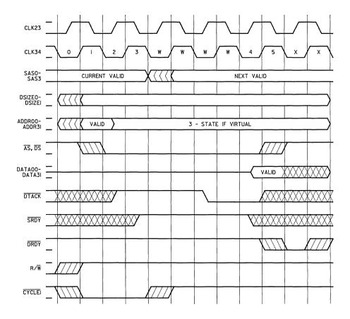
Figure 2-10. Read Transaction With Two Wait Cycles (Using DTACK)
