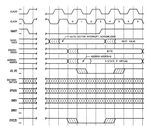
Note: The address bus ADDR00-ADDR31 contains all zeroes during the acknowledge of a nonmaskable interrupt.
