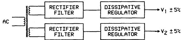
Figure 24-2 - AC Line-Operated Rectifier Block Diagram
