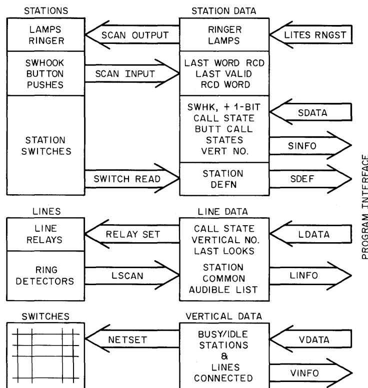
Figure 21-13 - System Data Buffering
