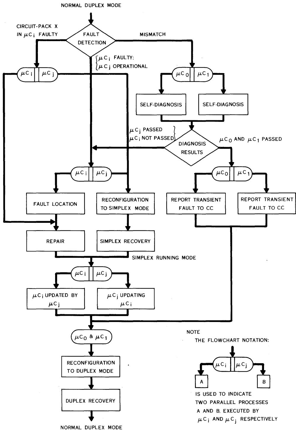
Figure 15-3 - Maintenance Functions
