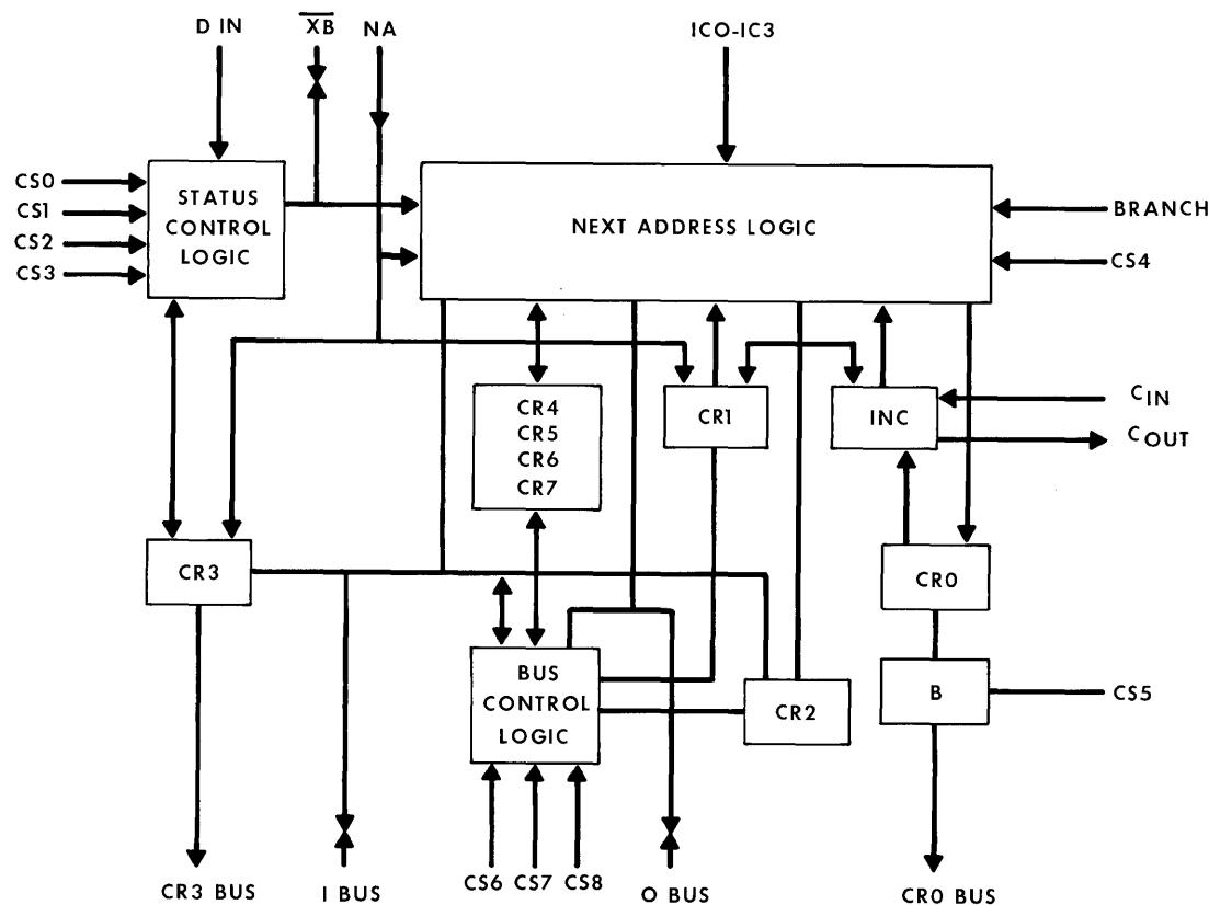
Figure 16-3 - Microprogram Control Function
