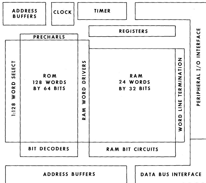
Figure 27-2 - Preliminary Placement of ROM-RAM-I/O Functions on LSI Chip
