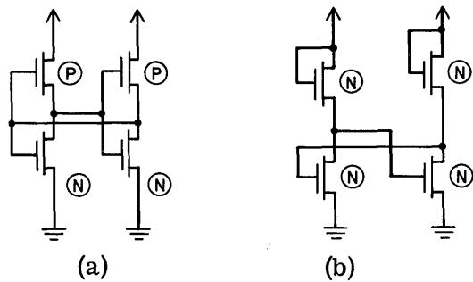
Figure 3-2 - CMOS and NMOS Memory Elements
