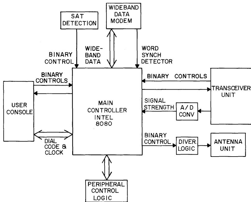
Figure 14-1 - Mobile Logic System
