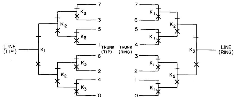
NOTE: WHEN NO TRUNK IS CONNECTED, THE K<sub>1</sub>, K<sub>2</sub>, AND K<sub>3</sub> RELAYS ARE LATCHED:
