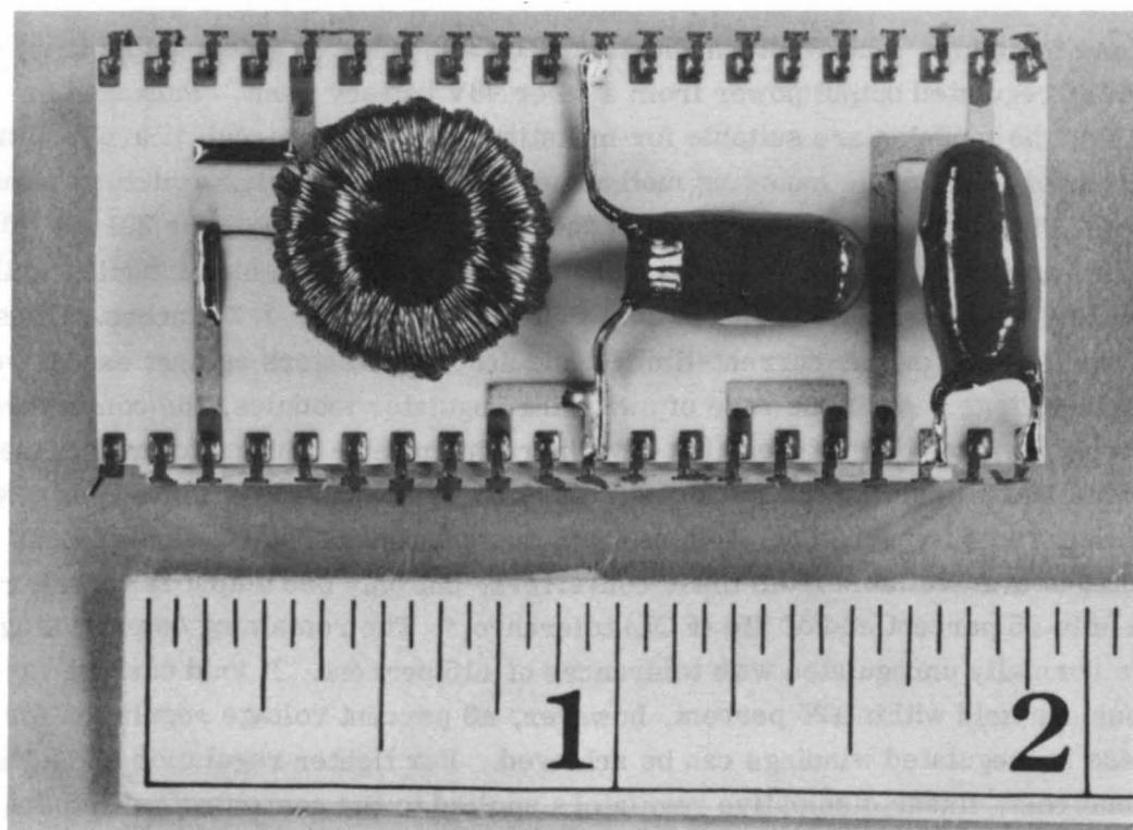
Figure 24-4 - 12V 70 mA DIP-Switching Regulator
