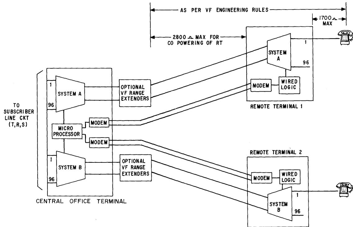
Figure 12-2 - Typical LSS System Layout - Two RTs
