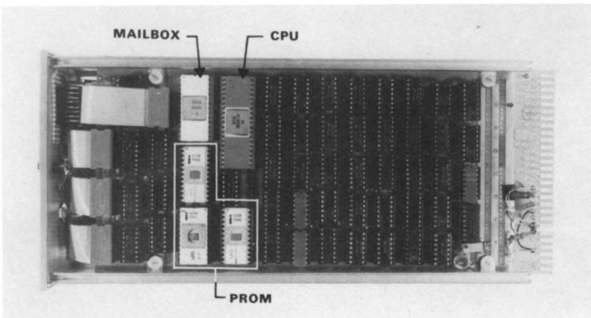
Figure 18-2(c) - Processor "One": CPU Board
