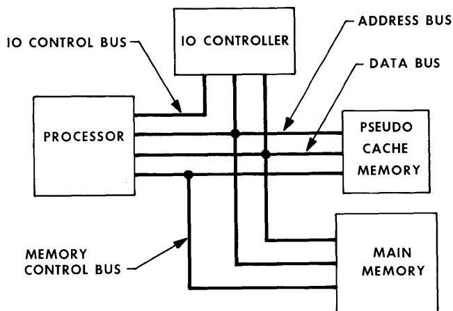
Figure 16-1 - System Structure
