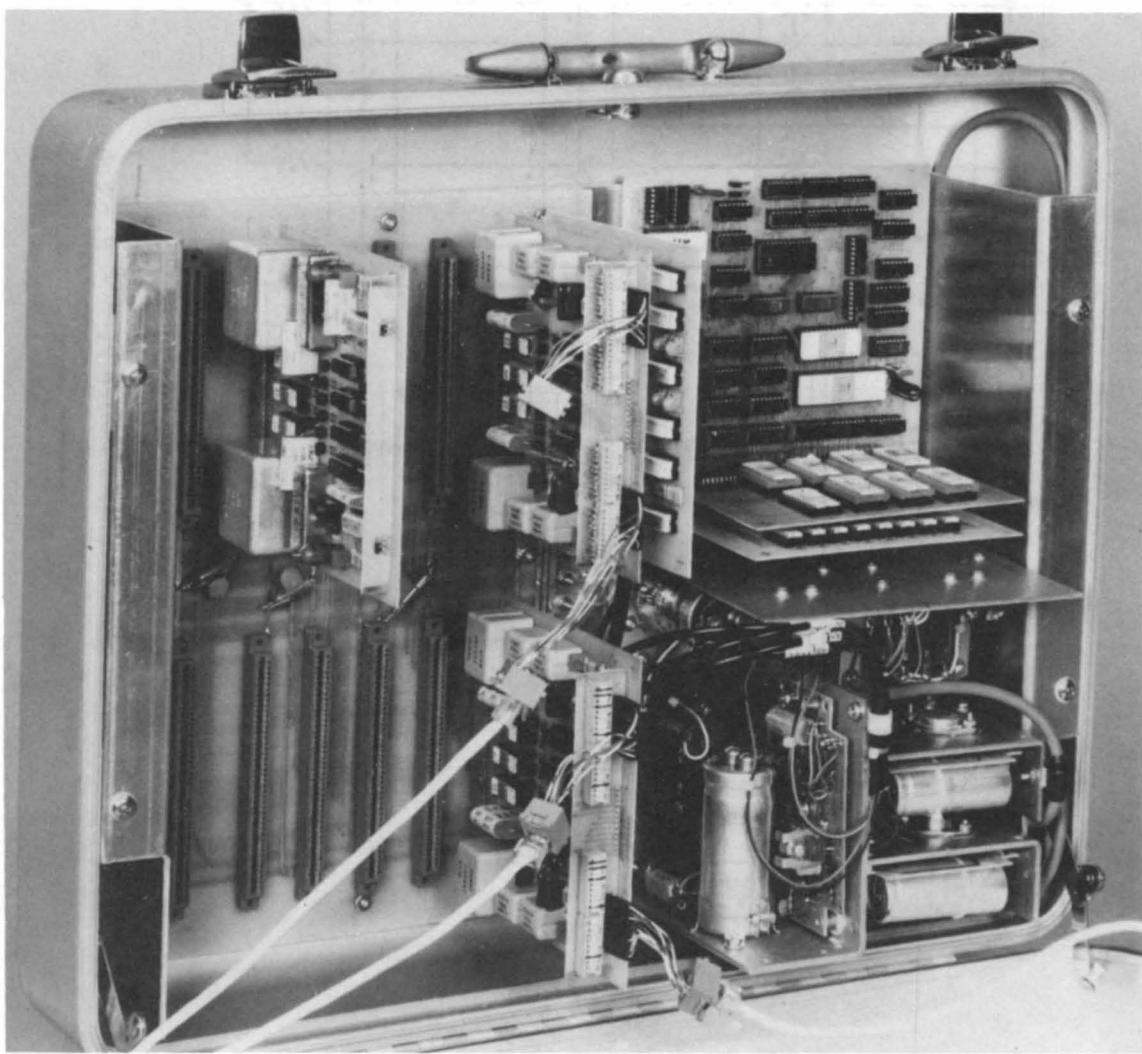
Figure 21-2 - Printed Circuit Card Arrangement
