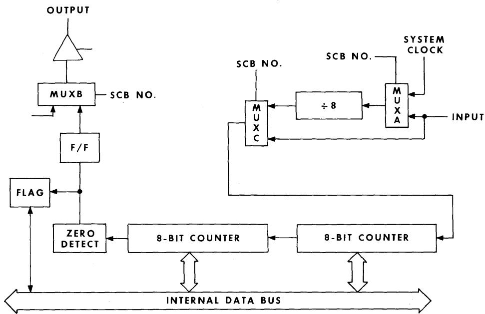
Figure 27-3 - Internal Timer Functions
