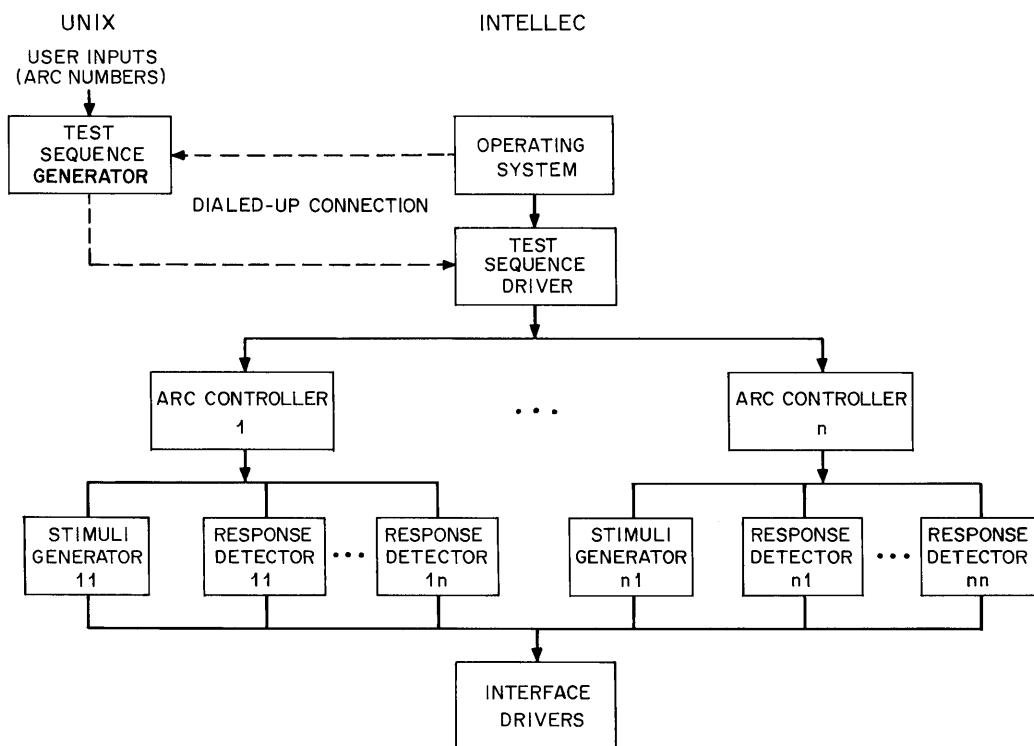
Figure 14-4 - Software Structure
