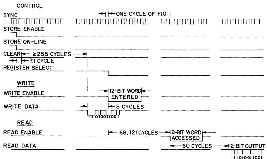
Figure 26-2 - SBS Register Sequencing
