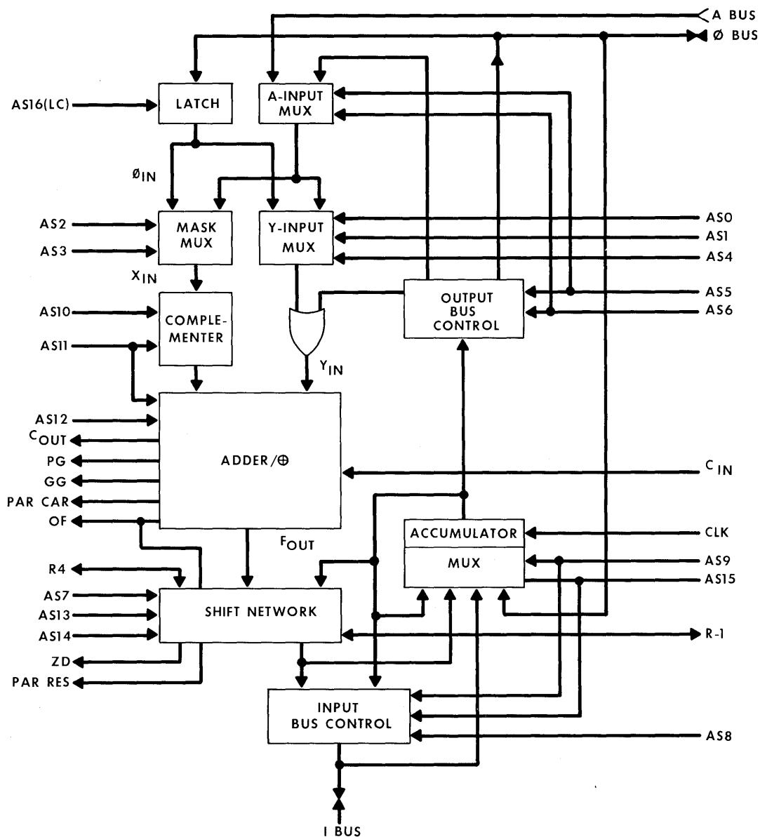
Figure 16-2 - Arithmetic Logic Unit
