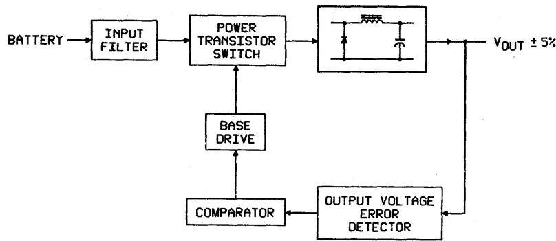
Figure 24-3 - Switching Regulator Block Diagram
