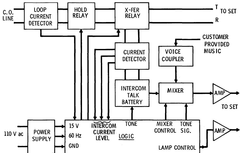
Figure 23-2 - SLS Controller Block Diagram
