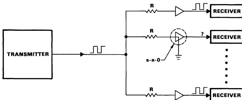
Figure 15-7 - Isolation of Input Faults
