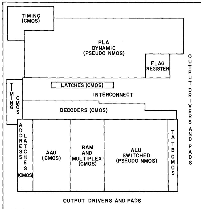
Figure 3-1 - Block Diagram of Chip
