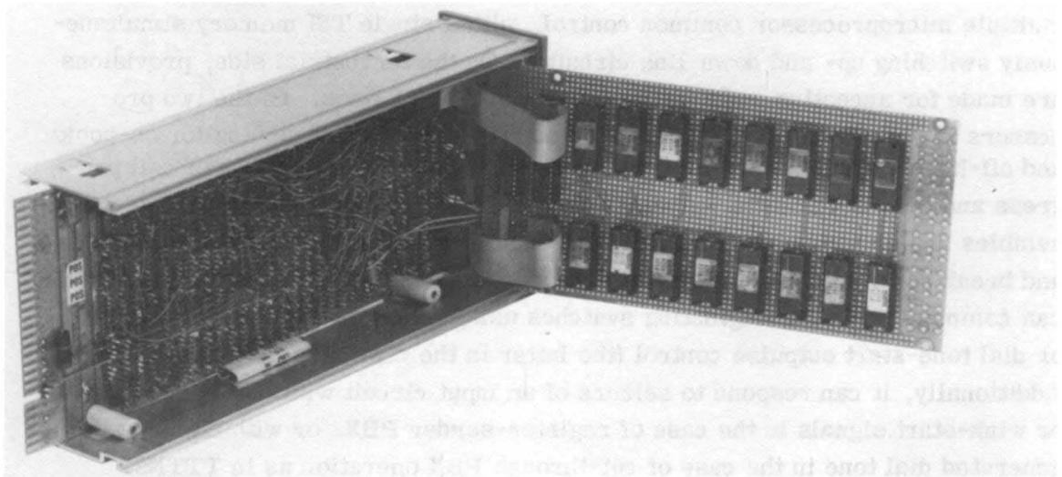
Figure 18-2(b) - Processor "One": RAM Board
