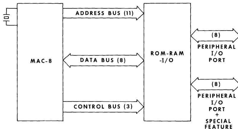
Figure 27-1 - Interconnection of a Single ROM-RAM-I/O Device
