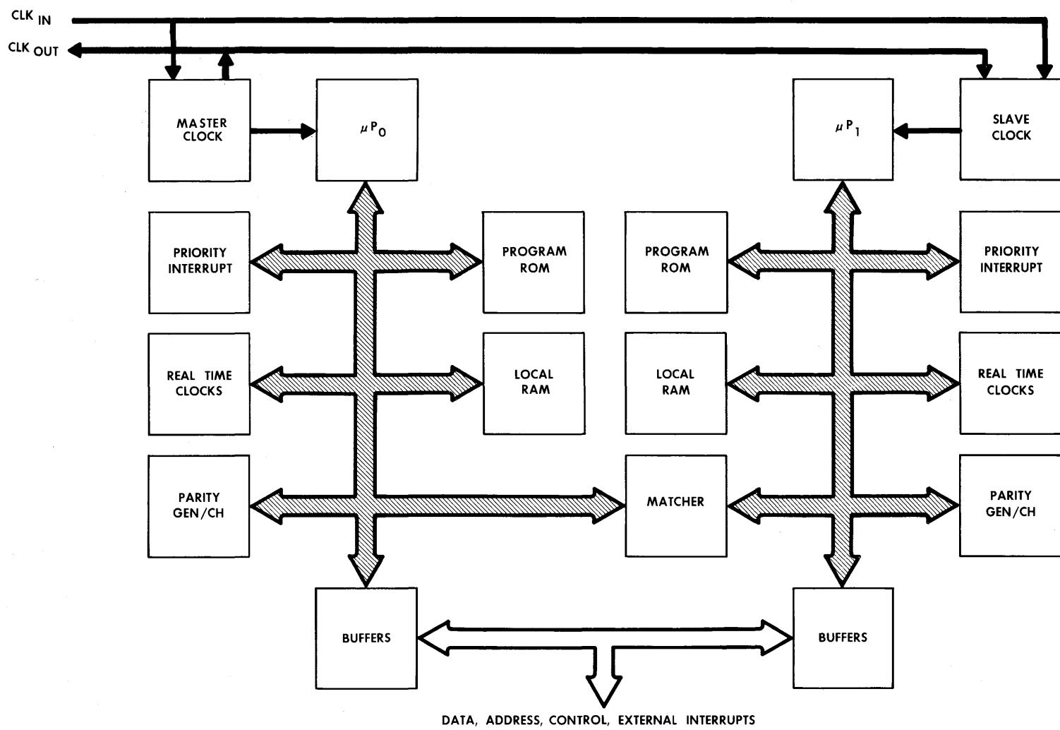
Figure 15-4 - Hard Core Block Diagram
