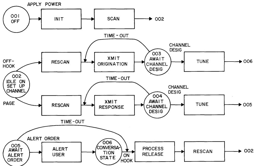
Figure 14-3 - Simplified State Diagram
