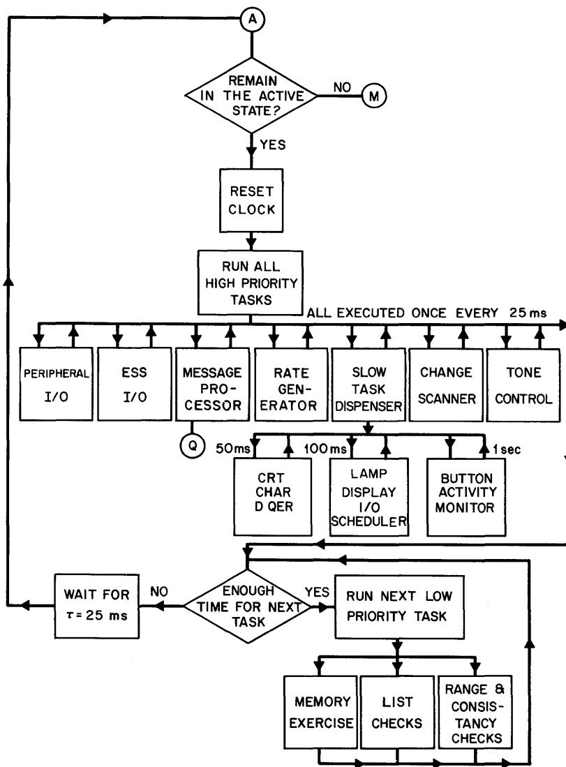
Figure 22-3 - RDI Software Flow Diagram
