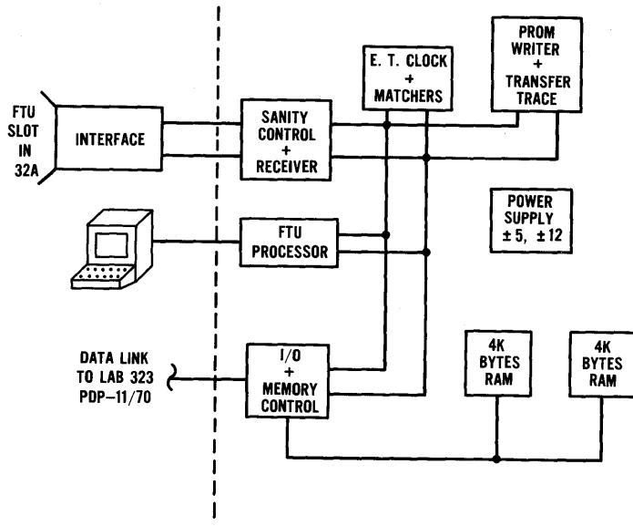
Figure 8-3 - Field Test Unit
