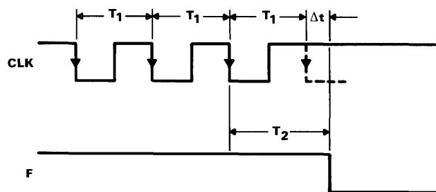
Figure 15-6 - Clock Fault Detection
