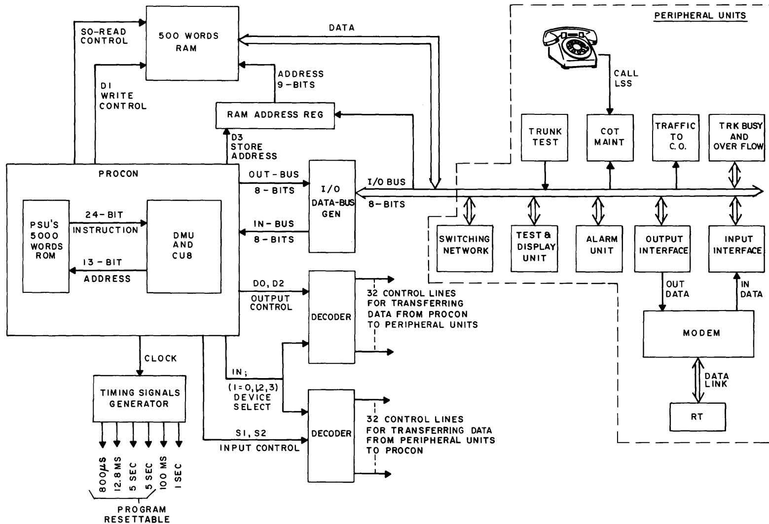
Figure 12-6 - Block Diagram Showing Communication Paths
