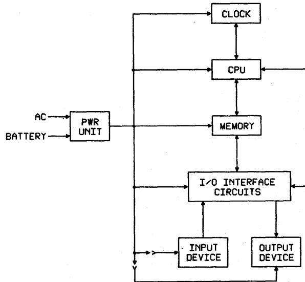
Figure 24-1 - Typical Microprocessor System
