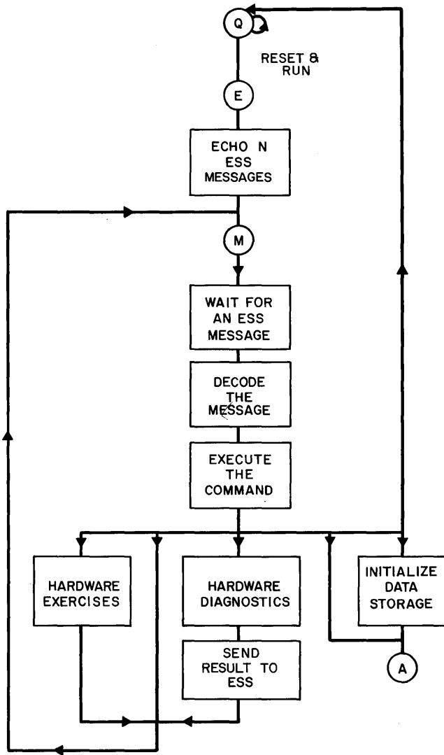
Figure 22-2 - RDI Software Flow Diagram
