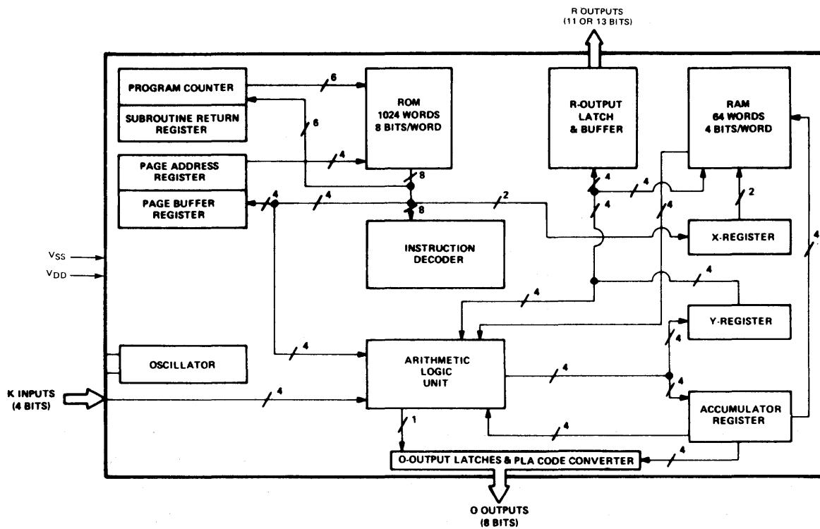
Figure 23-4 - TMS 1000 Computer Block Diagram
