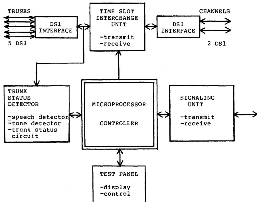
Figure 13-1 - TASI-E Microprocessor Interfaces
