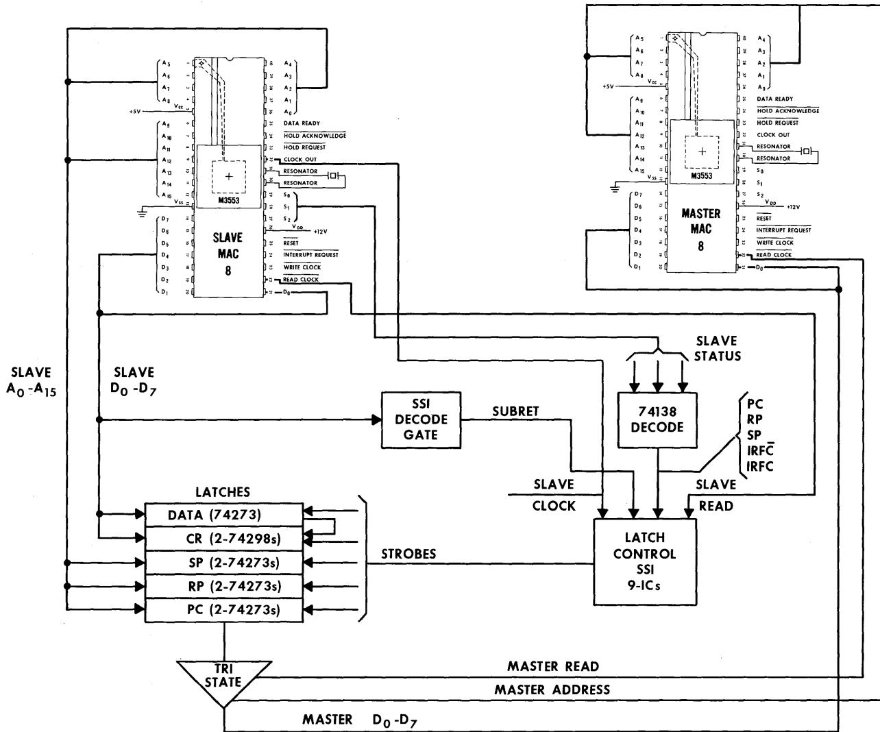
Figure 5-7 - Snapshotting MAC-8 Registers
