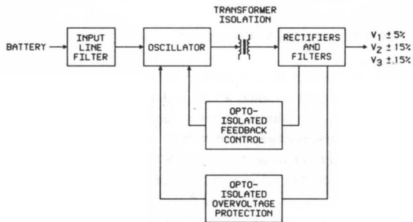
Figure 24-5 - DC-to-DC Converter Block Diagram
