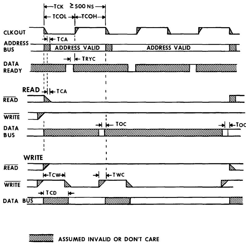
Figure 2-2 - Preliminary Timing Waveforms
