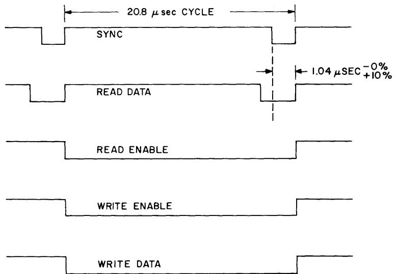
TRANSITION TIMES OF READ ENABLE, WRITE ENABLE AND
