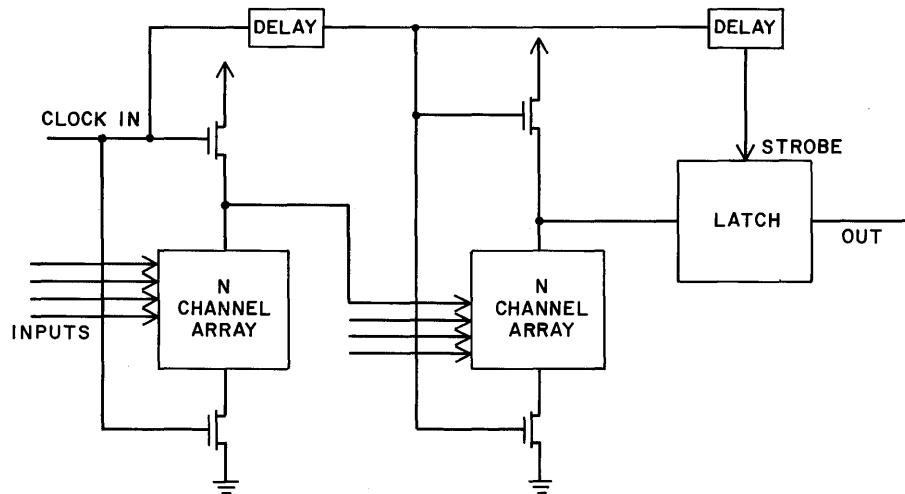
Figure 3-5 - PLA Block Diagram
