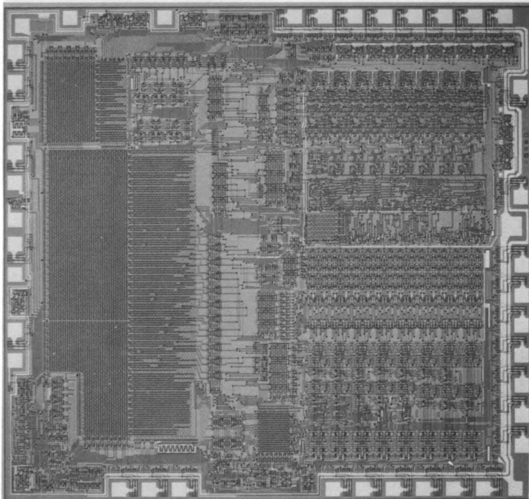
Figure 3-6 - The MAC-8 Microprocessor Chip
