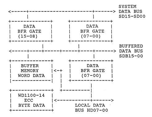
FIGURE 5-10 R/W DATA TRANSFER PATH FIXED DISK SECTION
