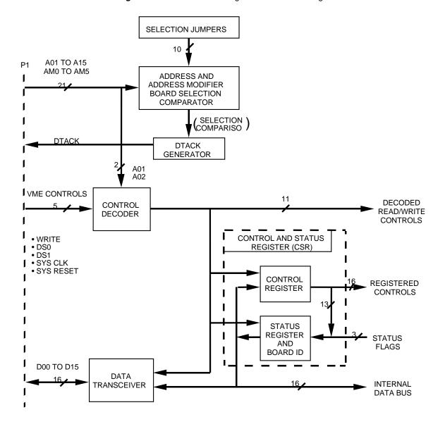
Figure 1-2 VMEbus Control Signals and Interface Logic
