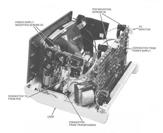
Figure 7-2. PCB Mounting
