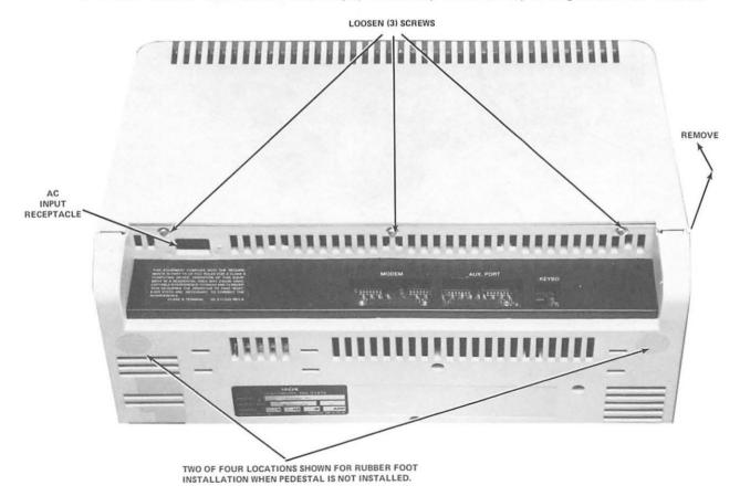
Figure 7-1. Top Cover Removal
