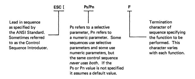
The following examples demonstrate the use of all three elements of the control sequence as specified by the ANSI X3.64 standard. Spaces are used for clarity only are not part of the sequence.
