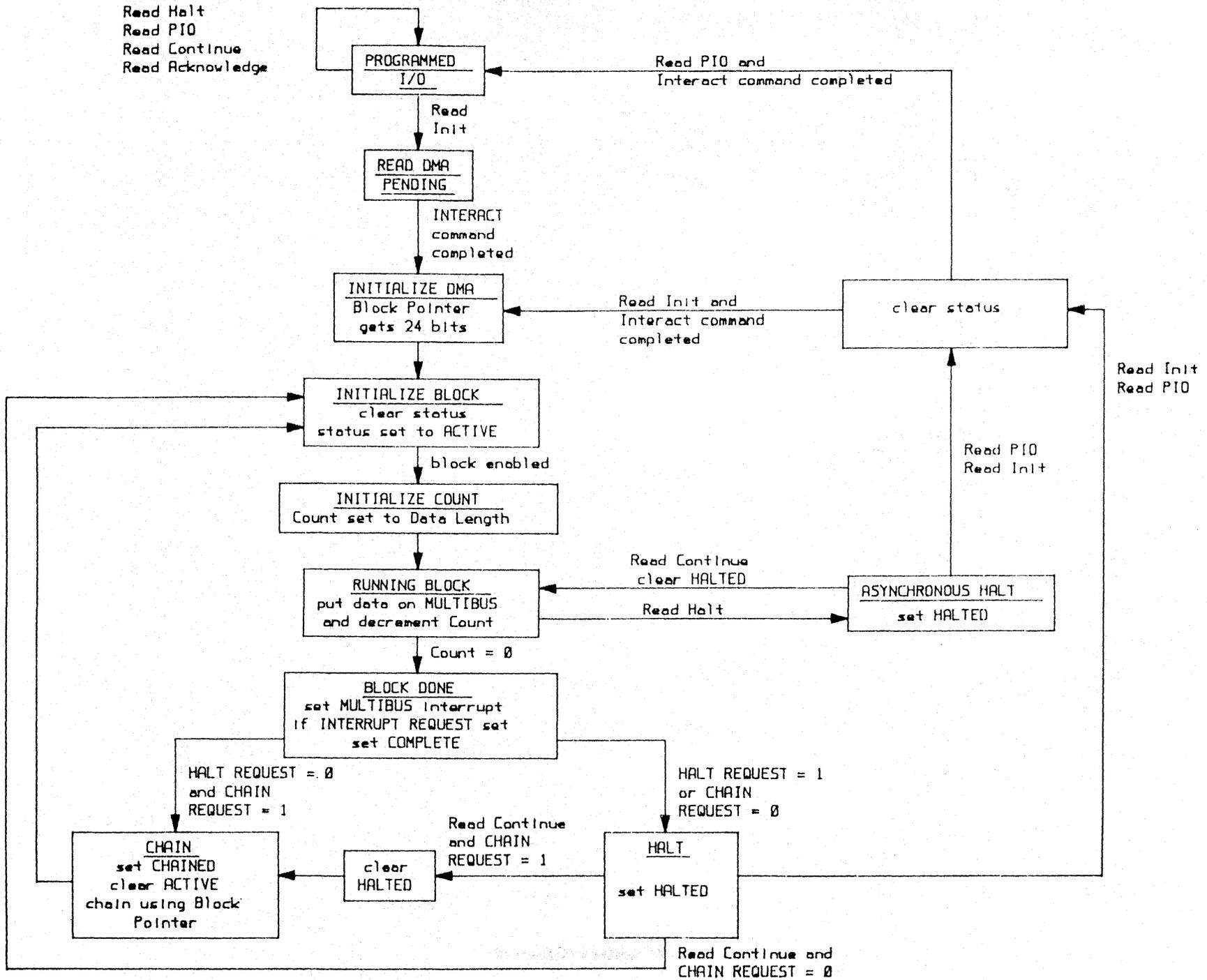
Figure 5.5 : DMA Read State Diagram
