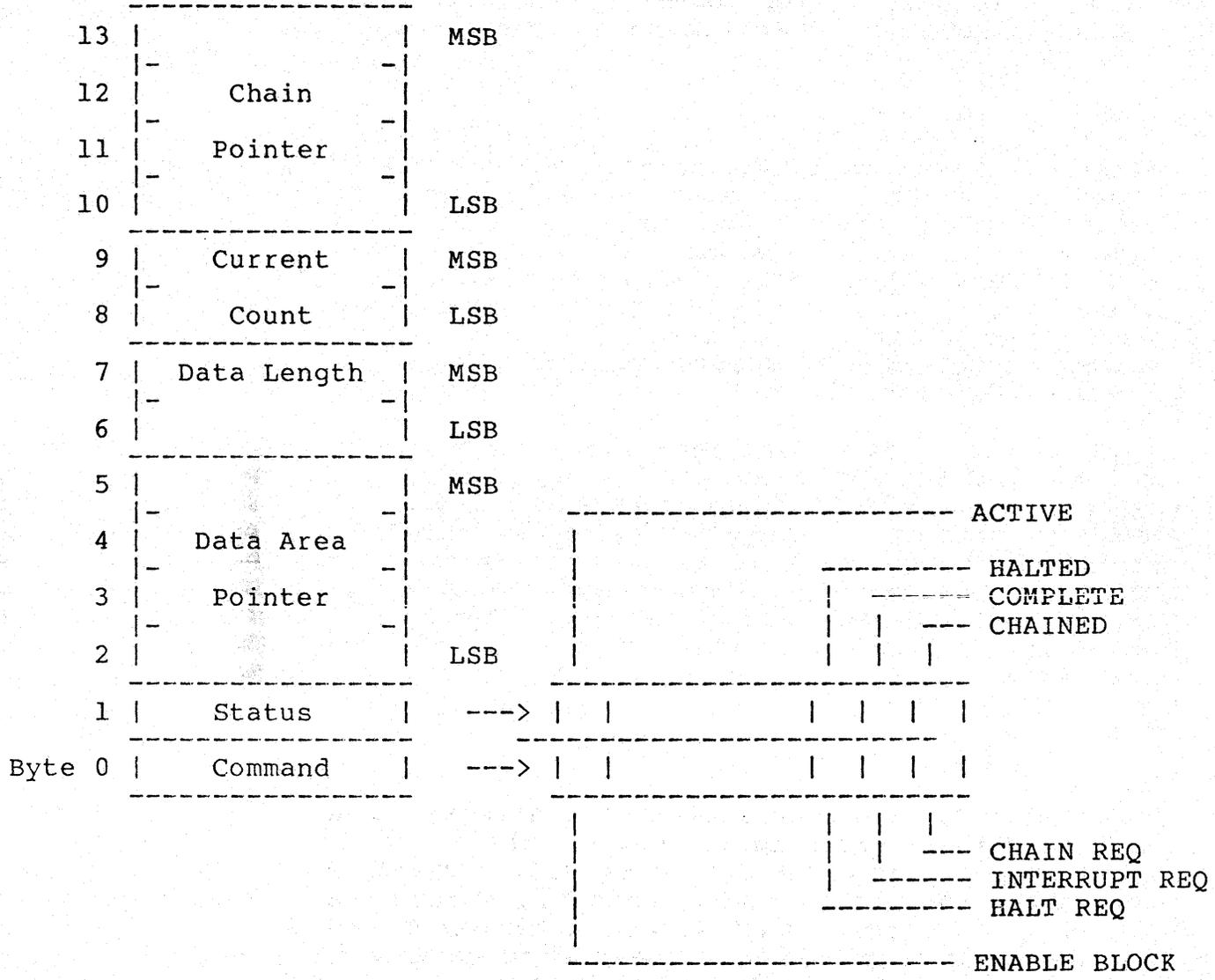
Figure 5.3 : DMA Block Header
