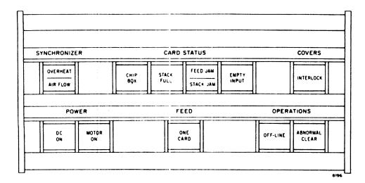
Figure 8-3. Card-Punch Control Panel
