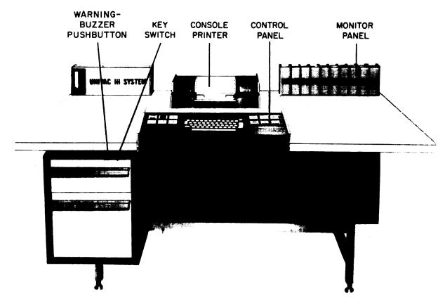
Figure 3-1. Operator's Console Model 124
