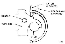
Figure 3-6. Type-Box Latch Operation
