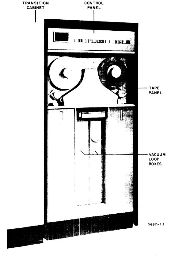
Figure 5-1. UNISERVO IIA Maanetic-Tape Unit Model 72 and Transition Cabinet
