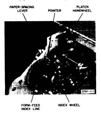
Figure 3-4. Console Printer, Rear View
