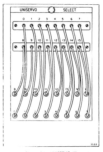
Figure 4-8. UNISERVO III lape-Unit-Select Patch Panel
