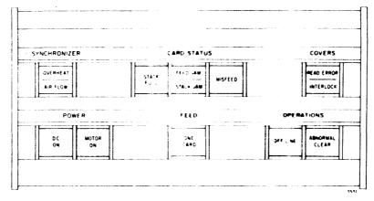
Figure 7-3. Card-Reader Control Panel
