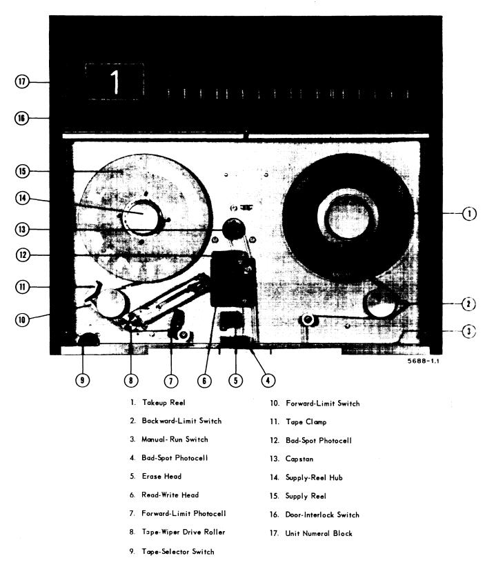
Figure 5-2. UNISERVO IIA Tape Panel and Control Panel
