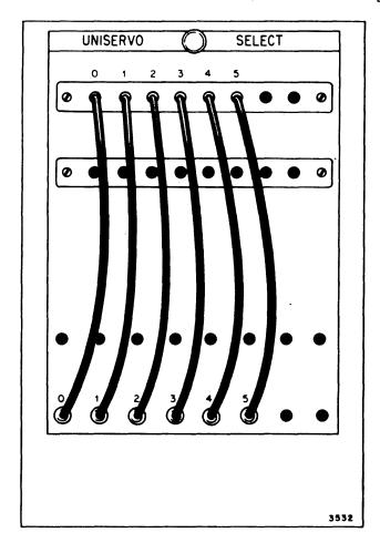
Figure 5-8. UNISERVO IIA Tape-Unit-Select Patch Panel
