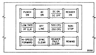
Figure 11-5. Reader Control Panel
