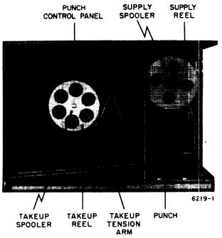
Figure 11-4. Punch, and Takeup Spooler Panel
