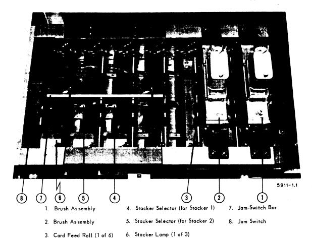
Figure 7-6. Stackers, Top View
