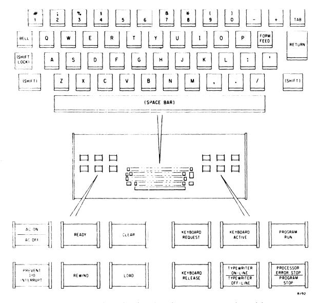
Figure 3-2. Control Panel and Keyboard, Operator's Console Model 124
