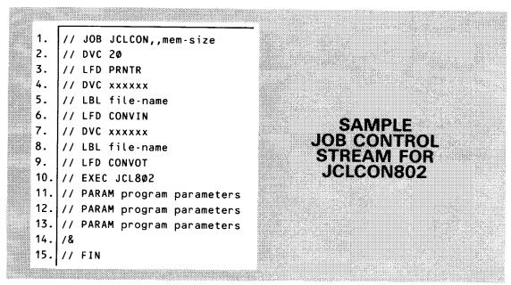
Line 1 names the job and specifies to the system how much memory is needed to execute it. The job name doesn't have to be JCLCON; it can be any name you choose.
