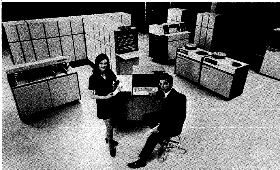
This view of a fairly small, disc-oriented UNIVAC 90/70 configuration shows the CRT-equipped System Console in the foreground and the Central Processor at left rear.
