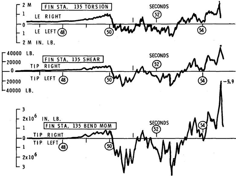
Figure 6. Severe turbulence effects, B-52 flight test.
