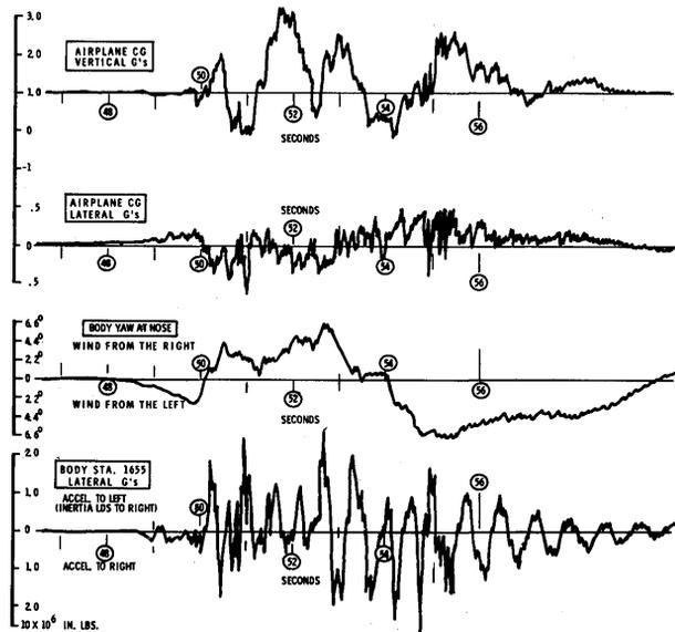
Figure 5. Severe turbulence effects, B-52 flight test.
