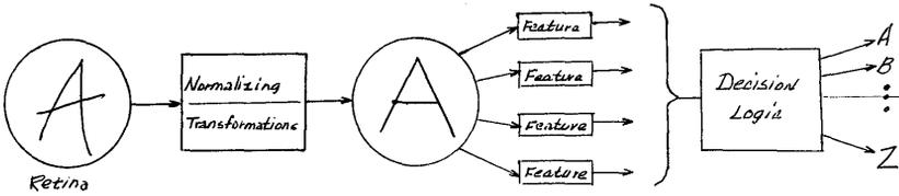
Figure 5. Schematic pattern recognizer.
