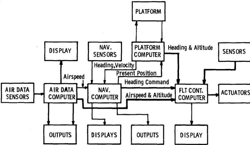
Figure 13. Integrated microelectronic avionic system.
