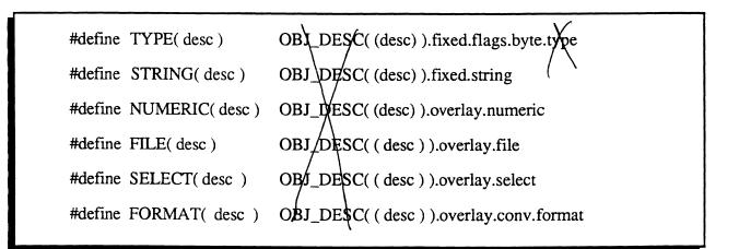
There will definitely be more definitions in that file as the  $desc\_struct$  structure evolves. The concept though should remain the same. Notice that we practically can get to any field in the structure by using a reference of the form **DESC\_type( ARG( n ) ).field**. That makes it consistent throughout the code.
