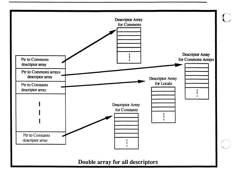
One significant advantage of this data structure is how **call** becomes simplified with respect to handling local variables. To give the program a new set of local variables, all that has to happen is save the address of the caller's local variables descriptor table and make the corresponding entry in the first array point to a newly allocated callee local variables descriptor table.
