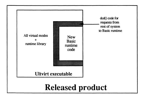
The way this is going to be done is by splitting the new opcodes (just for the purposes of development) into a separate executable that is a lot easier to link (a few seconds compared to a many minutes!).
