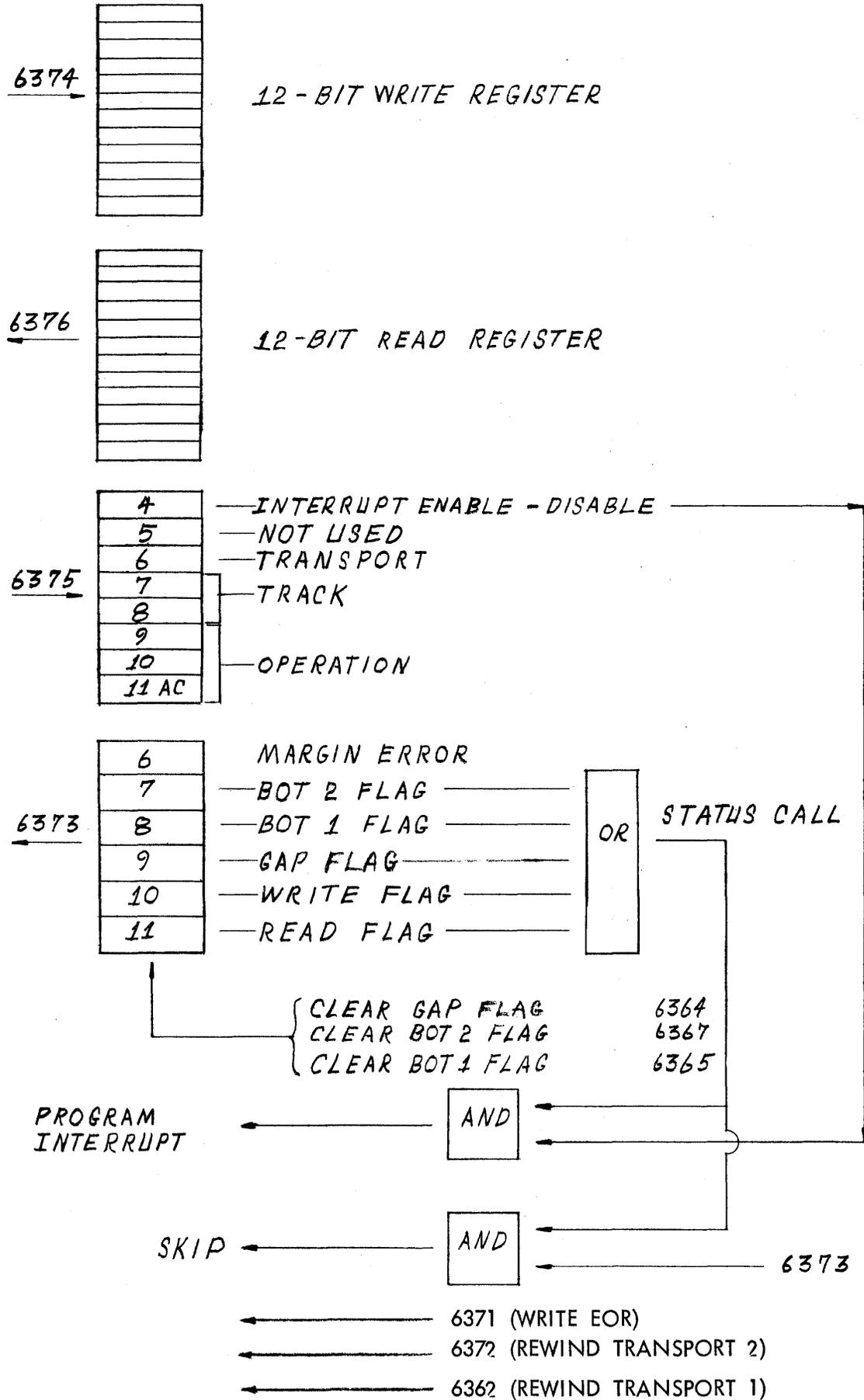
In general with the two-transport TP-1372 option, only one transport may be in operation at any one time. There is one exception: One transport may be rewound using its rewind instruction (page 4.0), while the other transport is being controlled through the command register.
