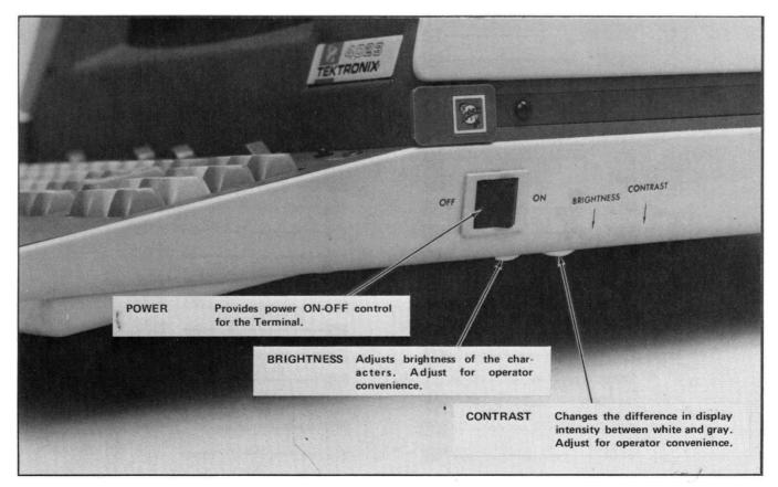
Fig. 1-9. Power and Display controls.
