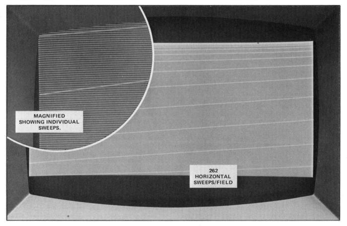
Fig. 6-1. Field definition. A video field contains 262 horizontal sweeps. The Standard Terminal is factory wired to generate 60 fields each second.
