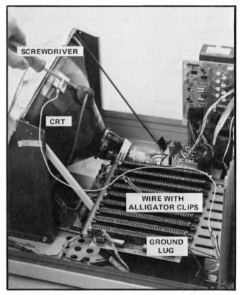
Fig. 3-3. Discharging the high voltage anode.
