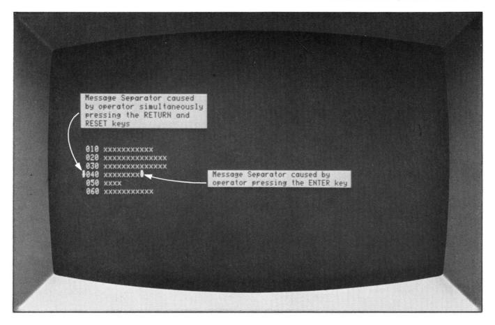
Fig. 1-13. Using Message Separators for selective input.
