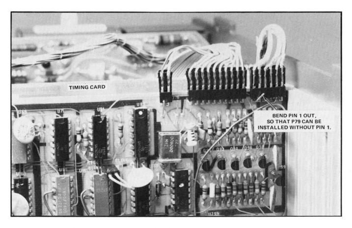
Fig. 4-3. Configuration of P/J79 for Vertical Sync Adjustment.
