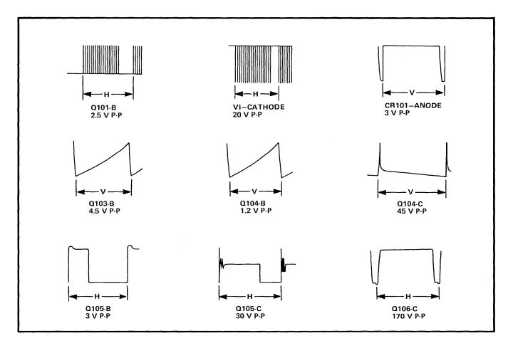
Fig. 6-13. Display waveforms.
