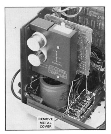
Fig. 1-6. Location of Transformer wiring connectors.
