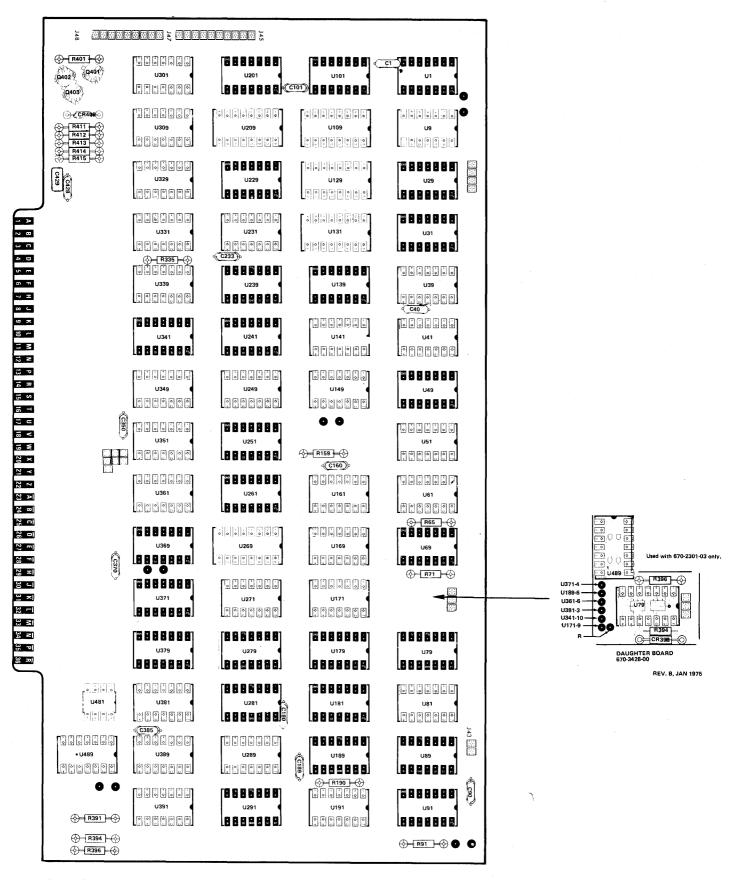
Fig. 6-22. Keyboard interface Card Component Locations 670-2301-04 and below.
