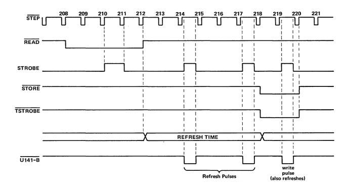
Fig. 6-11. RAM write timing.
