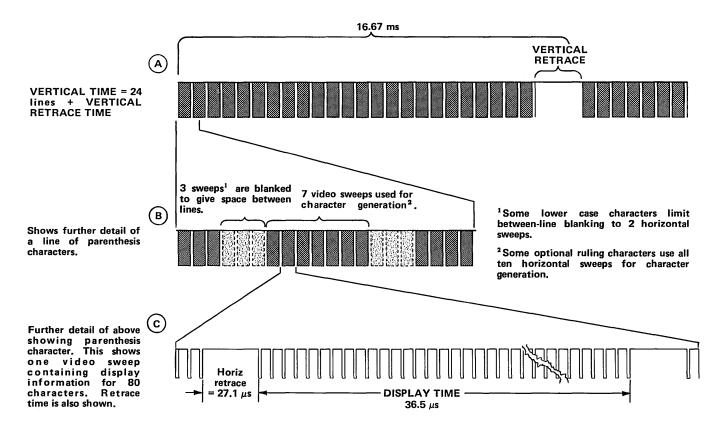
Fig. 6-4. TTL composite video signal.
