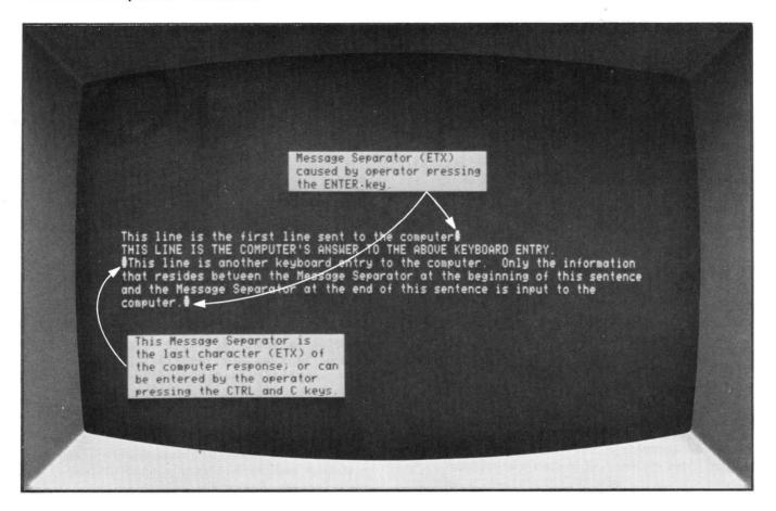
Fig. 1-12. Buffer transmission illustration.
