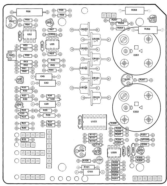
Fig. 6-32. Power Supply Board Component Locations.
