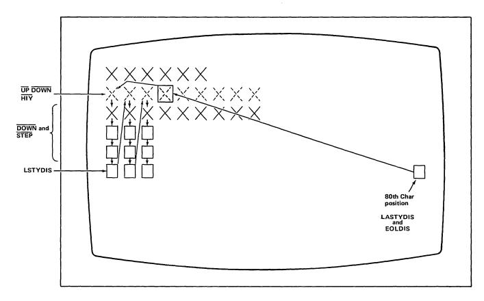
Fig. 6-8. Inserting a line (assume cursor is in 19th line).
