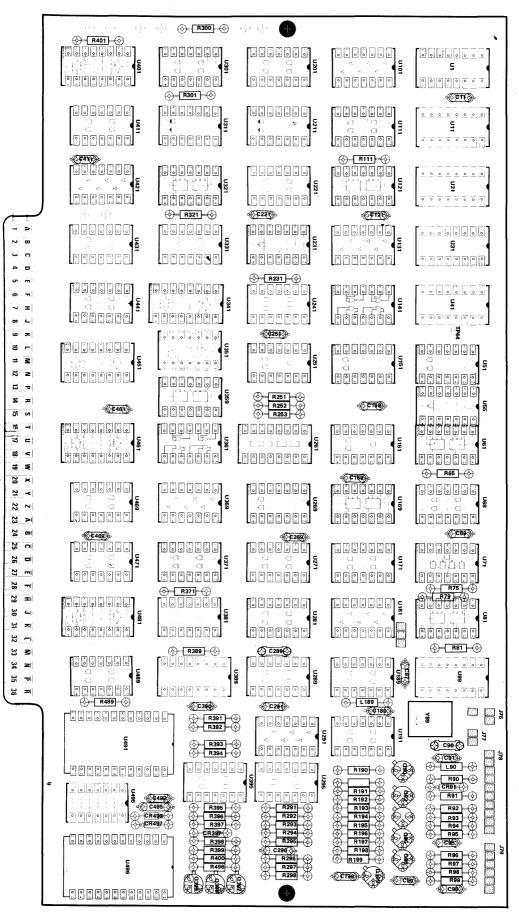
Fig. 6-20C. Timing Card Component Locations (670-2199-04).
