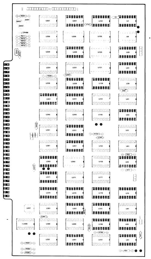
Fig. 6-22. Keyboard interface Card Component Locations 670-2301-04 and below.
