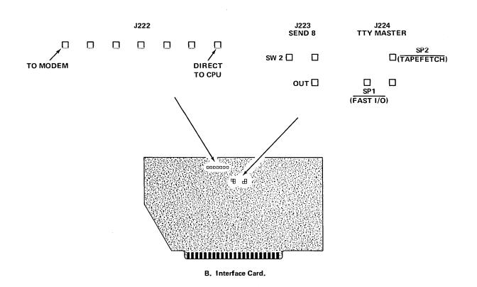
Fig. 1-4A & B. Options on the Timing and Standard Interface card that can be selected by strap placement.
