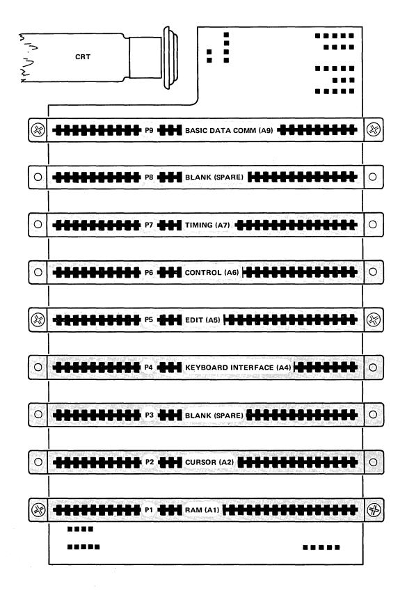
Fig. 1-5. Motherboard (minibus) connector assignments.
