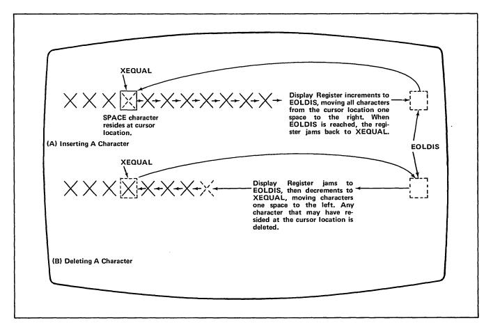
Fig. 6-10. Inserting and Deleting a character.
