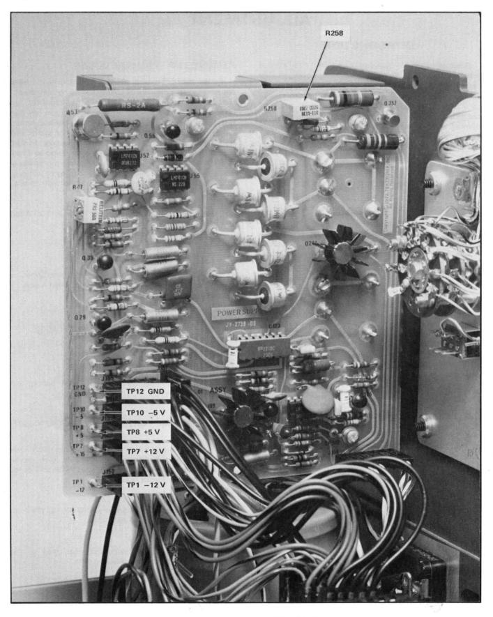
Fig. 4-1. Power Supply Adjustment and Test Point locations.
