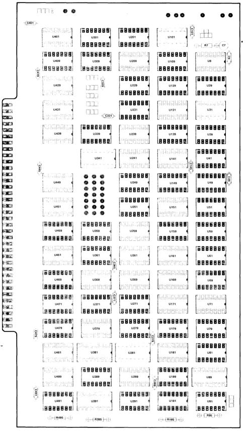
Fig. 6-24. Control Card Component Locations.
