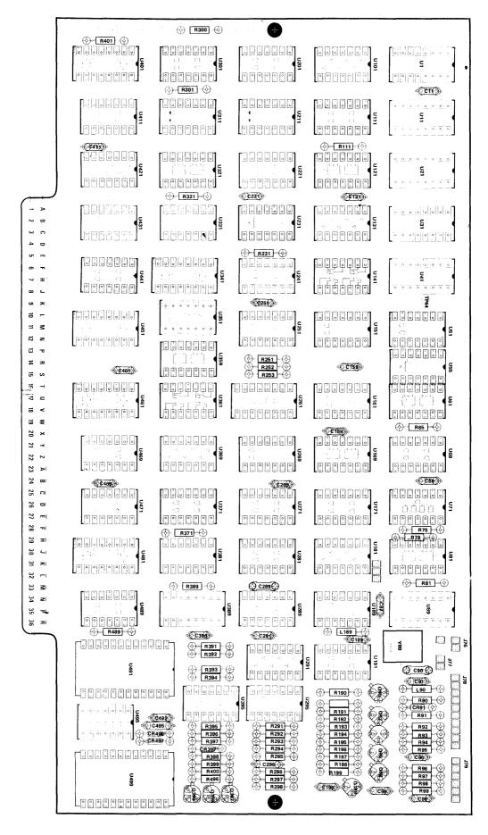
Fig. 6-20D. Timing Card Component Locations (670-2199-05).
