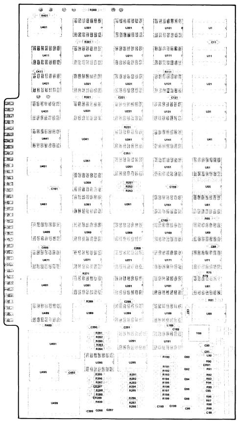
Fig. 6-20B. Timing Card Component Locations (670-2199-03).
