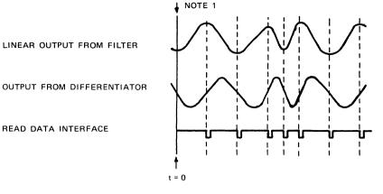
NOTES: t = 0 =250 MILLISECONDS AFTER DRIVE MOTOR STARTS, OR 20 MILLISECONDS AFTER STEP COMMAND, OR 100 u SECONDS AFTER TERMINATION OF WRITE BUSY, (WHICHEVER IS THE LATEST TIME)
