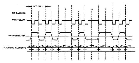
Figure 1-3 FM Recording Magnetization Profiles
