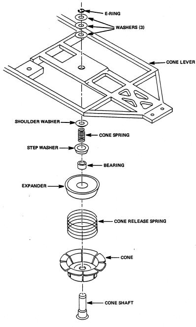
Figure 5-8 Cone's Component Parts
