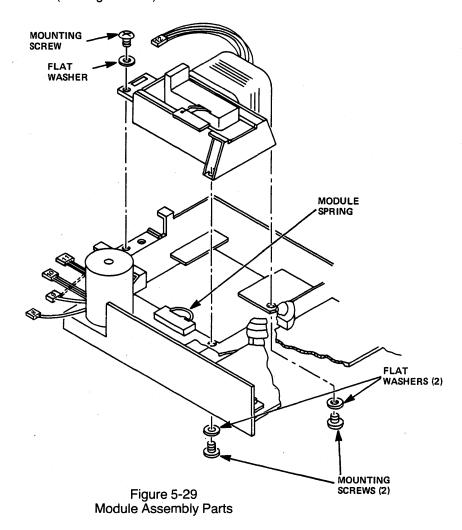
One screw is located on the top middle at the back of the chassis. The other two screws are located underneath the middle of the chassis.
