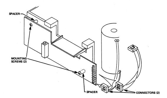
Figure 5-3 Servo PCBA Connectors, Mounting Screws, and Spacers
