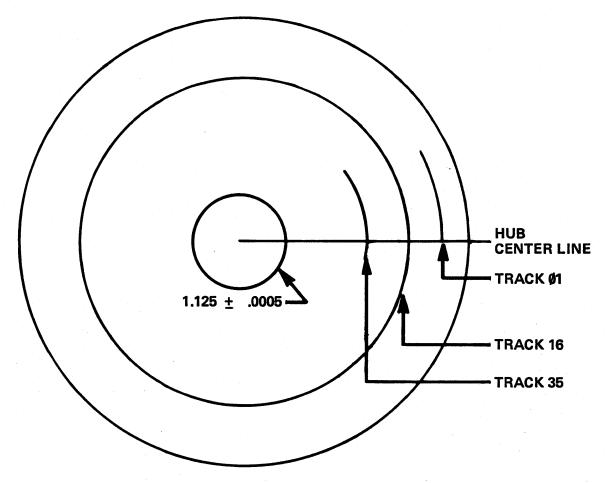
Figure 2-4 Hub Center Line and Track Locations
