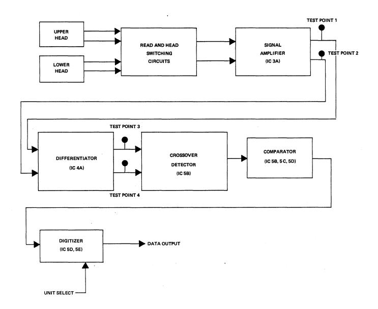
Figure 3-14 Read Circuit Block Diagram
