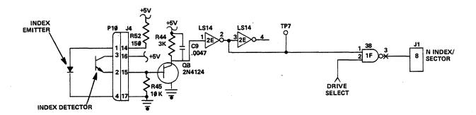
Figure 3-9 Index Schematic Diagram
