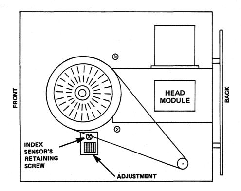
Figure 2-9 Index Sensor's Retaining Screw and Adjustment
