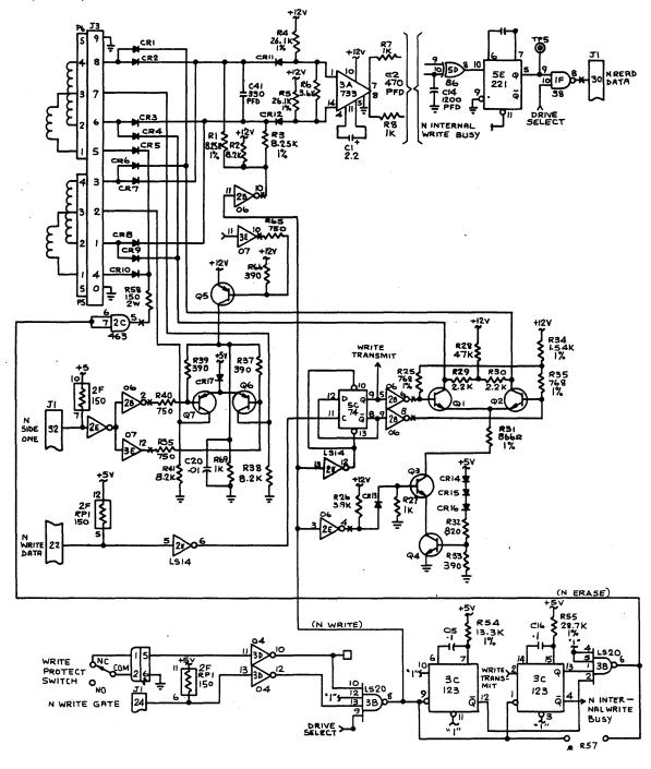
Figure 3-8 Side Select Schematic Diagram
