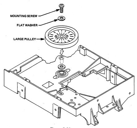
Figure 5-30 Spindle Assembly Mounting Screw, Washer, and Pulley
