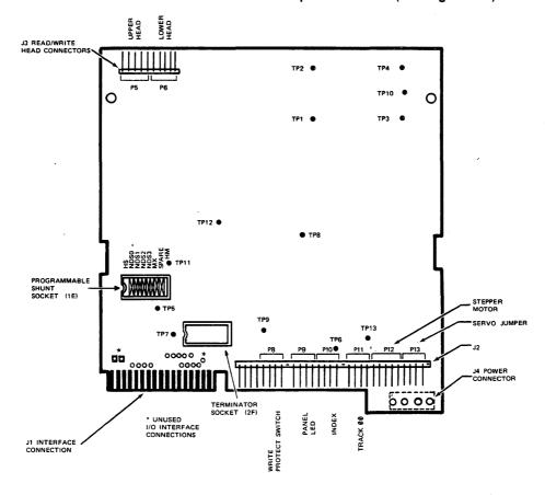
Figure 1-6 Logic Printed Circuit Board Assembly
