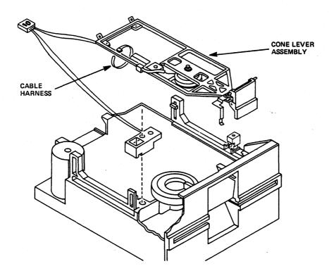
Figure 5-6 Cone Lever Assembly Cable Harness
