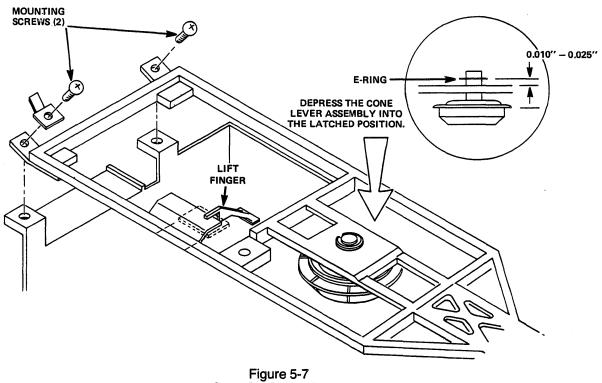
Figure 5-7 Cone Shaft and E-Ring
