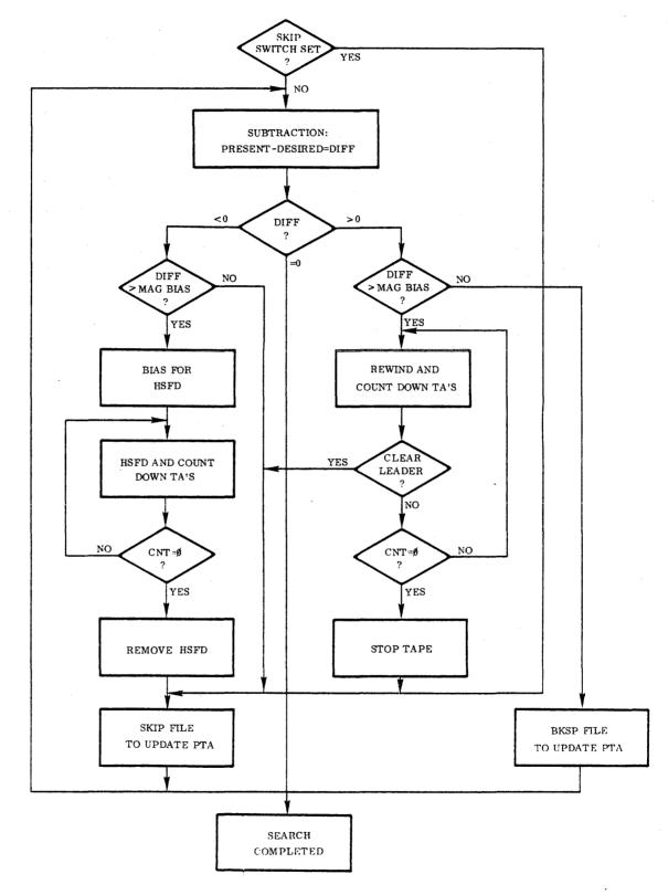
FIGURE 6-3 FLOW CHART, SEARCH FOR DESIRED TAPE ADDRESS
