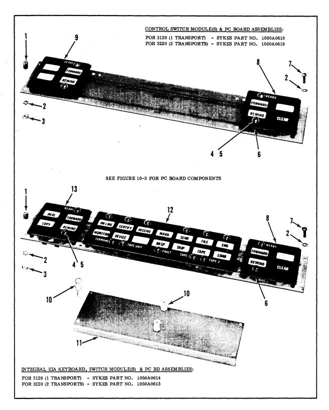
FIGURE 10-1 CONTROL SWITCH AND INTEGRAL KEYBOARD ASSEMBLIES
