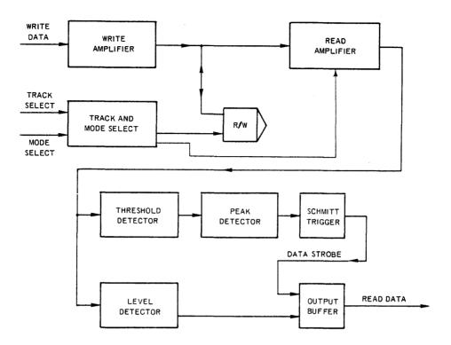
FIGURE 3-4 BLOCK DIAGRAM, READ/WRITE ASSEMBLY
