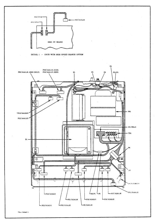
FIGURE 13-2 HARNESS LAYOUT - RACK MOUNTABLE SERIES 3000 UNIT
