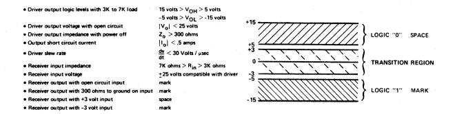
FIGURE 7-2 RS-232-C ELECTRICAL SPECIFICATIONS AND VOLTAGE LEVELS
