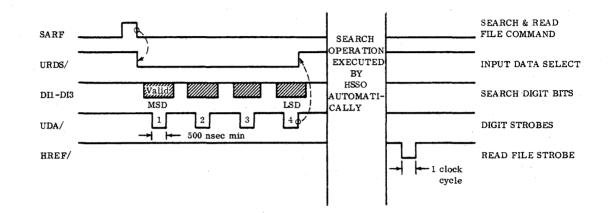
FIGURE 6-7 SEARCH AND READ FILE SIGNAL SEQUENCE TIMING
