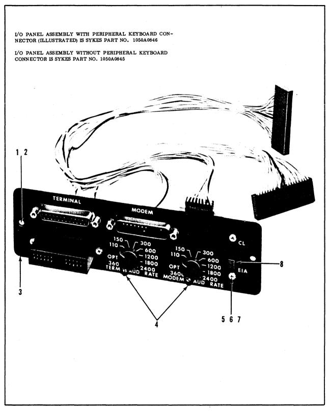
FIGURE 7-4 EIA INTERFACE I/O PANEL ASSEMBLY
