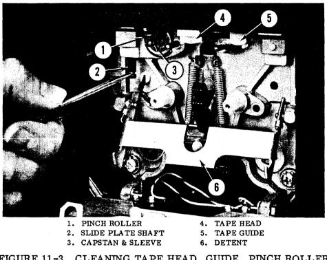
FIGURE 11-3 CLEANING TAPE HEAD, GUIDE, PINCH ROLLER
