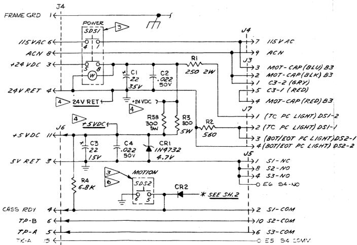
DWG. NO. 1020B40 SHEET 2 of MOTOR CONTROL BOARD 1 SCHEMATIC
