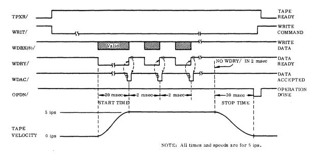
FIGURE 5-8 WRITE DATA TIMING
