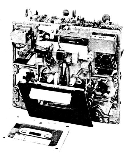
FIGURE 3-1 TAPE TRANSPORT ASSEMBLY, FRONT VIEW
