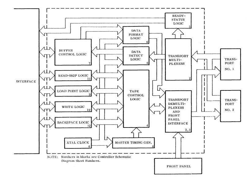
The Series 3000 controller logic performs many functions in the system. The main functions are:
