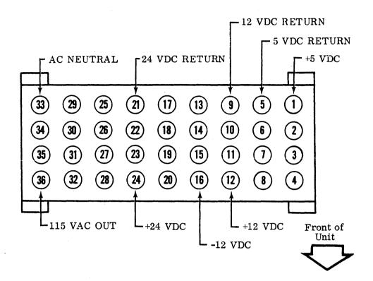
FIGURE 4-1 WIRING SIDE OF CONNECTOR P1 (PS1J1 MATE)
