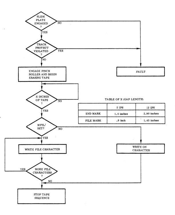
FIGURE 5-5 FLOW CHART, WRITE FILE OR END MARK SEQUENCE
