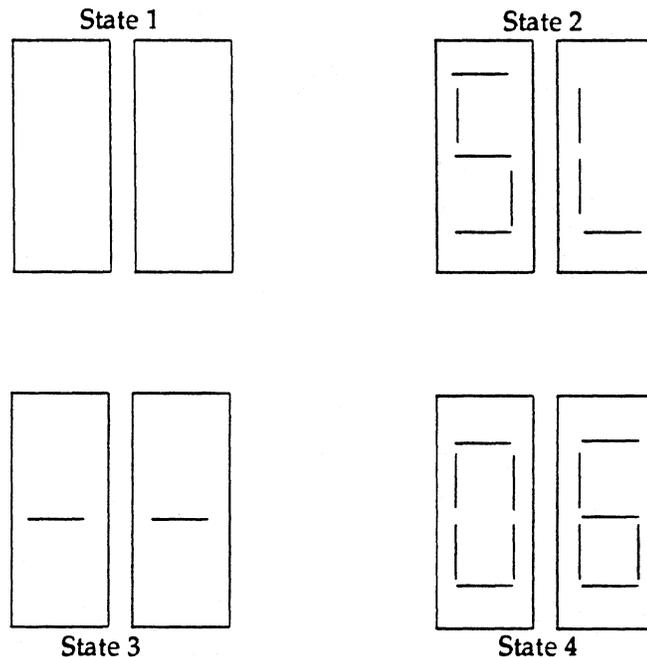
Figure 1-5. Normal Multiprocessor Slave States
