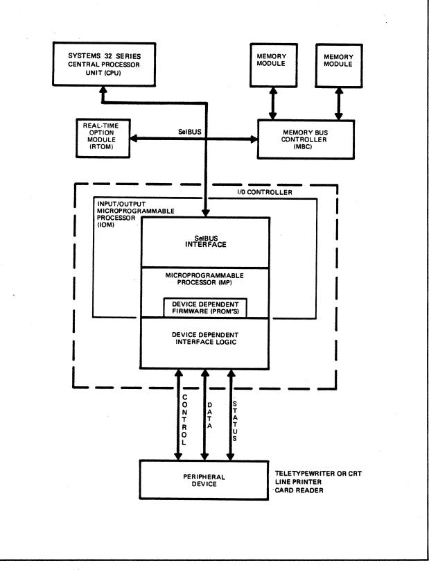
Figure 3-1. Block Diagram - SYSTEMS 32 SERIES Computer
