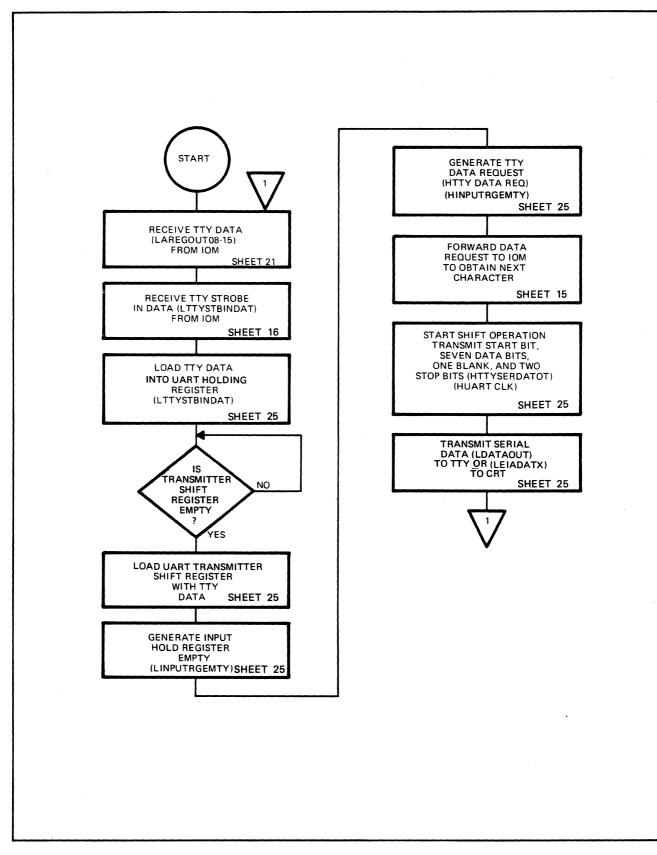
Figure 3-13. Output Data Transfer (TTY)
