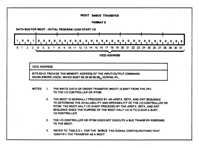
Figure 3-2. Write Data or Order Transfer (WDOT) Format (Sheet 3 of 3)
