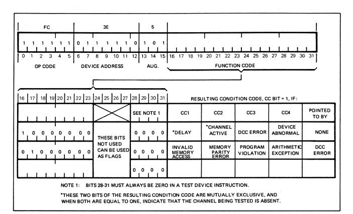
Figure 2-9. Test Device Format and Function Code TTY System
