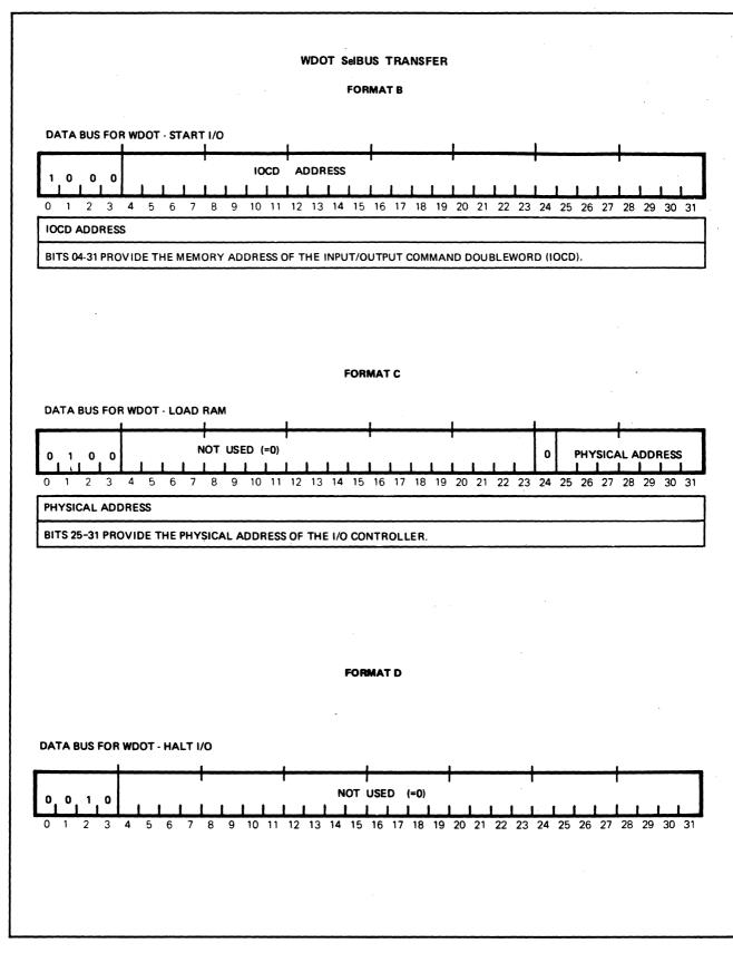
Figure 3-2. Write Data or Order Transfer (WDOT) Format (Sheet 2 of 3)
