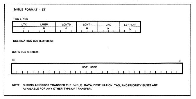
Figure 3-6. Error Transfer (ET) Format
