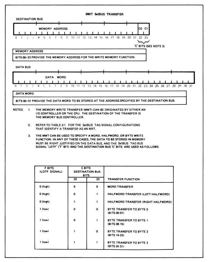
Figure 3-7. Memory Write Transfer (MWT) Format
