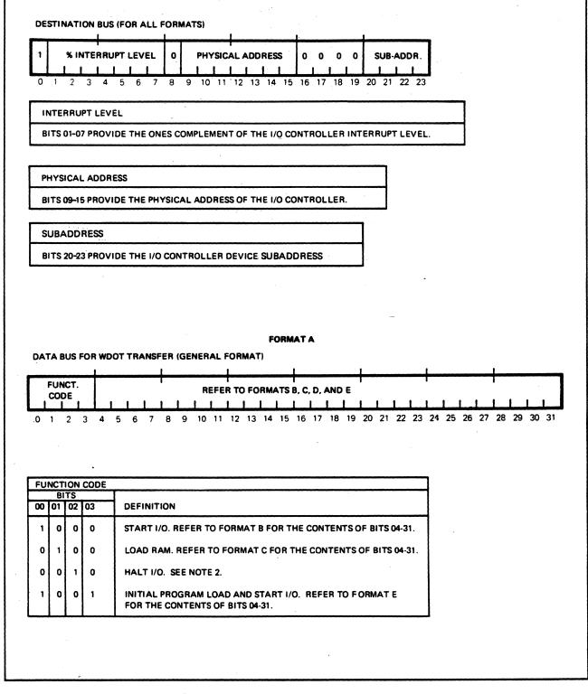
Figure 3-2. Write Data or Order Transfer (WDOT) Format (Sheet 1 of 3)
