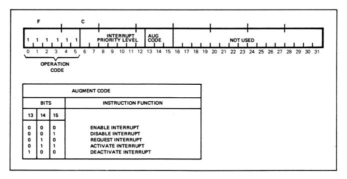
Figure 2-6. Interrupt Control Instruction Format
