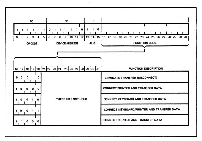
Figure 2-8. Command Device Format TTY System
