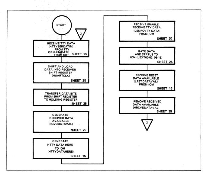
Figure 3-14. Input Data Transfer (TTY)
