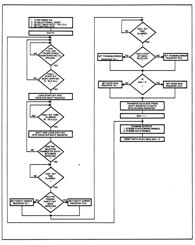
Figure 3-12. UART - Receiver Flow Diagram
