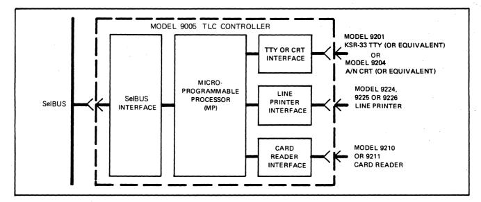
Figure 1-2. Block Diagram - TLC Controller
