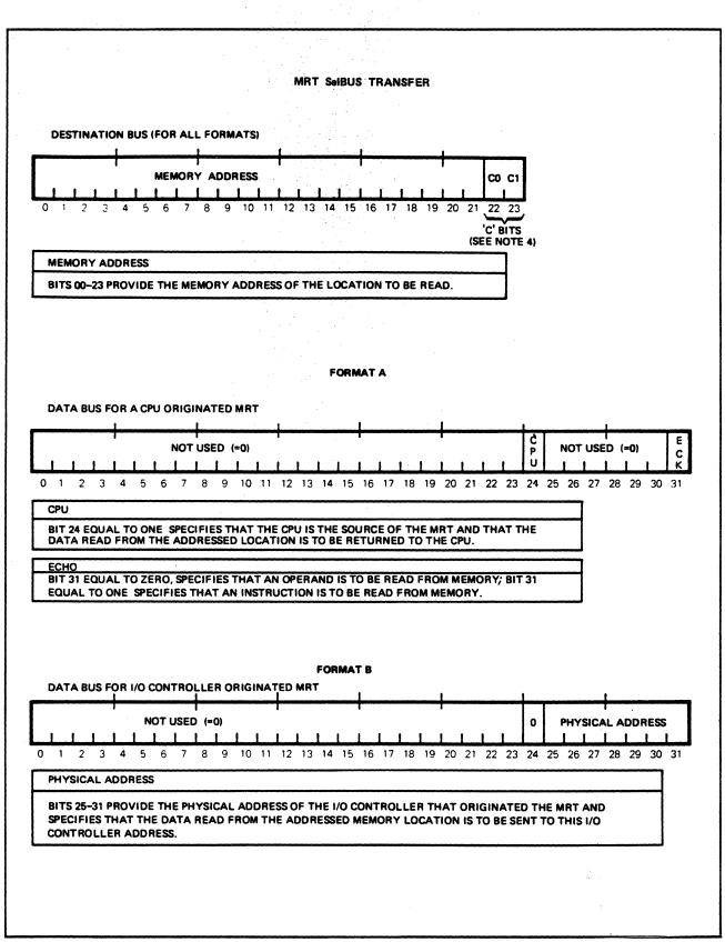
Figure 3-8. Memory Read Transfer (MRT) Format (Sheet 1 of 2)
