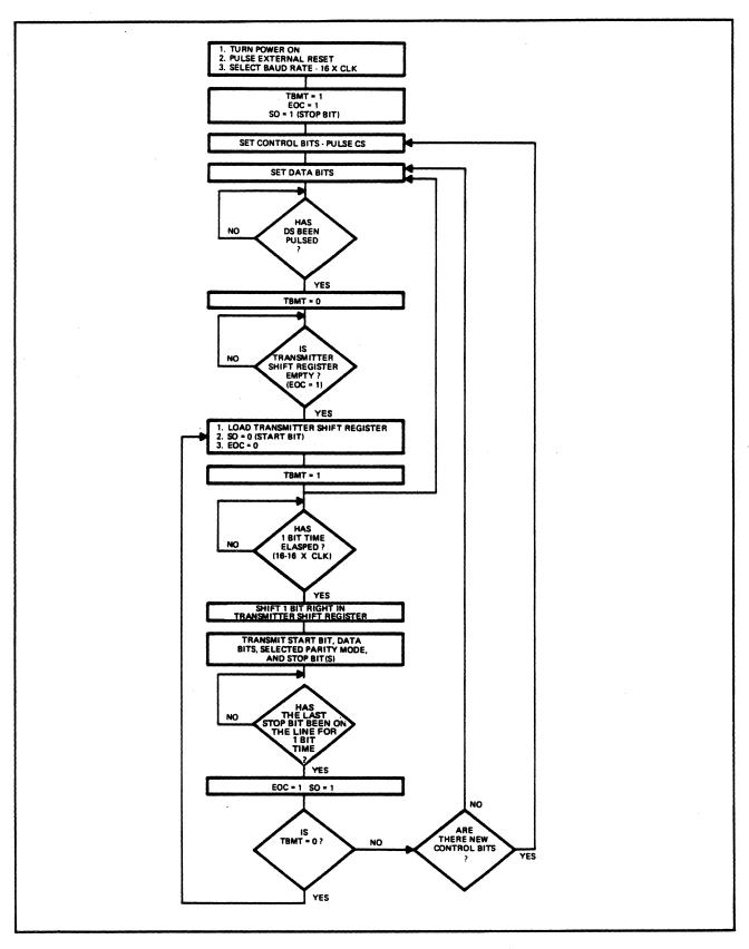
Figure 3-11. UART - Transmitter Flow Diagram
