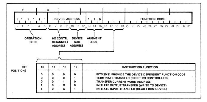
Figure 2-1. Command Device (CD) Instruction Format
