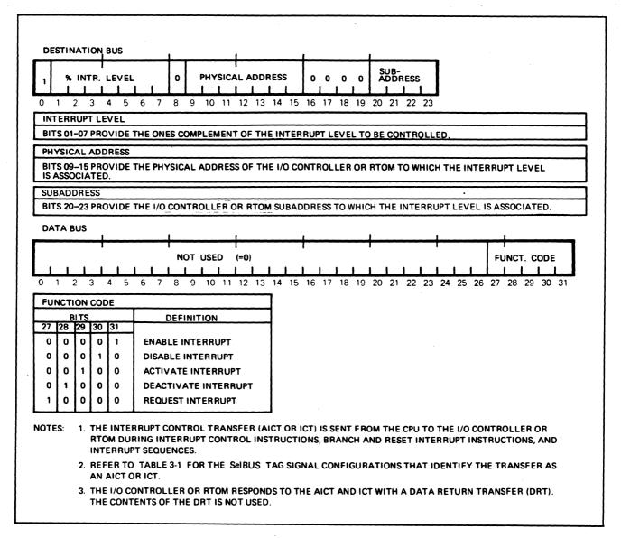
Figure 3-3. Advance Interrupt Control Transfer (AICT) and Interrupt Control Transfer (ICT) Formats
