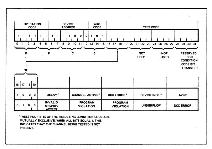
Figure 2-13. Card Reader Test Device Instruction Format
