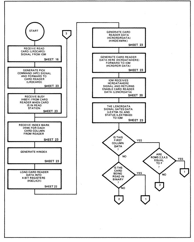
Figure 3-20. Card Reader Operation (Sheet 1 of 2)
