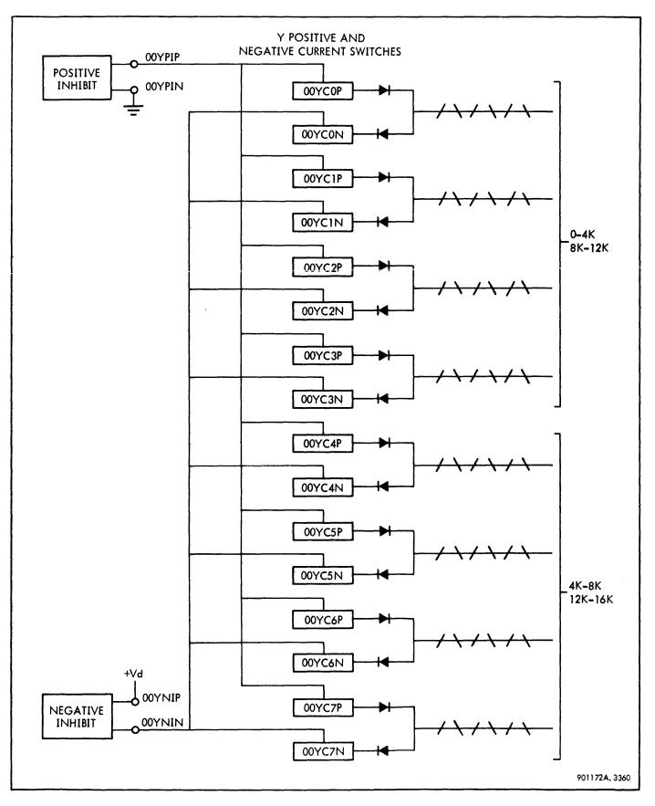
Figure 3-118. Positive and Negative Y Current Inhibit, Bit 0
