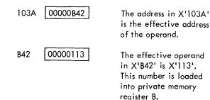
The reference address (X'103A') of the instruction is indirectly addressed (bit 0 = 1); therefore, the contents of this location (X'103A') contain the actual address (X'B42') of the operand or effective word. The operand finally loaded into register B is X'113'.
