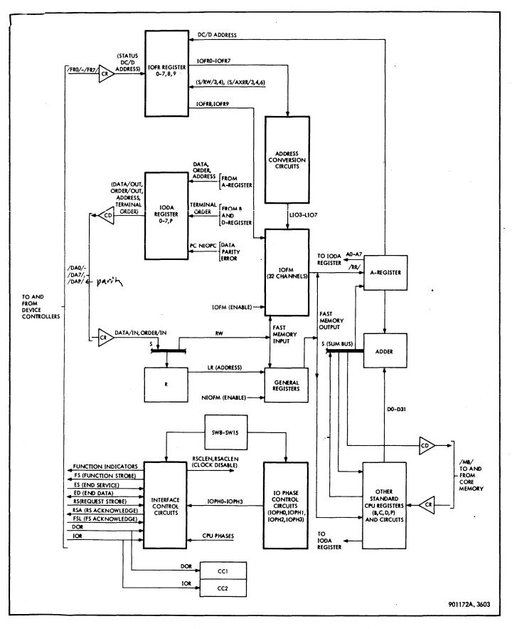
Figure 3-229. Integral IOP, Functional Block Diagram
