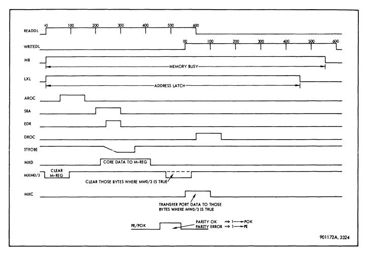
Figure 3-82. Partial Write Timing Diagram
