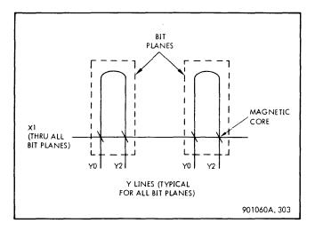
Figure 3-8. Typical X and Y Core Wiring
