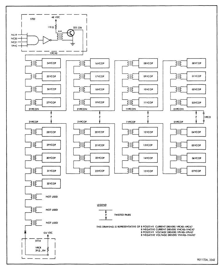
Figure 3-100. Y Positive Current Predrive/Drive Coupling, Simplified Schematic
