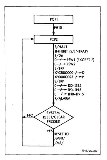
Figure 3–221. CPU RESET/CLEAR and SYSTEM RESET/ CLEAR, Flow Diagram
