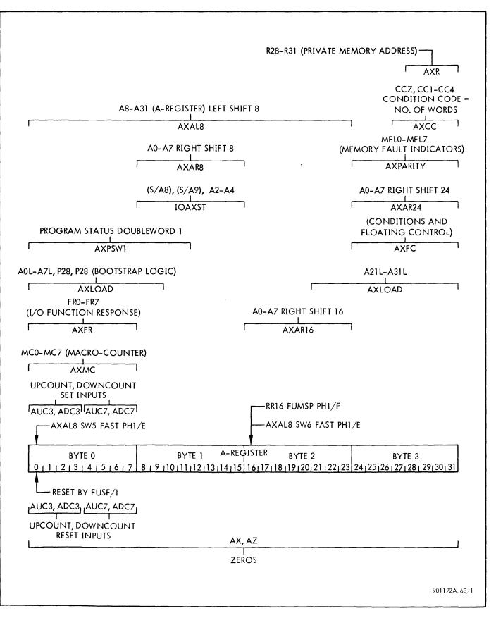
Figure 3-17. A-Register Inputs and Enabling Signals (Sheet 1 of 2)
