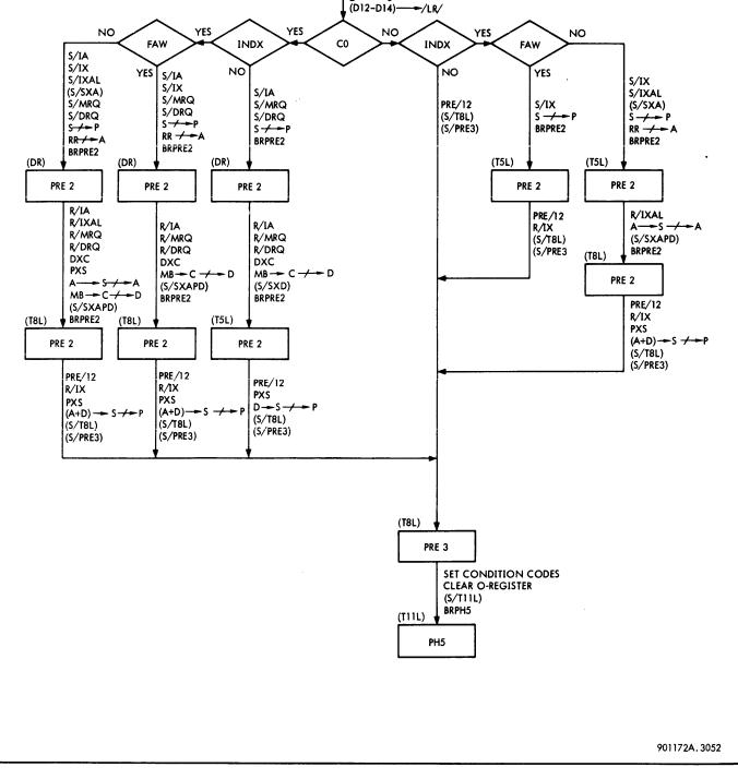
Figure 3-140. Analyze Instruction, Preparation Phases Flow Diagram
