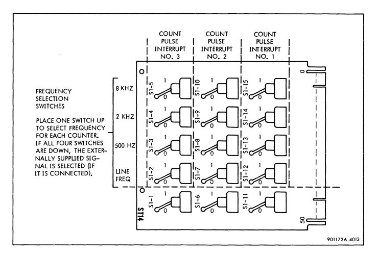
Figure 4-1. Address Selector Module ST14
