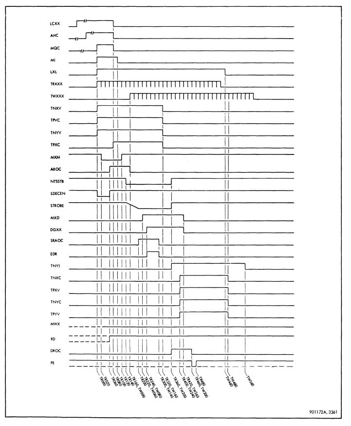
Figure 3-119. Read-Restore, Timing Diagram
