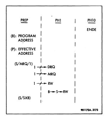
Figure 3-180. BAL Instruction, Phase Sequence Diagram
