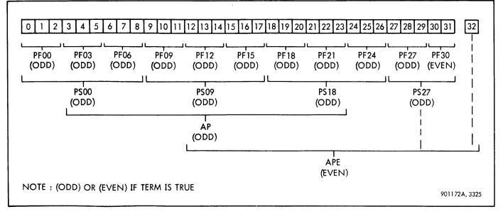
Figure 3-83. Parity Determination Logic Scheme
