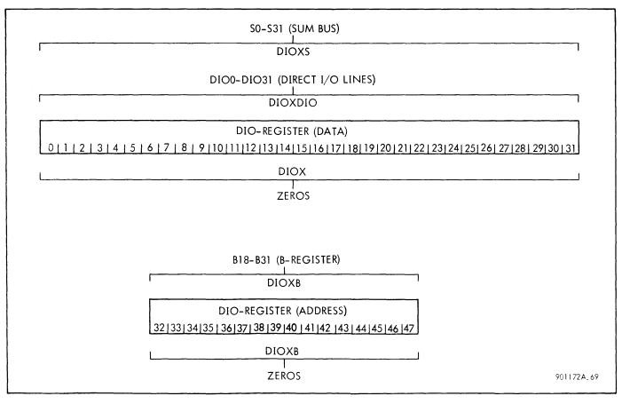
Figure 3-23. DIO-Register Inputs and Enabling Signals
