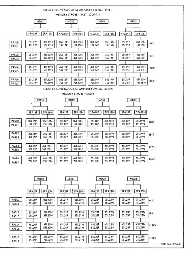
Figure 3-113. Sense Line/Preamp/Sense Amplifier System (Bytes 1 and 2) (Sheet 2 of 3)
