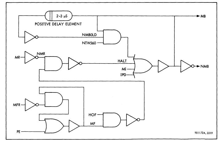
Figure 3-77. Memory Busy (MB), Logic Diagram
