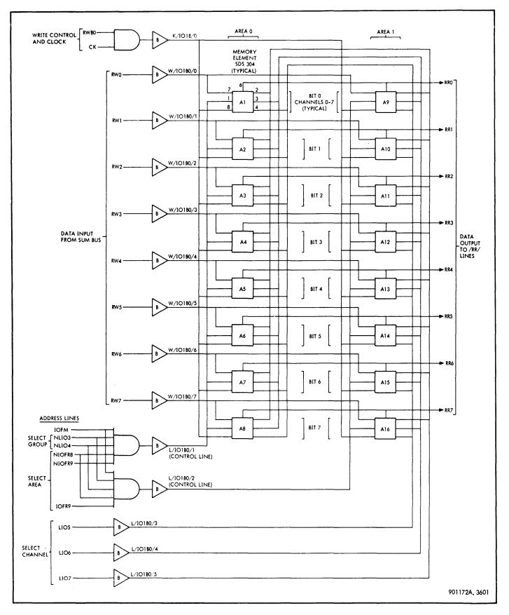
Figure 3-232. Fast Memory Module FT25, Logic Diagram
