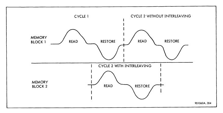
Figure 3-9. Example of Interleaving in Read-Restore Mode
