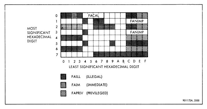
Figure 3-52. Operation Codes Resulting in Trap
