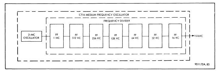
Figure 3-44. Oscillator Clock Generator, Block Diagram
