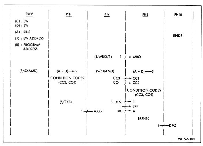
Figure 3–156. Compare With Limits in Register, Phase Diagram
