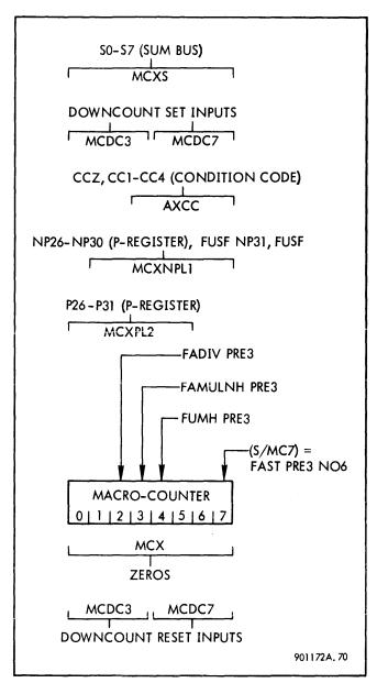
Figure 3-24. Macro-Counter Inputs and Enabling Signals
