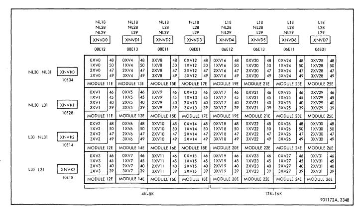
Figure 3-106. X Negative Voltage Predrive Matrix
