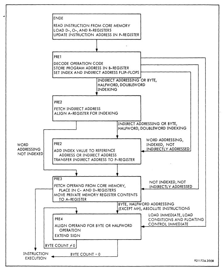
Figure 3-123. Preparation Phases General Functions, Block Diagram
