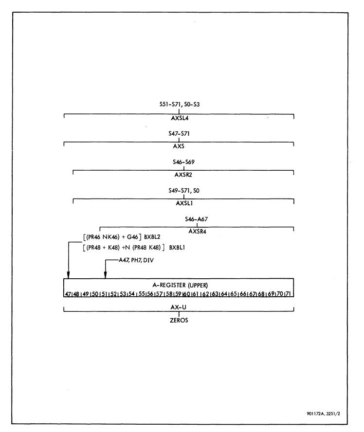
Figure 3-211. Floating Point A-Register Inputs and Enabling Signals (Sheet 2 of 2)
