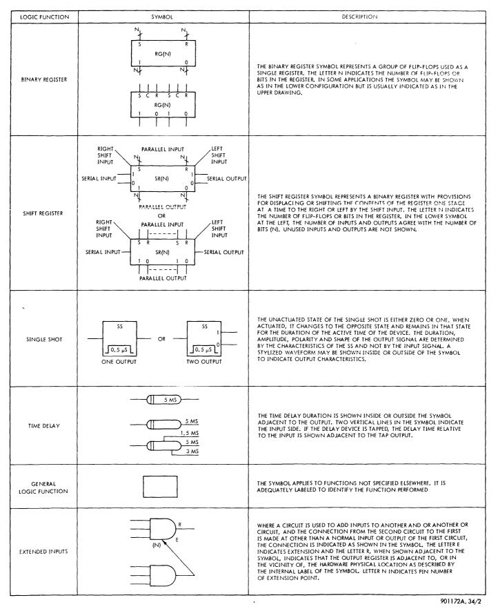
Figure 3-13. Basic Logic Symbols Chart (Sheet 2 of 3)
