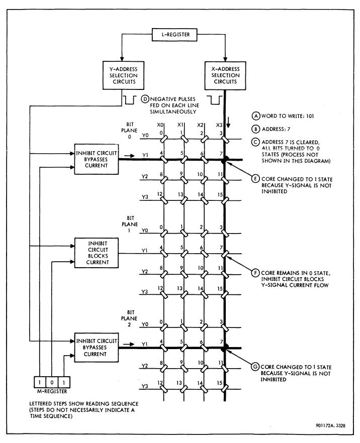
Figure 3-86. Simplified Memory, Clear Write Operation
