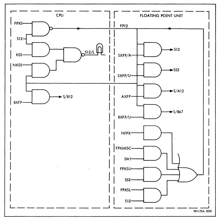
Figure 3-218. Floating Point Bit 12, Logic Diagram
