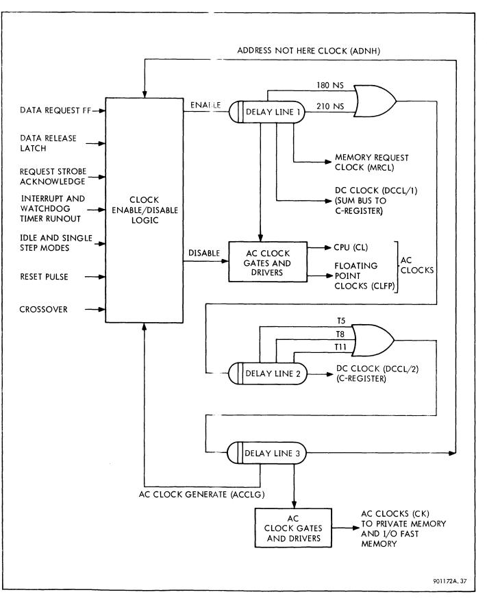
Figure 3-4. CPU Clock Generator, Simplified Block Diagram
