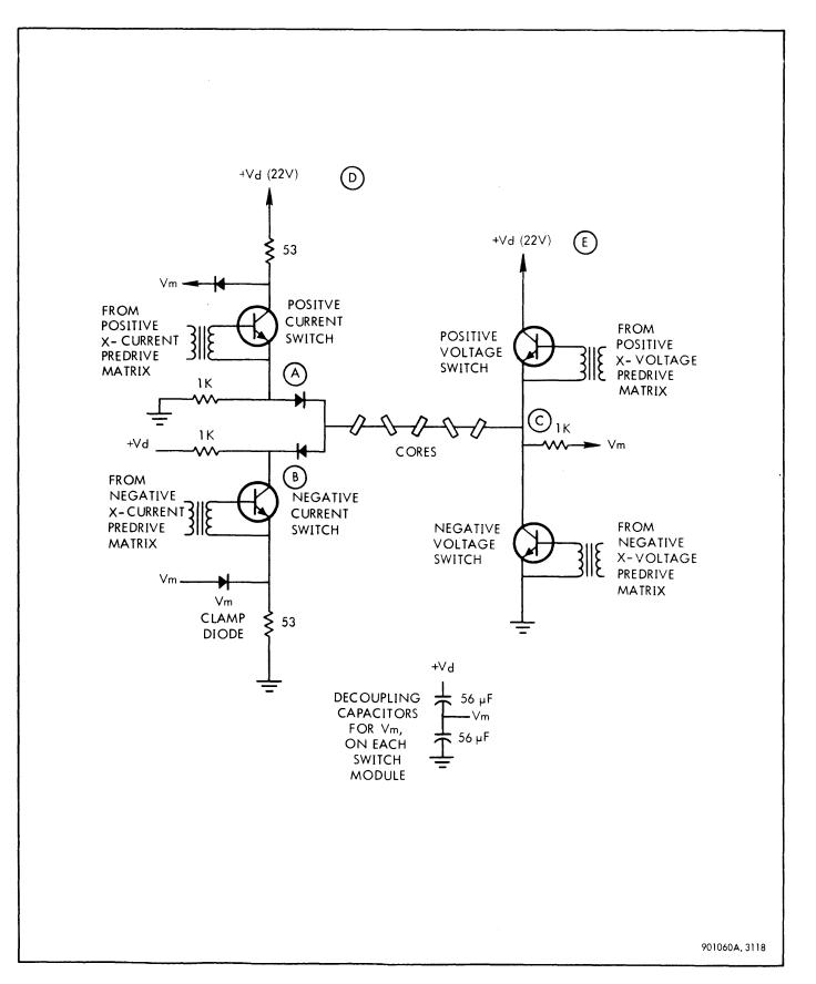
Figure 3-95. Memory Core Drive System, Simplified Schematic
