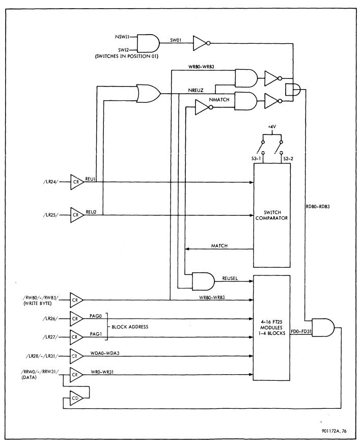
Figure 3-34. Register Extension Chassis, Simplified Logic Diagram
