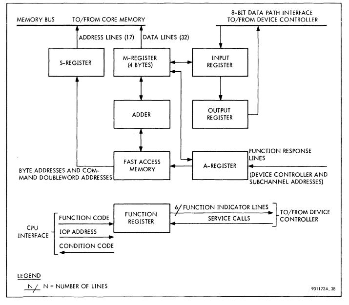
Figure 3-10. Multiplexing IOP, Simplified Block Diagram
