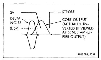
Figure 3-115. Sense Waveforms
