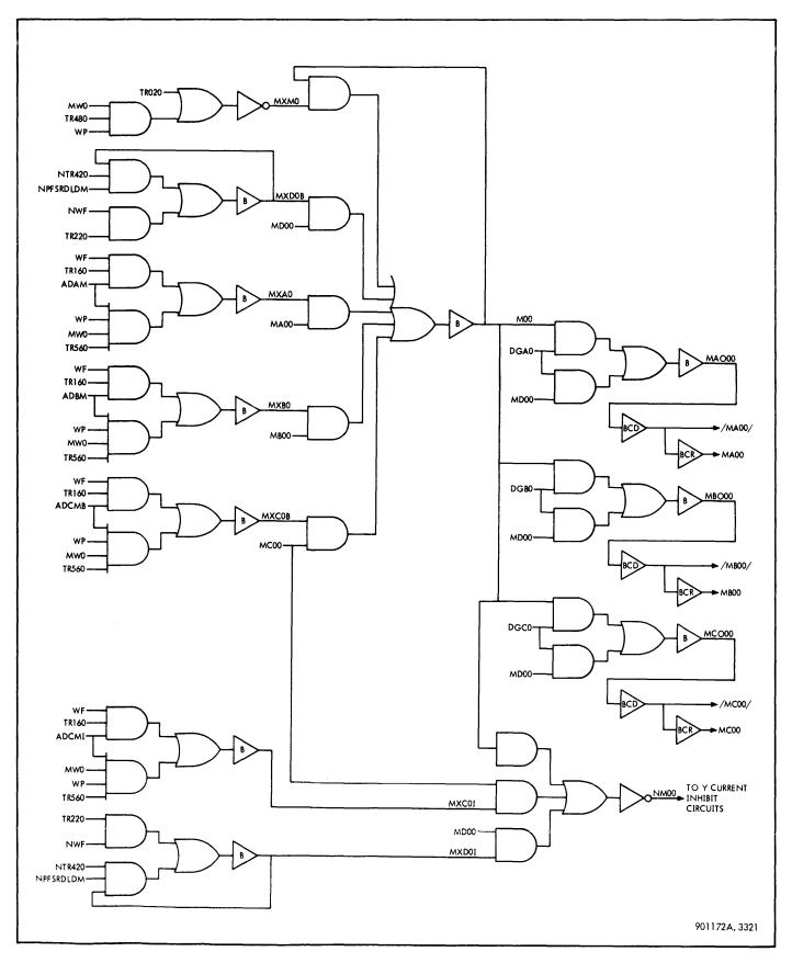
Figure 3-79. M-Register (M00, Typical of M00-M31)
