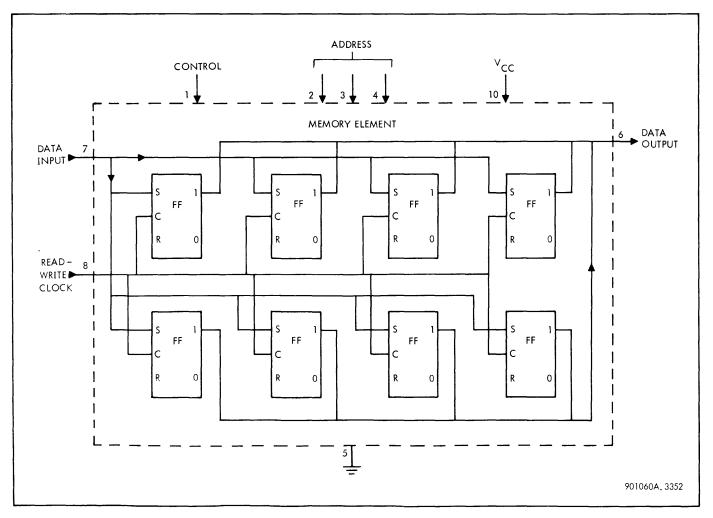
Figure 3-30. SDS 304 Memory Element, Simplified Diagram
