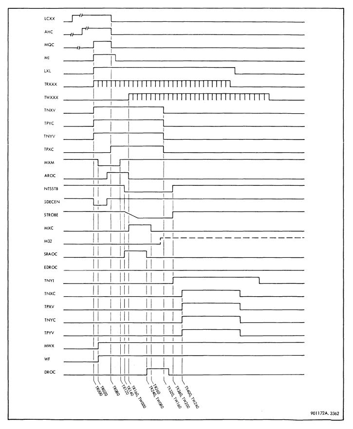
Figure 3-120. Full Clear Write, Timing Diagram
