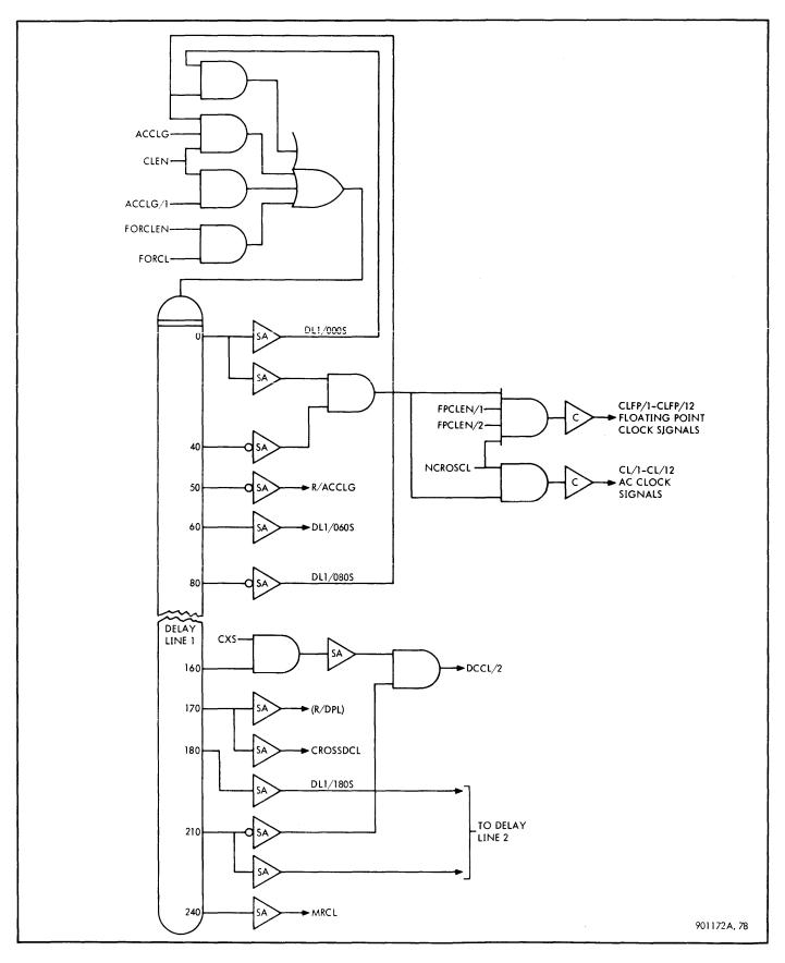
Figure 3-37. Delay Line 1, Logic Diagram
