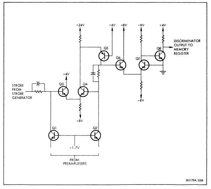
Figure 3-116. Sense Amplifier, Simplified Schematic
