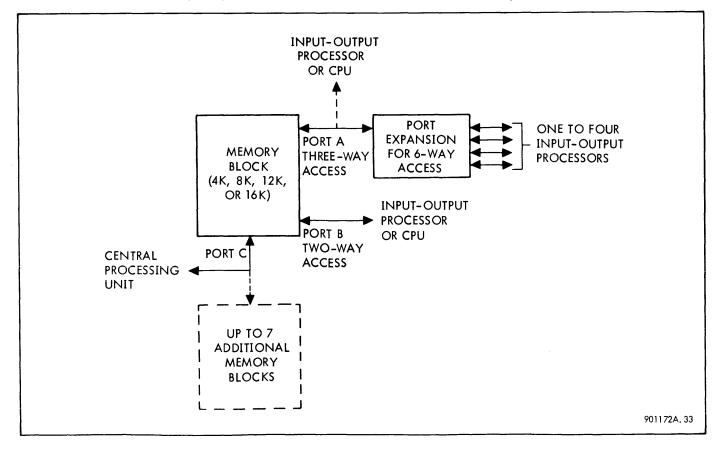
Figure 3-7. Memory Connections and Port Expansion
