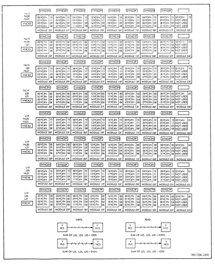
Figure 3-108. Y Negative Current Predrive/Drive Coupling System
