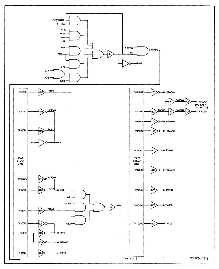
Figure 3-72. Read and Write Delay Lines
