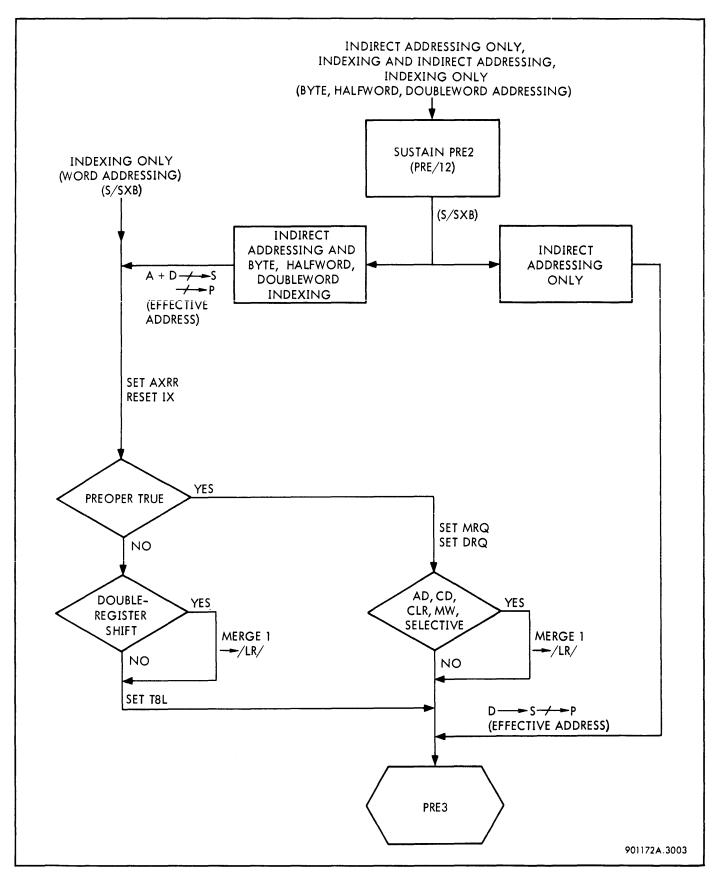
Figure 3-127. Preparation Phase PRE2 (PRE/12 Time), Flow Diagram
