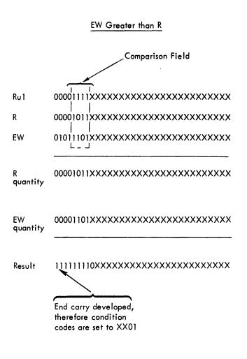
Compare Selective Phase Sequence. Preparation phases for the CS instruction are the same as the general PREP phases for word instructions, paragraph 3–59. Figure 3–138 shows the simplified phase sequence for the CS instruction, and table 3–42 lists the detailed logic sequence during all execution phases of the instruction.
