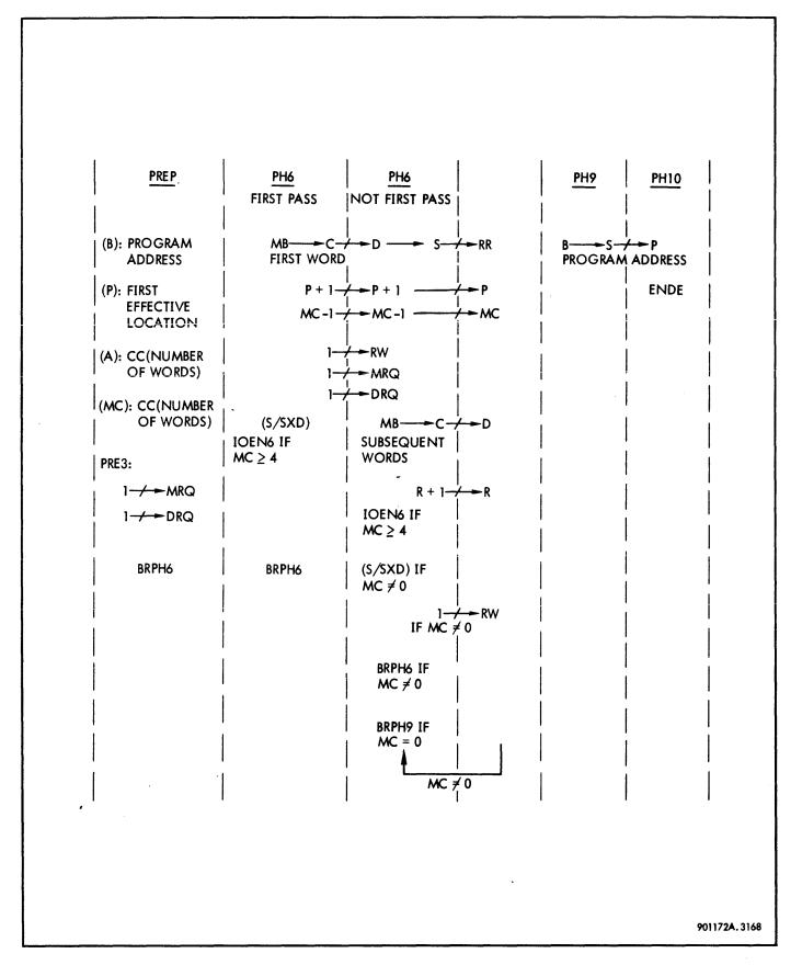
Figure 3-176. Load Multiple Instruction, Phase Sequence Diagram
