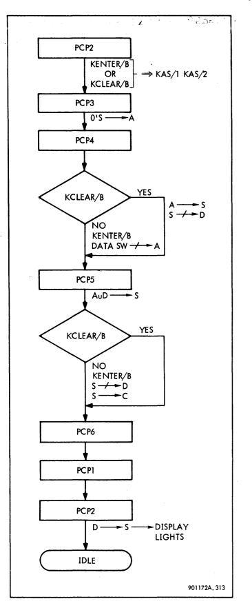
Figure 3-223. DATA ENTER/DATA CLEAR, Flow Diagram
