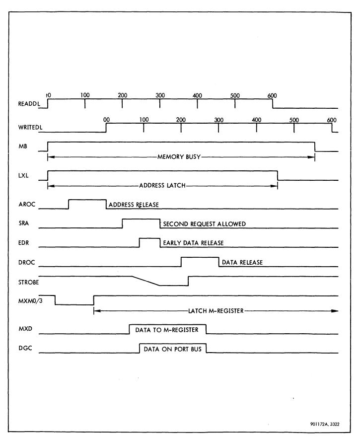
Figure 3-80. Read Timing Diagram
