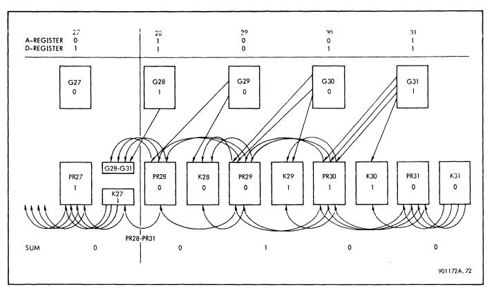
Figure 3-26. A Plus D Adder Logic
