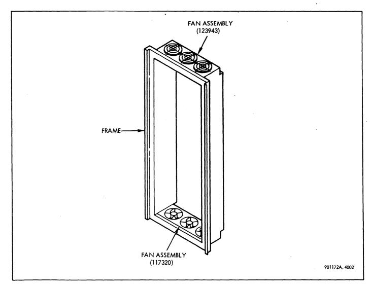
Figure 4-4. Frame Assembly With Fan Arrangement
