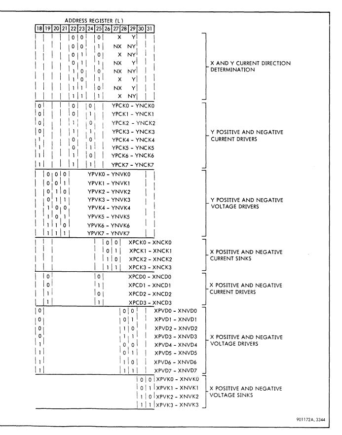
Figure 3-102. X and Y Predrive Selection Relative to Memory Address
