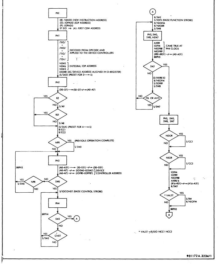
Figure 3-197. SIO, HIO, TIO, TDV Flow Diagram for Integral IOP (Sheet 1 of 2)
