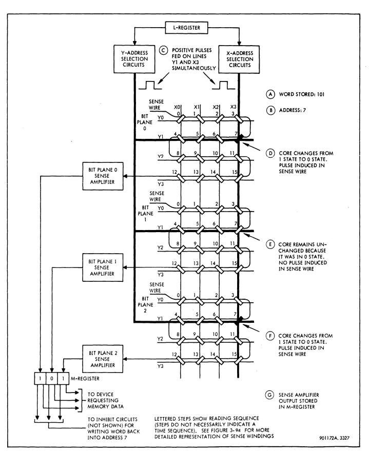
Figure 3-85. Simplified Memory, Read-Restore Operation
