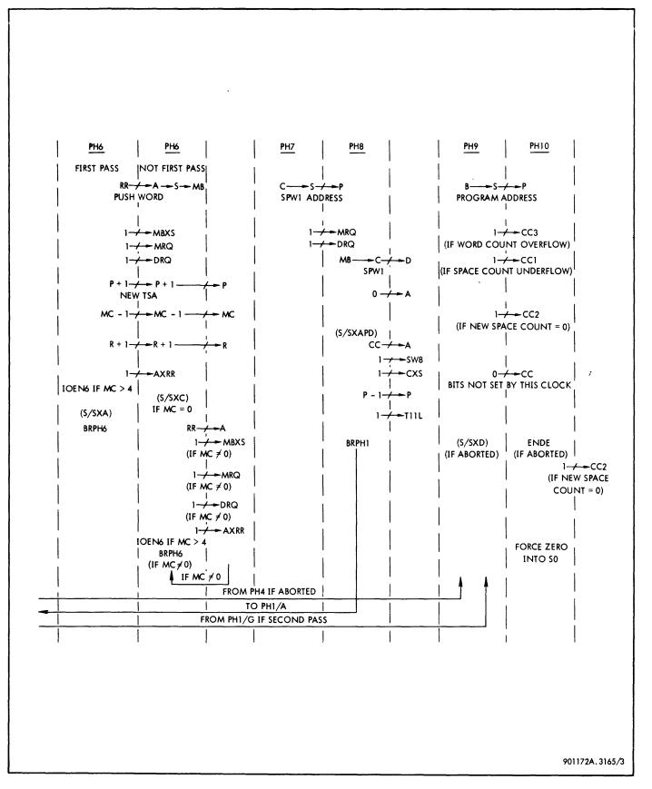
Figure 3-173. Push Multiple Instruction, Phase Sequence Diagram (Sheet 3 of 3)
