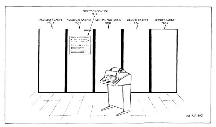
Figure 1-1. Sigma 5 Computer (Typical Configuration)
