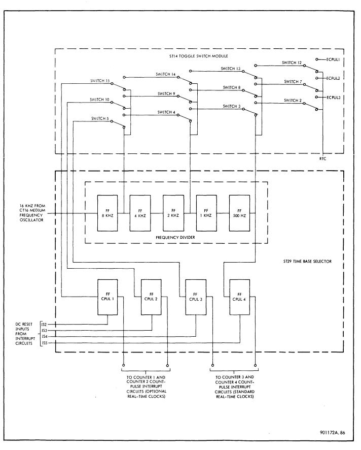
Figure 3-45. Real-Time Clock, Simplified Diagram
