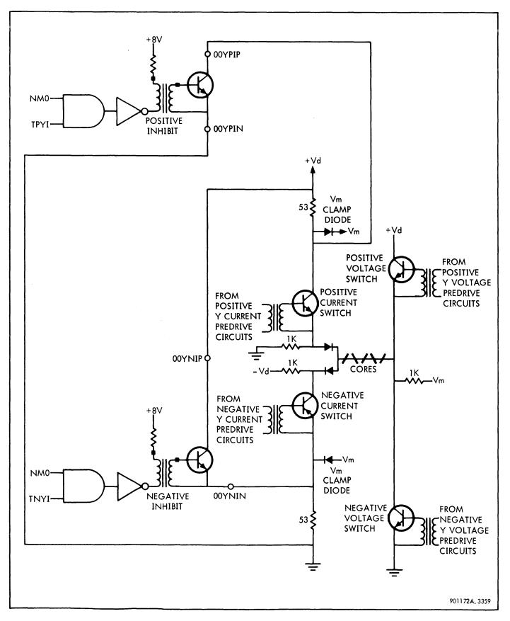
Figure 3-117. Y Current Inhibit Circuits, Simplified Diagram
