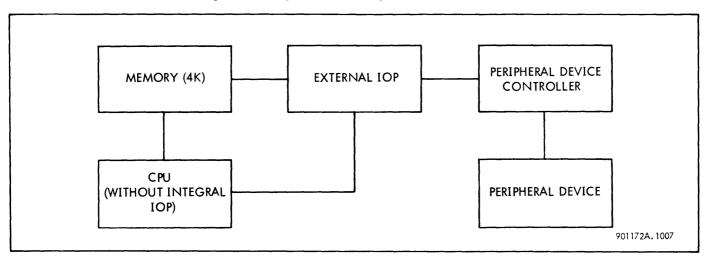
Figure 1-7. Sigma 5 Minimum System Without Integral IOP
