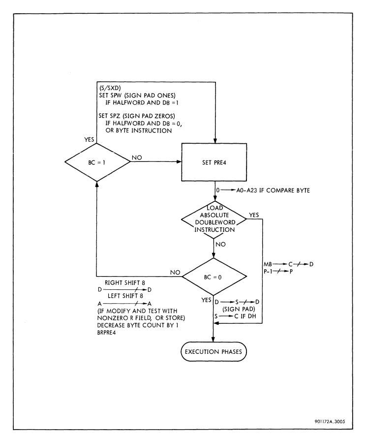
Figure 3-129. Preparation Phase PRE4, Flow Diagram
