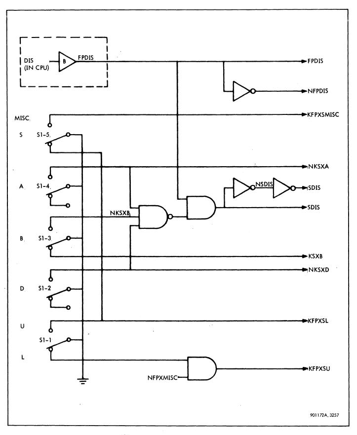
Figure 3-217. Floating Point Display Switches, Logic Diagram
