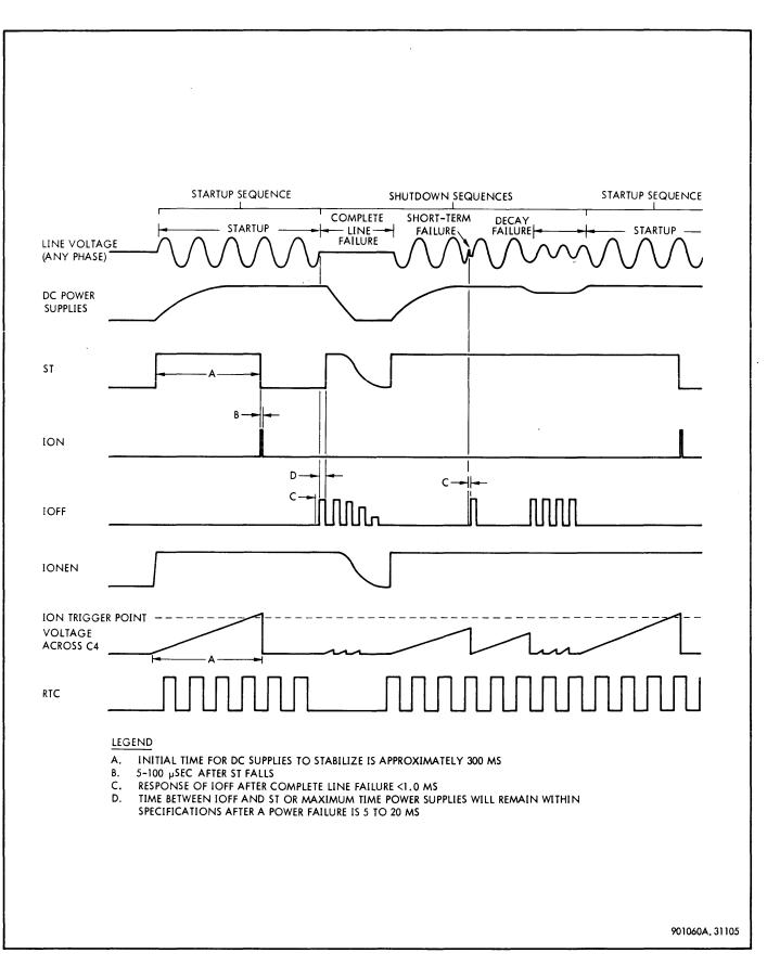
Figure 3-205. Power Fail-Safe Waveforms
