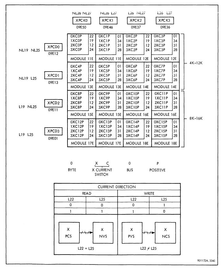
Figure 3-103. X Positive Current Predrive Matrix
