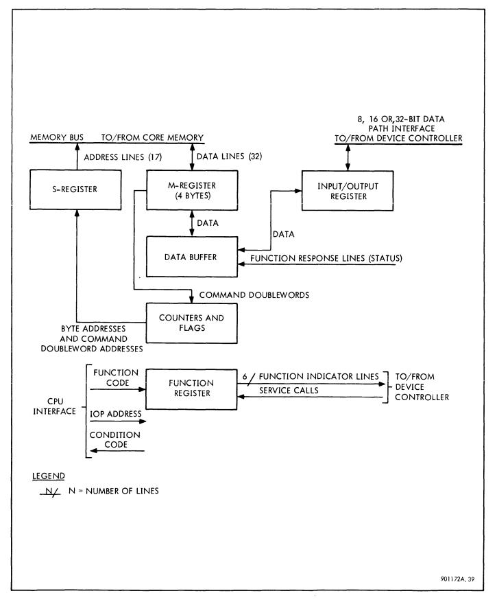
Figure 3-11. Selector IOP, Simplified Block Diagram
