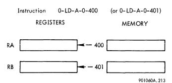
Where even doubleword addresses are specified, the data transfer is from memory even word to register even word, and memory odd word to register odd word.
