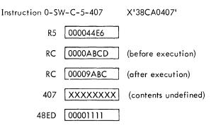
In this example memory location X'407' is not actually addressed and its contents are not affected in any way. The contents of register R5 added to the virtual address of the instruction result in an effective address of X'48ED'. The contents of memory location X'48ED' are subtracted from the contents of register RC and the difference is stored in register RC.
