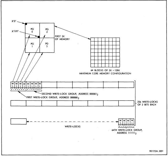
Figure 3-187. Write-Lock Configuration
