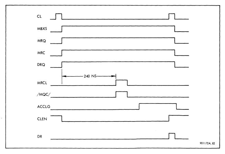
Figure 3-41. Store Operation Timing Diagram
