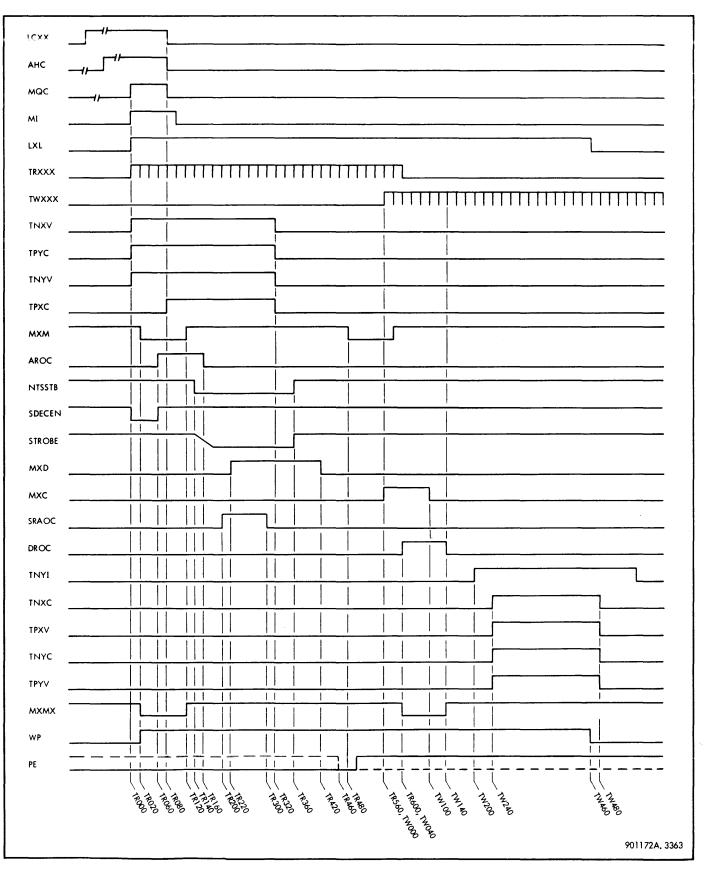
Figure 3-121. Partial Write, Timing Diagram
