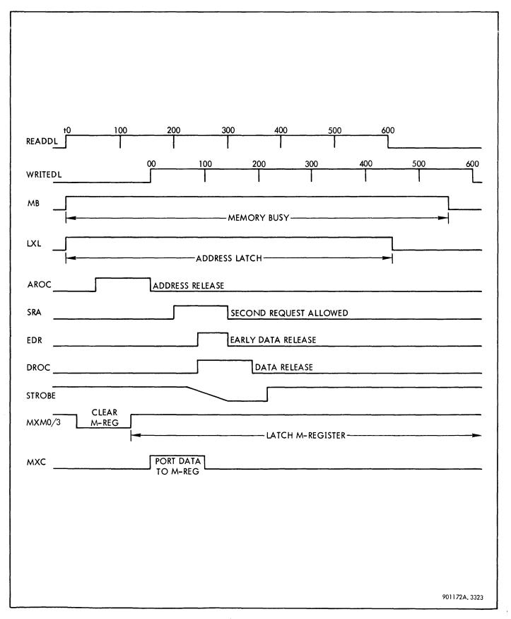
Figure 3-81. Full Write Timing Diagram
