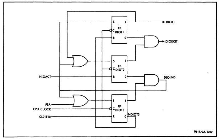
Figure 3-192. DIO Timing Flip-Flops, Simplified Logic Diagram
