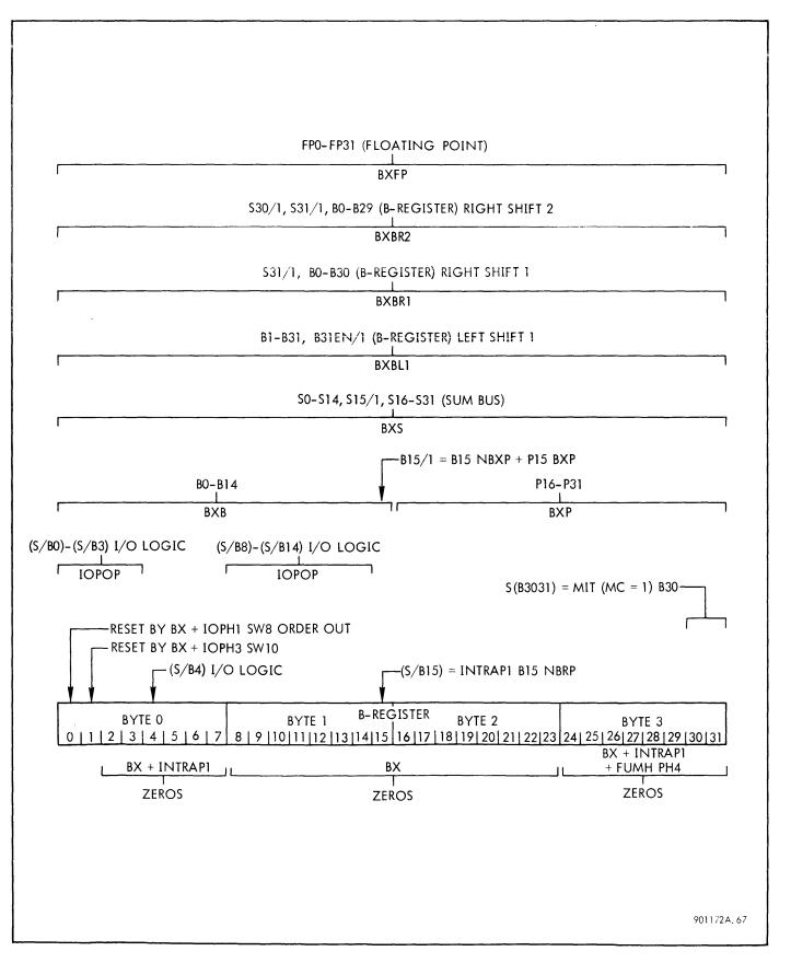
Figure 3-21. B-Register Inputs and Enabling Signals
