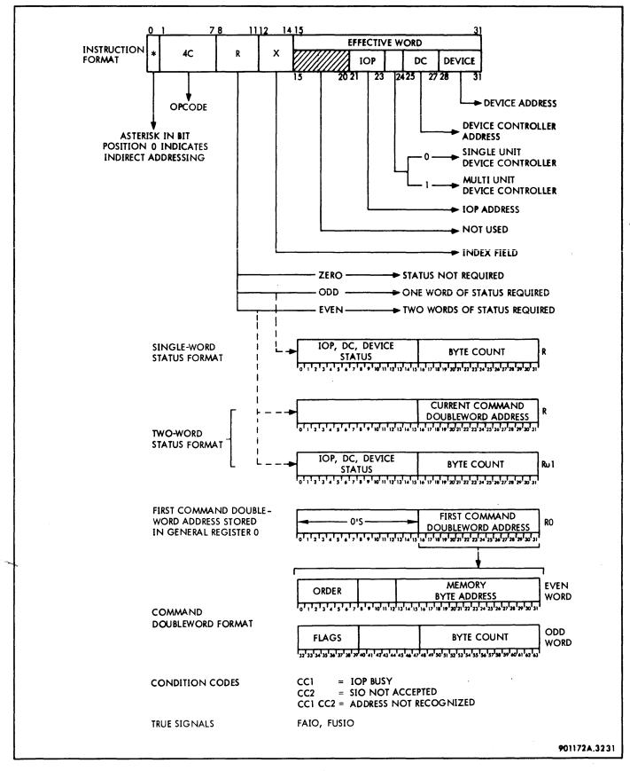
Figure 3-194. Start Input/Output Instruction Format
