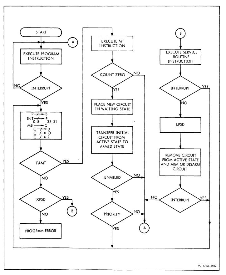
Figure 3-54. Interrupt Sequence, Flow Diagram
