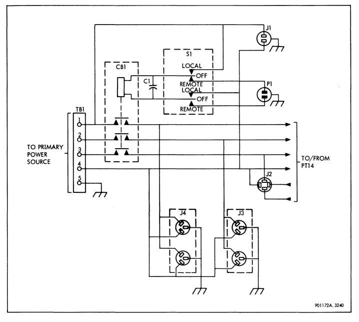
Figure 3-234. Main Power Distribution Box, Schematic Diagram
