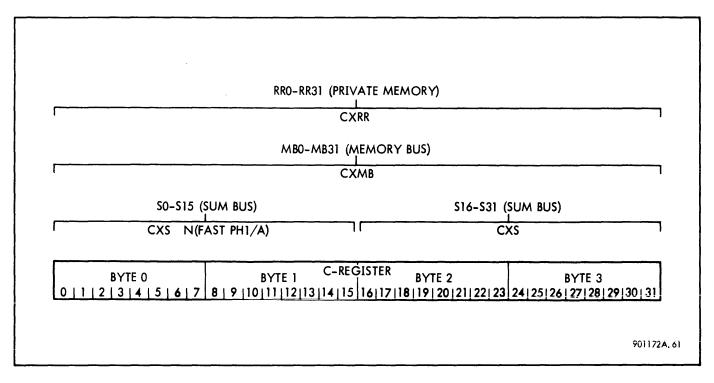
Figure 3-15. C-Register Inputs and Enabling Signals
