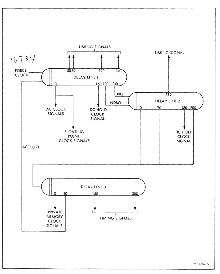
Figure 3-36. Clock Generator, Simplified Block Diagram
