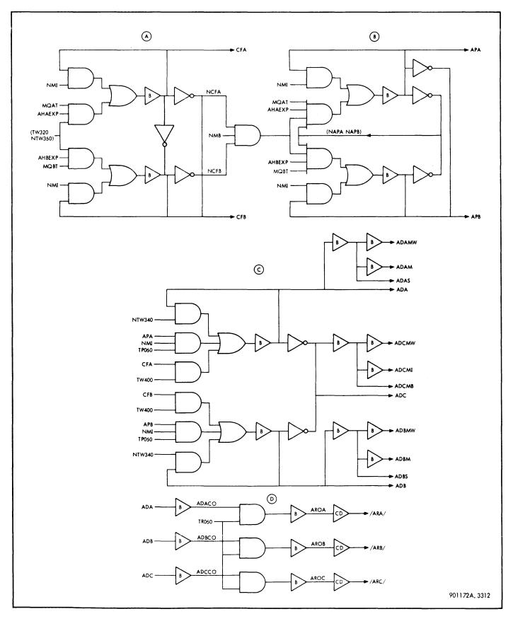
Figure 3-70. Port Priority and Address Release Logic
