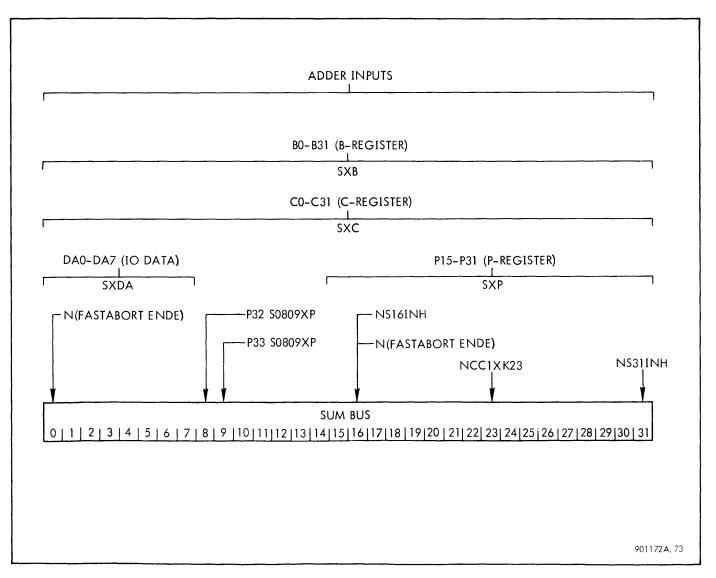
Figure 3-27. Sum Bus Inputs and Enabling Signals
