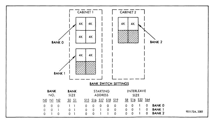
Figure 3-63. 32K Interleaved Memory, Example 2
