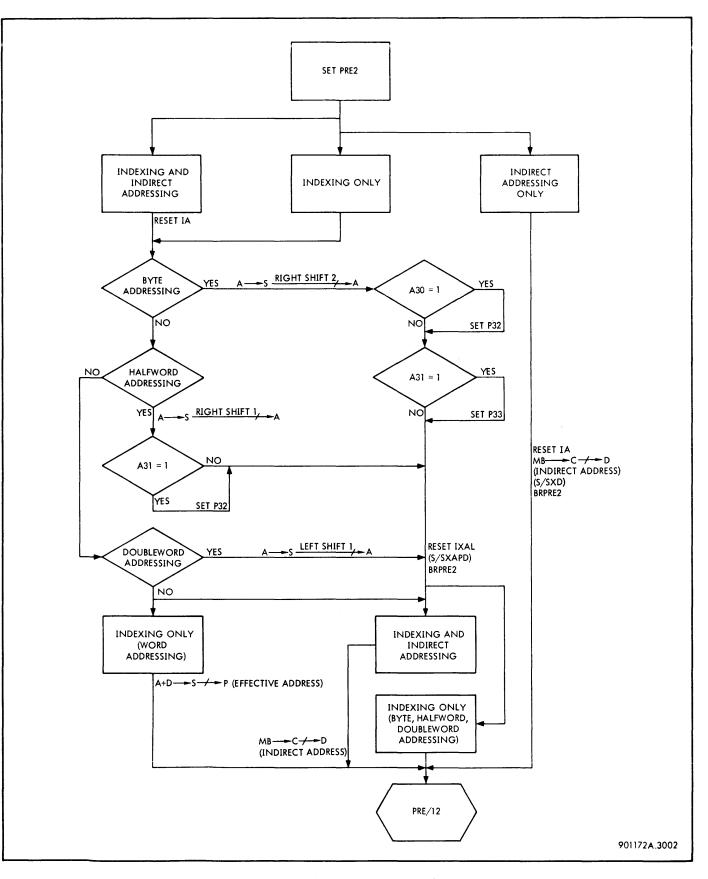
Figure 3-126. Preparation Phase PRE2 (Not PRE/12), Flow Diagram
