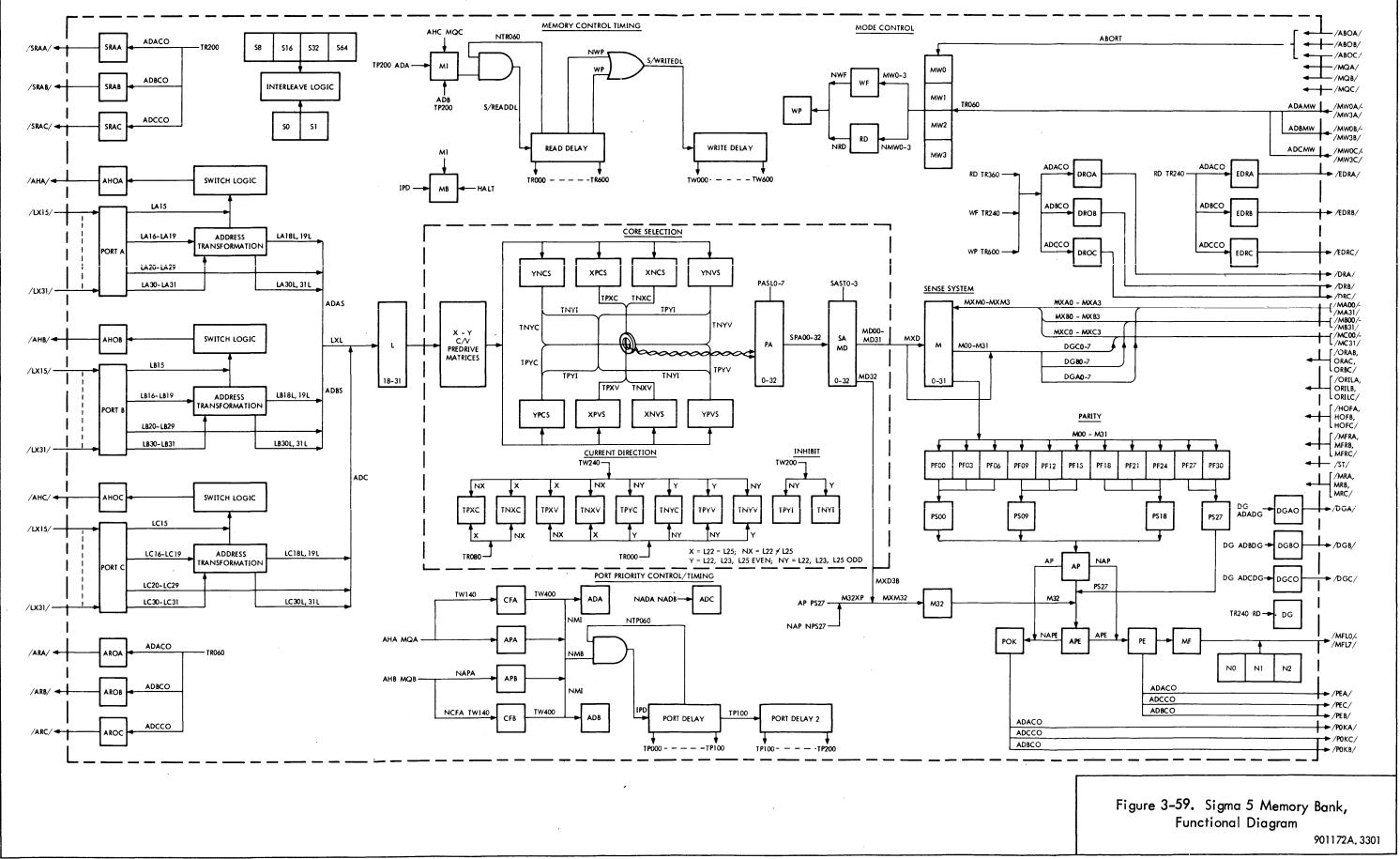
Before data is processed and stored in the magnetics section, the data is transferred to the M-register. For example, for data to be stored, the sequence occurs as follows:
