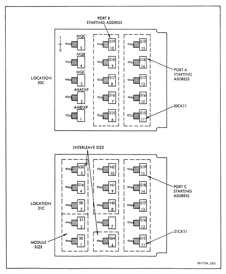
Figure 3-61. Toggle Switch Modules (ST14)
