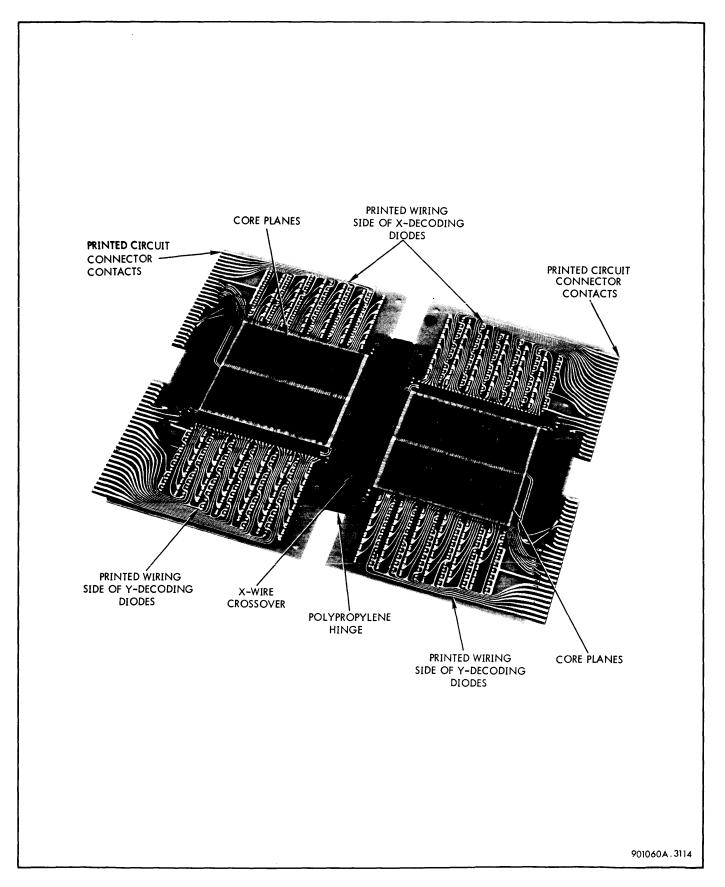
Figure 3-88. Core Diode Module, Open to Expose Bit Planes
