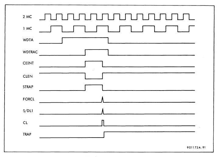
Figure 3-47. Watchdog Timer Runout, Timing Diagram
