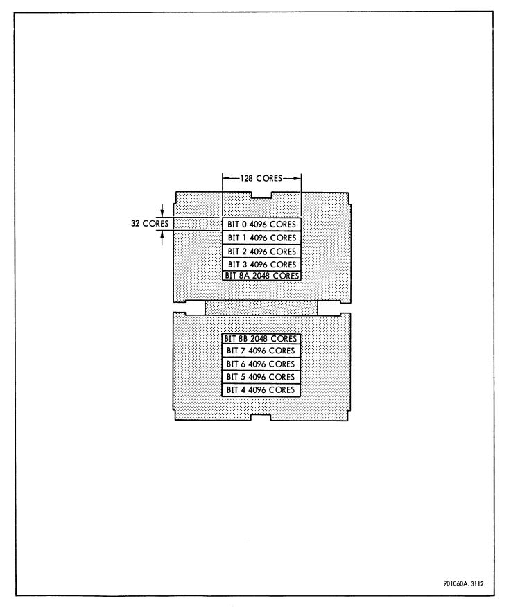
Figure 3-87. Bit Plane Layout in a Core Diode Module
