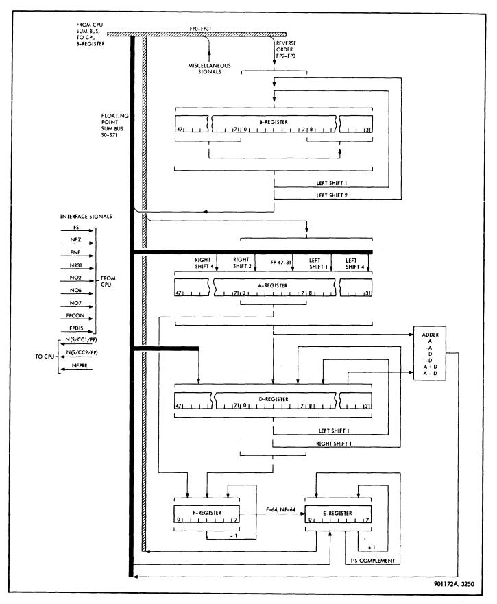
Figure 3-210. Floating Point Unit, Block Diagram
