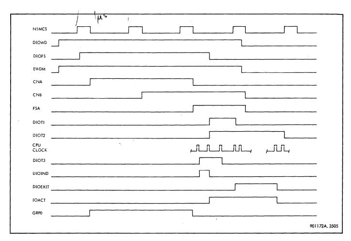
Figure 3-57. Write Direct Sequence, Timing Diagram
