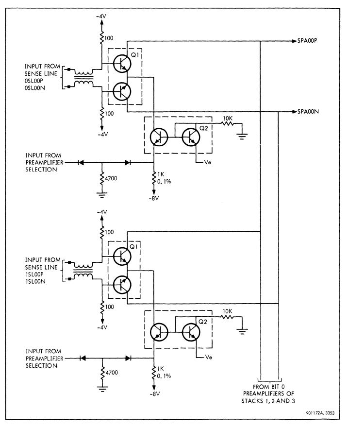
Figure 3-111. Sense Preamplifier (HT26) Simplified Schematic, Bit 0, Stack 0
