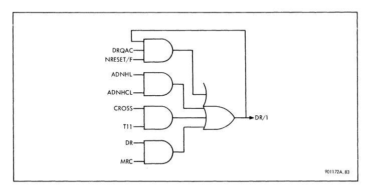
Figure 3-42. Data Release Latch, Logic Diagram
