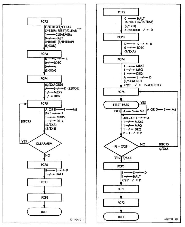
Figure 3-227. Clear Memory, Flow Diagram
