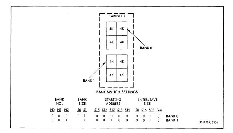
Figure 3–62. 32K Interleaved Memory, Example 1
