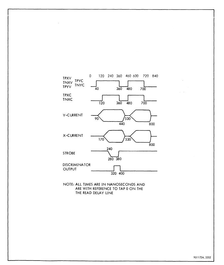
Figure 3–110. Magnetics Timing Diagram
