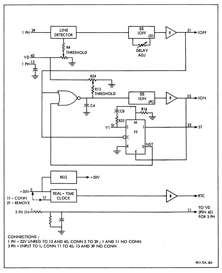
Figure 3-203. WT22 Line Detector, Block Diagram
