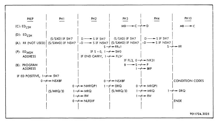
Figure 3–134. Load Absolute Doubleword Phases
