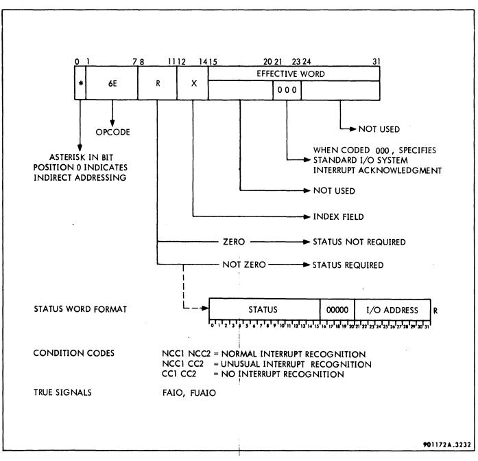
Figure 3-195. Acknowledge Input/Output Interrupt Instruction Format
