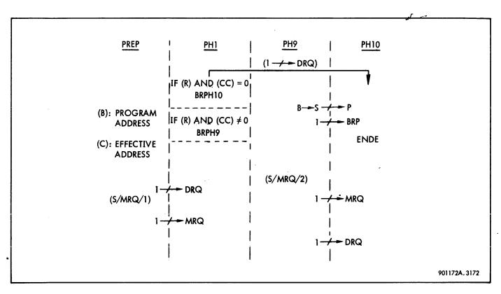
Figure 3-179. BCR Instruction, Phase Sequence Diagram
