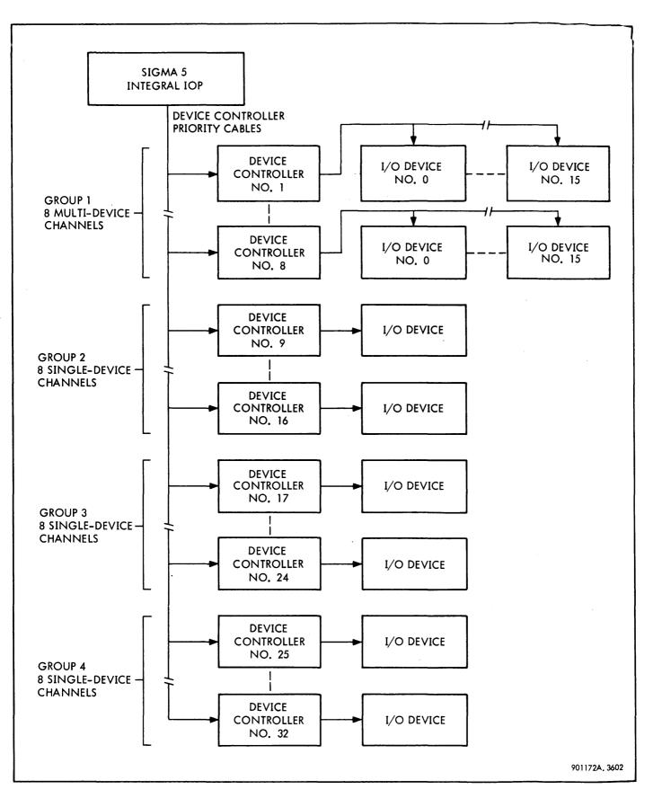
Figure 3-230. Integral IOP, Device Controller/Device Configuration
