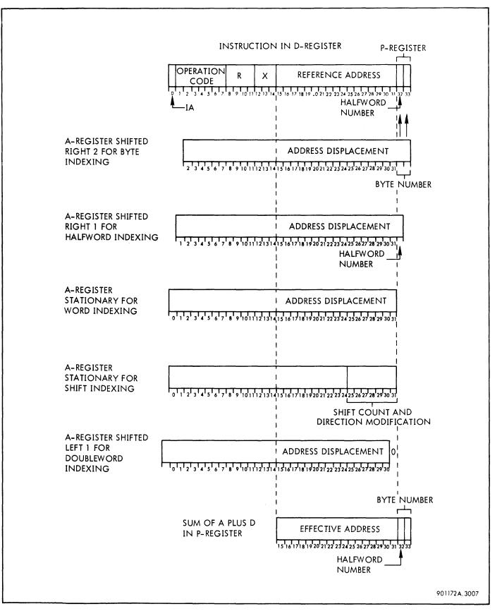
Figure 3-131. Index Register Alignment for Effective Address Computation
