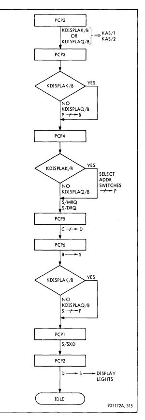
Figure 3-225. DISPLAY SELECT ADDR/DISPLAY INSTR ADDR, Flow Diagram
