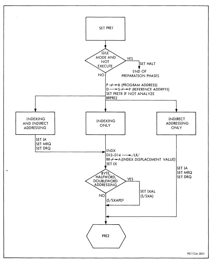
Figure 3-125. Preparation Phase PRE1, Flow Diagram
