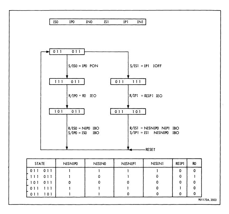
Figure 3-55. Power-On and Power-Off Interrupt Circuits, Cycle of Operation
