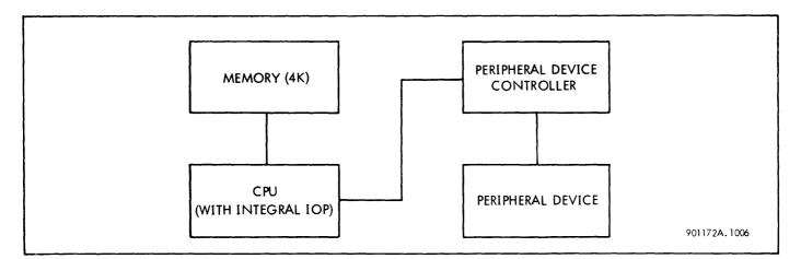
Figure 1-6. Sigma 5 Minimum System With Integral IOP
