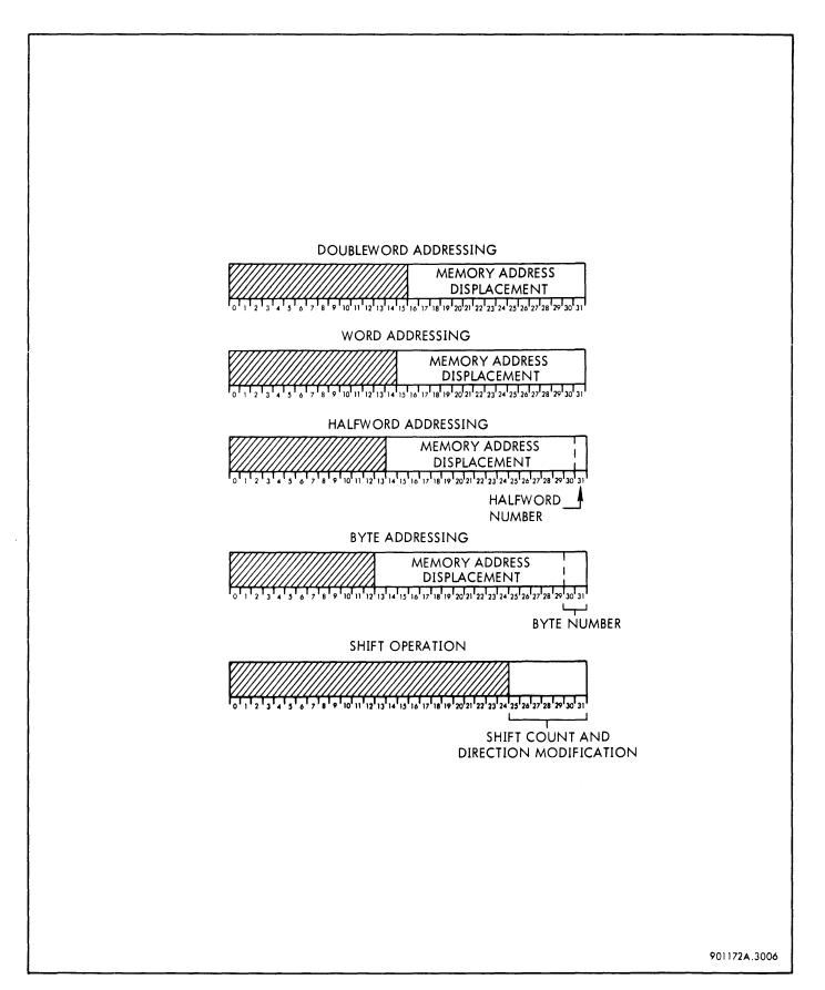
Figure 3-130. Index Register Contents for Byte, Halfword, Word, Doubleword, and Shift Operations
