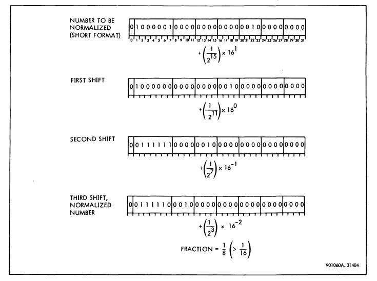
Figure 3-167. Normalization of Floating Point Numbers
