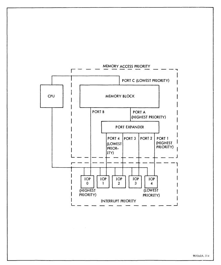
Figure 3-12. Typical IOP Priority Arrangement
