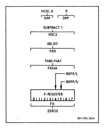
Figure 3-214. Floating Point F-Register Inputs and Enabling Signals
