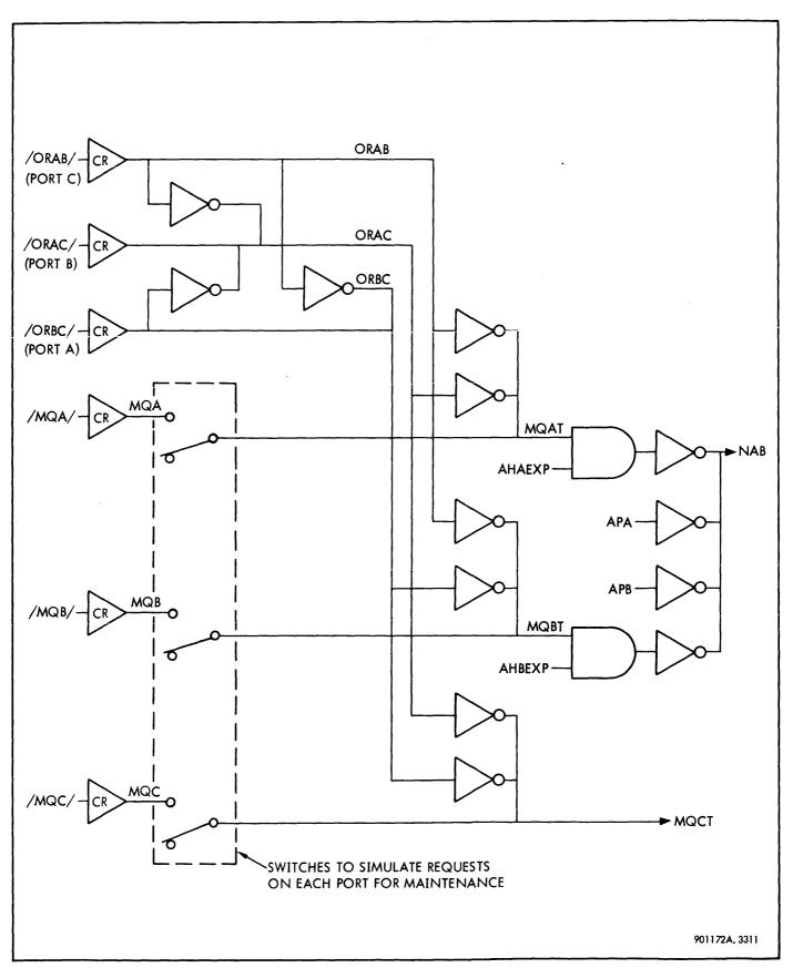
Figure 3-69. Memory Request and Port Override Logic
