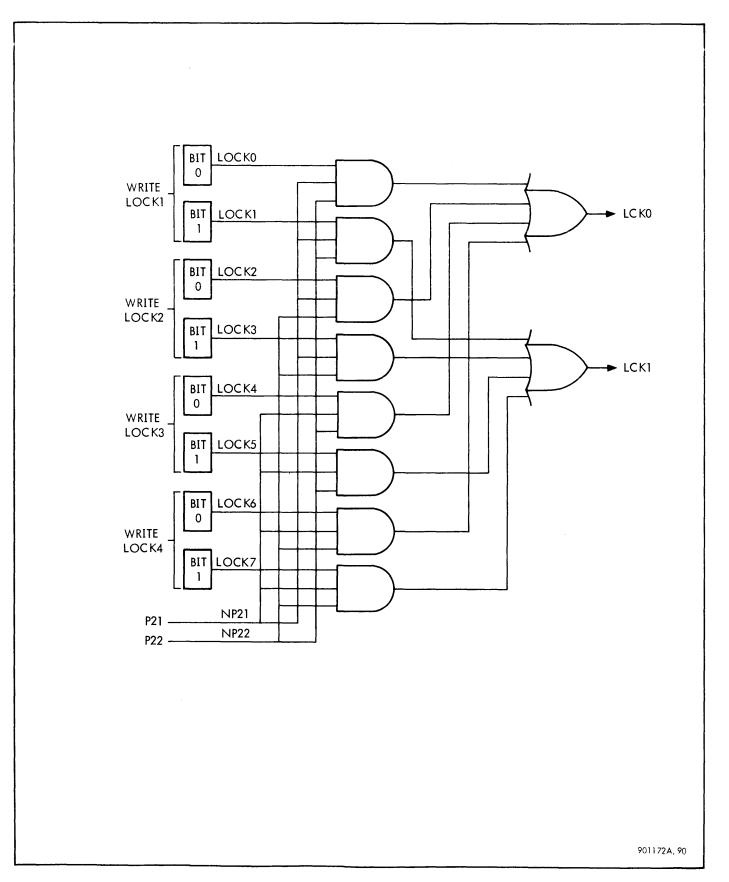
Figure 3-50. Write Lock Addressing
