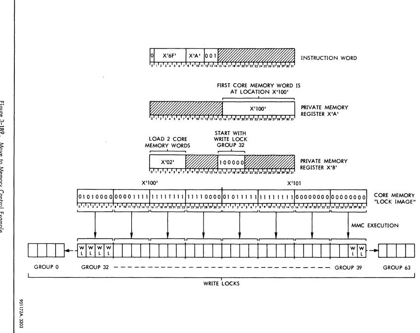
Figure 3-189. Move to Memory Control Example
