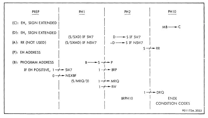
Figure 3-132. Load Absolute Halfword Phases
