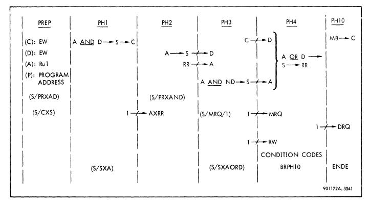
Figure 3–136. Load Selective Phases
