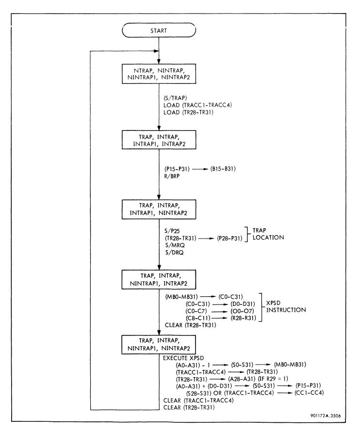
Figure 3-51. Trap Sequence, Flow Diagram
