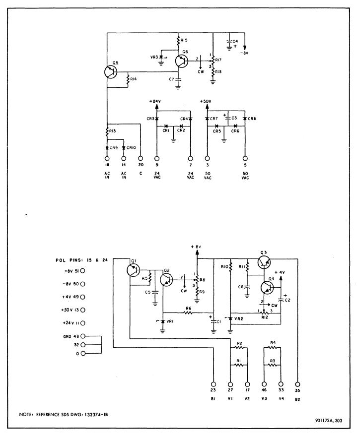
Figure 3-202. WT21 Regulator, Schematic Diagram
