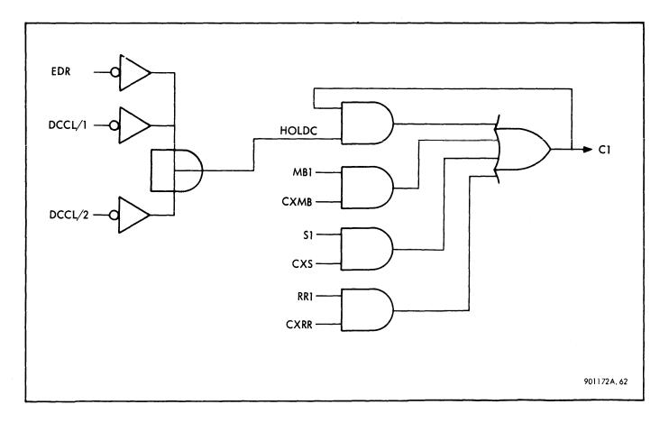
Figure 3-16. C-Register Bit 1 Logic Diagram
