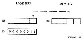
The binary addition of the contents of index register R4 to the virtual operand address of the instruction is performed in the following manner:
