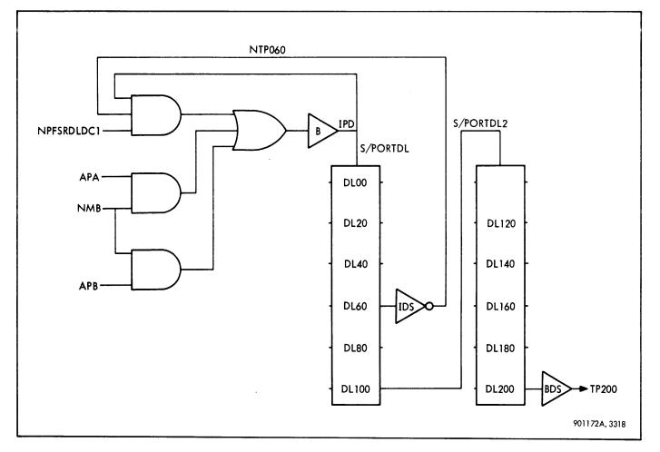
Figure 3-76. Ports A and B Delay Line
