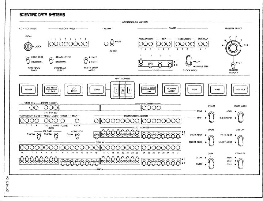
Figure 2-1. Sigma 5 Processor Control Panel (PCP)
