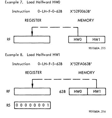
In each of the load halfword instructions shown in examples 7 and 8, the sign of the halfword is extended 16 places to the left before it is loaded into register RF. Thus, if the contents of instruction HW0 in example 7 were X'FFOA', register RF would be loaded with X'FFFFFFOA'; if the contents of instruction HW1 in example 8 were X'0004', register RF would be loaded with X'00000004'.
