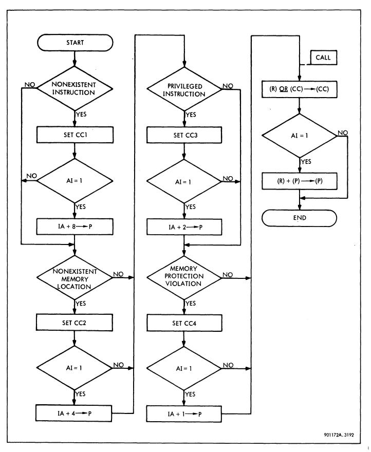
Figure 3-185. Exchange Program Status Doubleword Instruction, Flow Diagram
