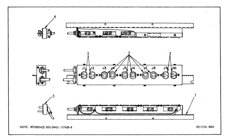
Figure 4-7. Power Distribution Box Assembly
