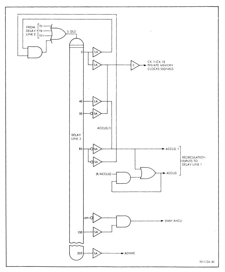
Figure 3-39. Delay Line 3, Logic Diagram
