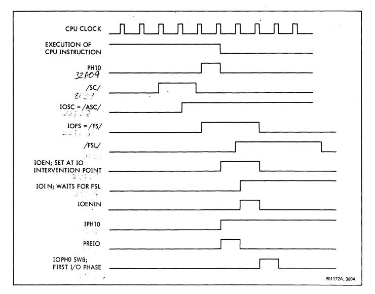
Figure 3-233. Service Call Connect Phases, Typical Timing Sequence
