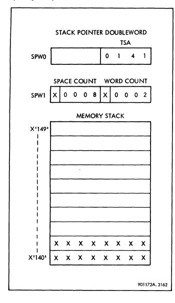
Example. An example of a memory stack with the corresponding stack pointer doubleword is shown below.
