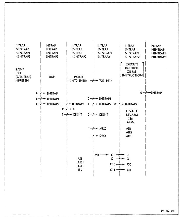
Figure 3–53. Interrupt Phases
