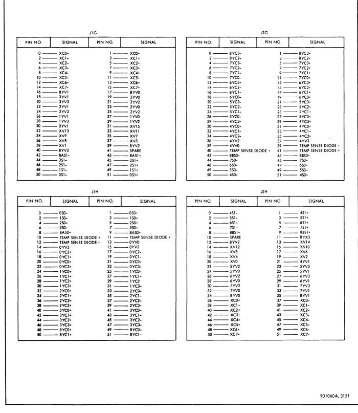
Figure 3-91. Core Diode Module, Jack Pins and Signals
