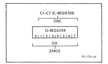
Figure 3-18. O-Register Inputs and Enabling Signals
