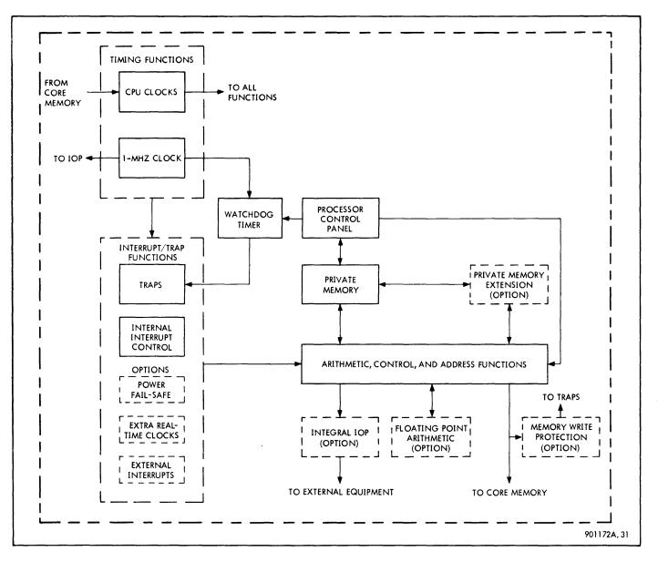
Figure 3-2. Central Processing Unit, Functional Block Diagram
