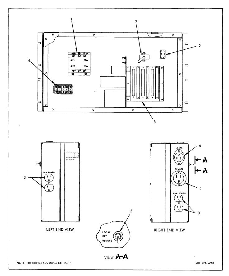
Figure 4-5. Power Distribution Assembly
