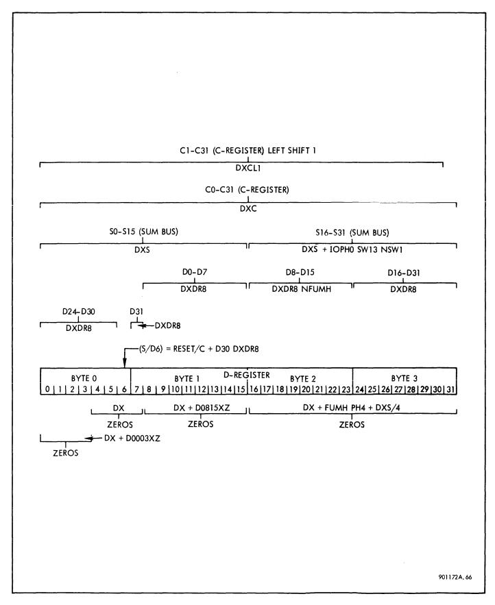
Figure 3-20. D-Register Inputs and Enabling Signals
