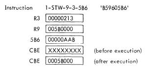
The virtual address X'5B6' in the instruction word is translated into a second virtual address X'AAB'. The contents of register R3 are added to this second virtual address and the sum (CBE) becomes the effective address of the memory location into which the operand in register R9 is stored.
