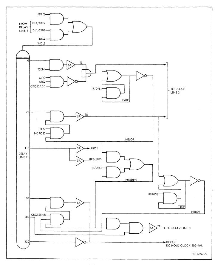
Figure 3-38. Delay Line 2, Logic Diagram
