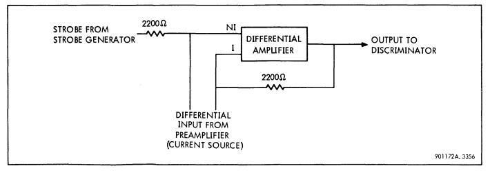
Figure 3-114. Basic Sense Amplifier, Logic Diagram
