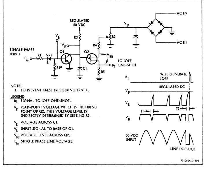
Figure 3-206. Single-Phase Detection
