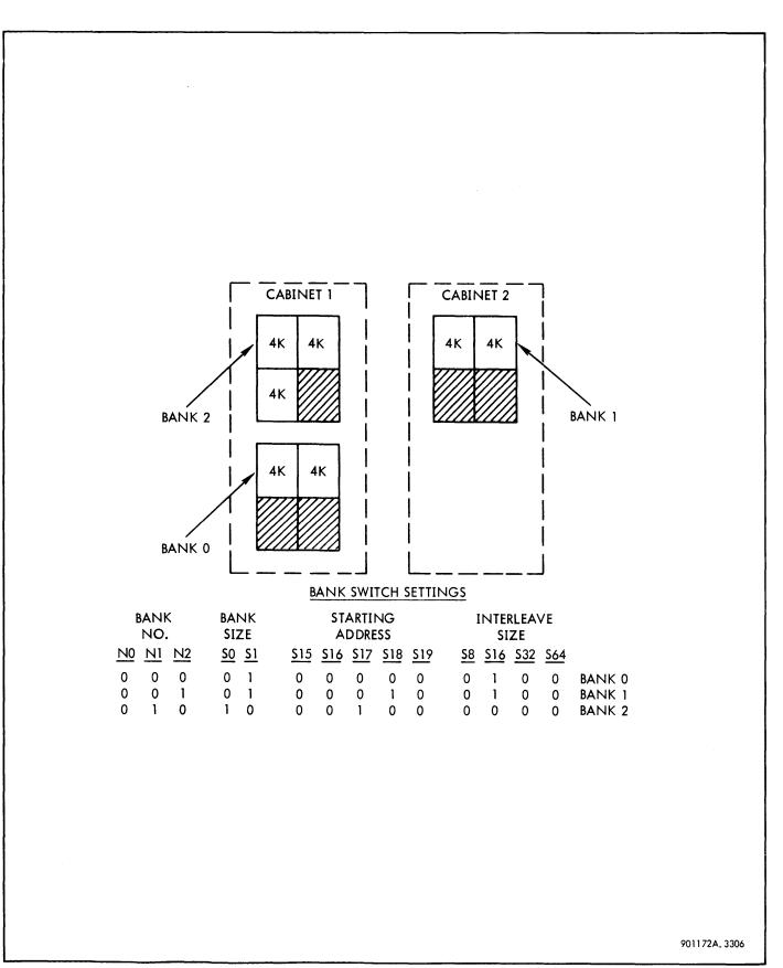
Figure 3-64. 32K Interleaved Memory, Example 3
