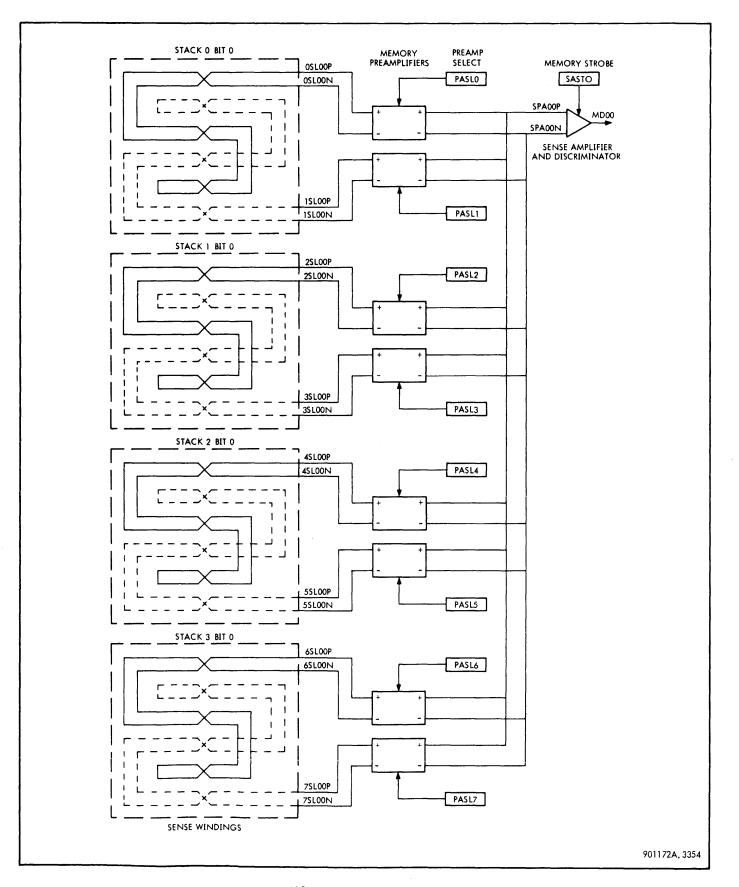
Figure 3-112. Sensing System for Bit 0 (Typical)
