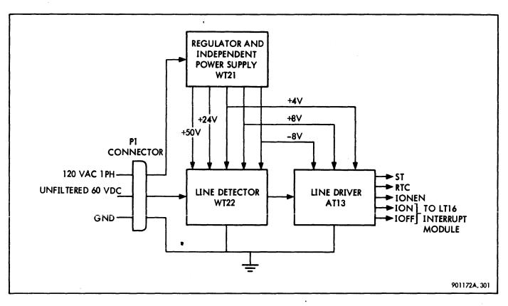
Figure 3-200. Power Monitor Assembly, Simplified Block Diagram
