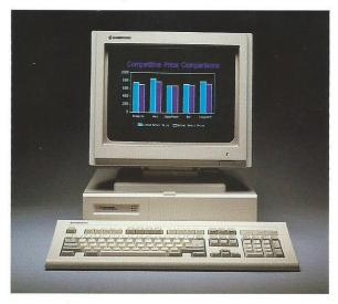
The PCterminal/386SX is a fully AT compatible diskless LAN workstation. Features a built-in Ethernet interface and is compatible with all versions of Novell NetWare.
