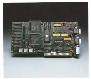
The 8-bit SVGA1 provides up to 800 x 600 resolution and is compatible with a wide range of video standards including VGA, EGA, CGA, MDA and Hercules graphics. Includes software drivers for Ventura Publisher®, Aldus PageMaker® Windows, GEM and AutoCAD/AutoSHADE®.
