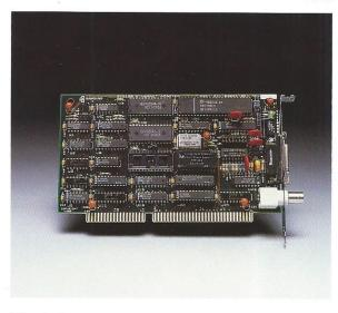
The SE2100 is a high-performance, 16-bit memory-mapped Ethernet interface card for all PC's and compatibles. Maximum performance in both fileservers and LAN workstations. Provides up to twice the overall system throughput of other cards.
