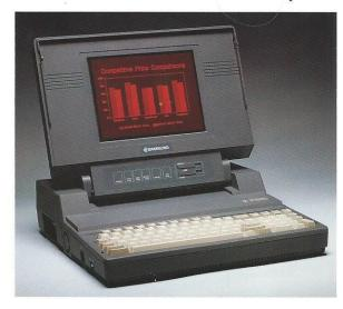
Compact, high-speed portable with all the features of advanced desktop computers, including a built-in 32MB hard disk drive and 640 x 400 gas-plasma display with external EGA video port.
