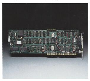
The DCB/FDC is a high-performance SCSI controller adapter for network fileservers, boosting disk throughput with faster data transfers, higher reliability and enhanced data integrity.
