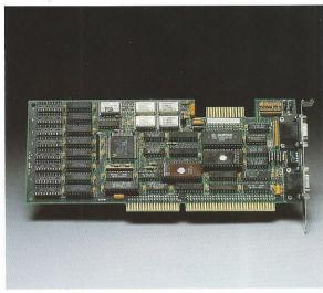
Offers superior resolution, and compatibility with all popular video standards including Super-VGA, VGA, EGA, CGA, MDA and Hercules graphics. Delivers 1,024 x 768 and 800 x 600 resolution and includes software drivers for Ventura Publisher, Aldus Pagemaker, Windows, GEM, and AutoCAD/AutoSHADE.
