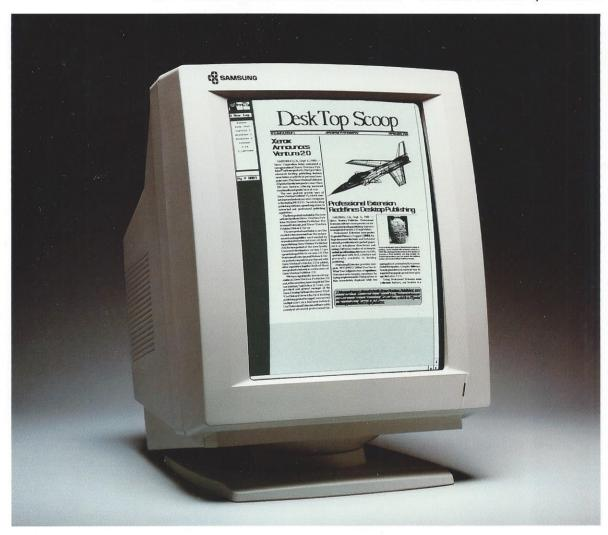
A full-page vertical display with 1,006 x 1,048 (IBM®) or 640 x 870 (Apple® Mac II® and Mac SE®) resolution designed for desktop publishing applications. Sharp, crisp images for CAD, complex graphics and full-screen wordprocessing or spreadsheets. Includes video card and software drivers disk.
