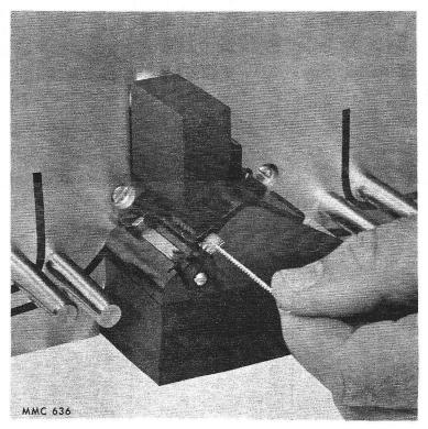
Figure 5.0. Brush Insertion for Readhead Cleaning.
