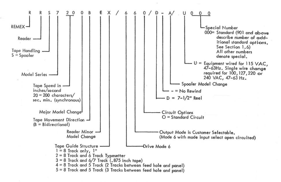
Figure 1-3. Model Number Coding For RRS7200.
