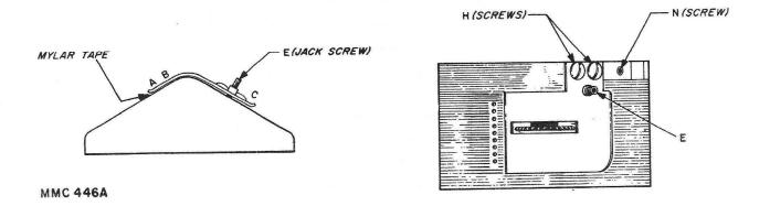
Figure 5-4. Adjustment of the Upper Tape Guide.
