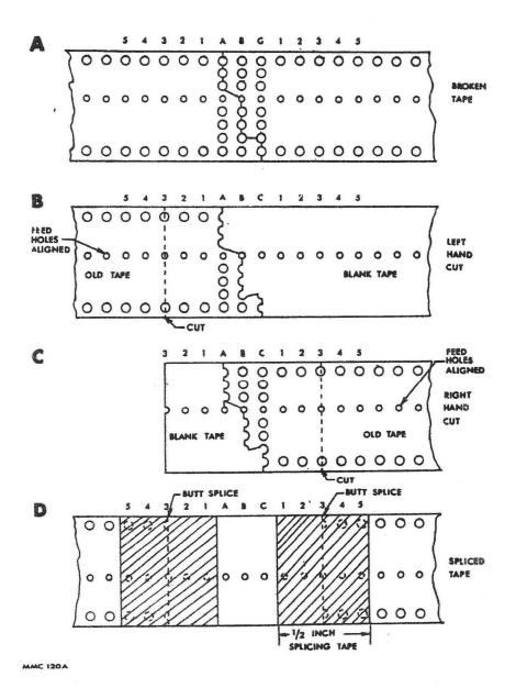
Figure 5-5. Tape Splicing Procedure.
