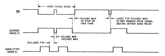
Figure 3-5. Timing Diagram for Reader
