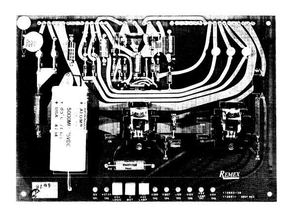
Figure 7-14. Reader Card Assembly 110801-003 (Top) and Power Supply Card Assembly 113681-001 (Bottom).
