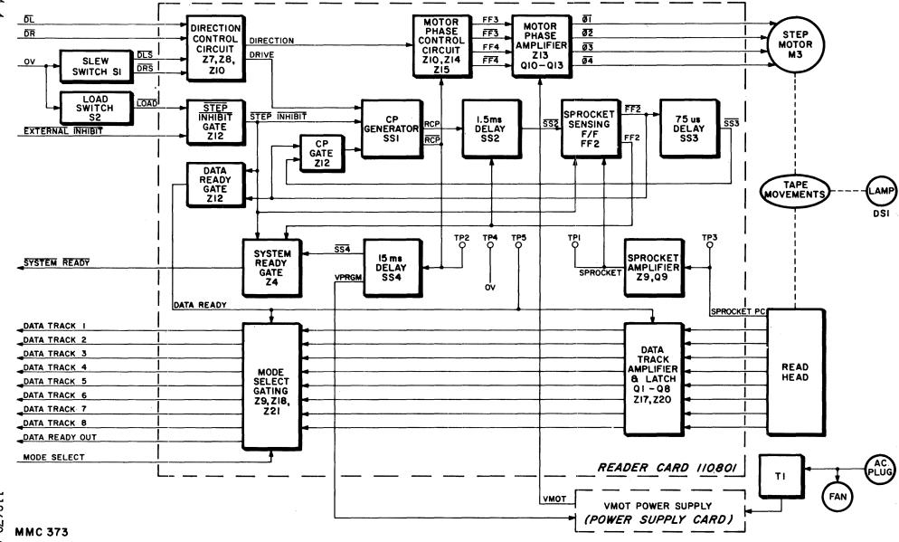
Figure 4-2. Block Diagram, Reader Section
