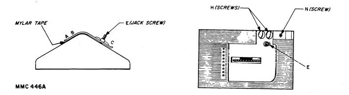
Figure 5-6. Adjustment of the Upper Tape Guide.
