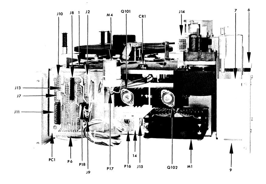
Figure 7-6. Chassis Assembly 113688-001, Inside View.
