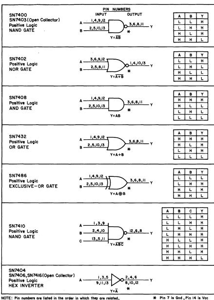
NOTE: Pin numbers are listed in the order in which they are related, for EXAMPLE, on SN7410, pins 1, 2, 13 and 12 function together on one gate.
