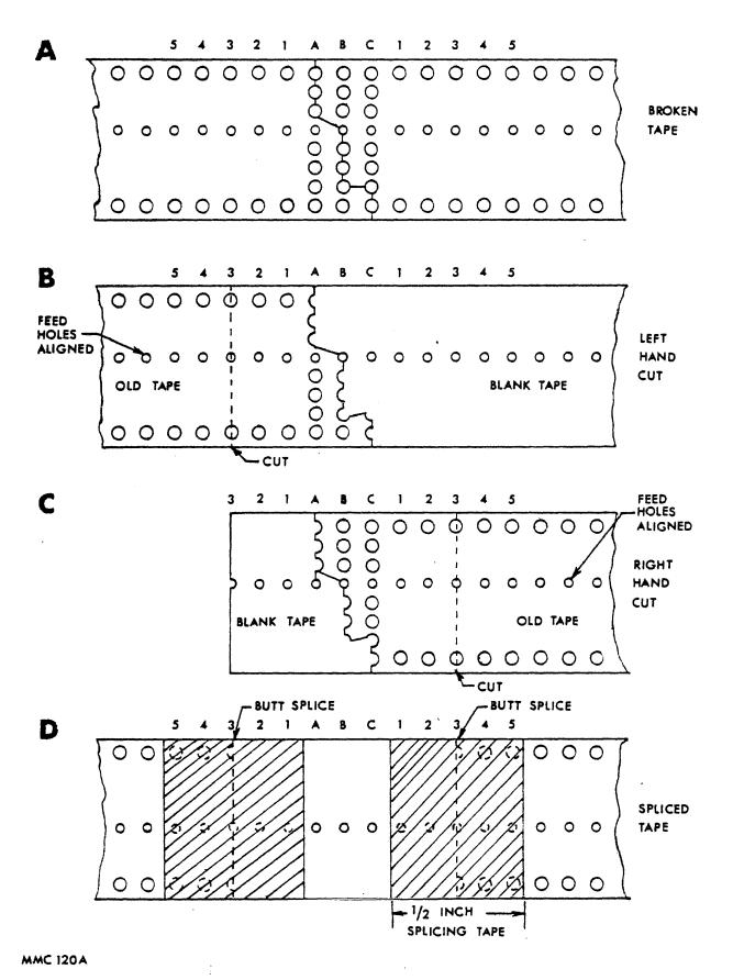
Figure 5-9. Tape Splicing Procedure
