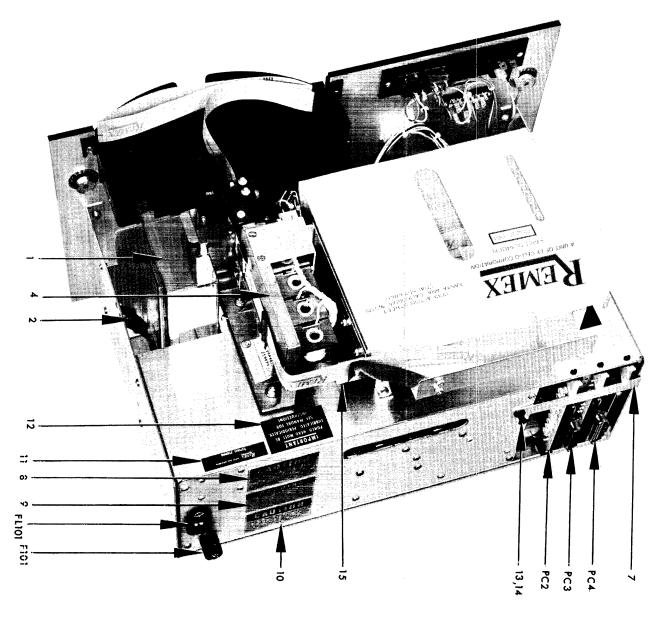
Figure 7-12. Top View, RAF612X.
