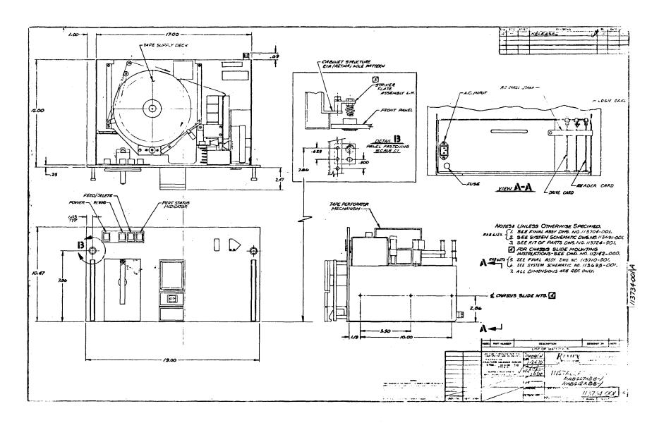
Figure 1-4. Installation Drawing, Model RAB612X.
