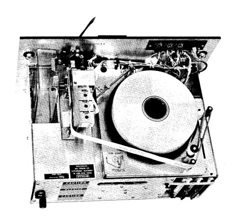
Figure 3-1. Tape Loading, Roll Type Tape
