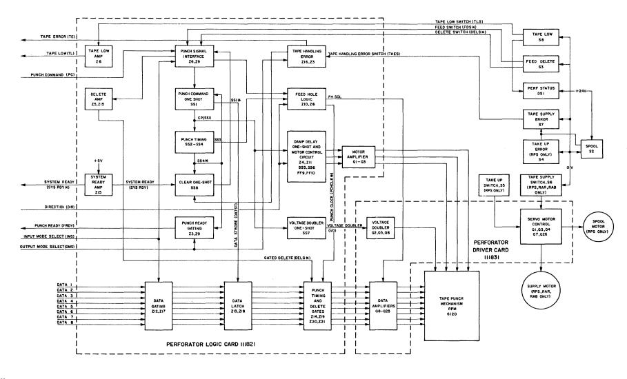
Figure 4-1. Block Diagram, Perforator Section
