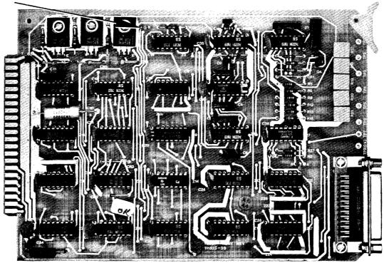
Figure 7-13. Perforator Driver Card Assembly 111831-001 (Top) and Perforator Logic Card Assembly 111821-001 (Bottom).
