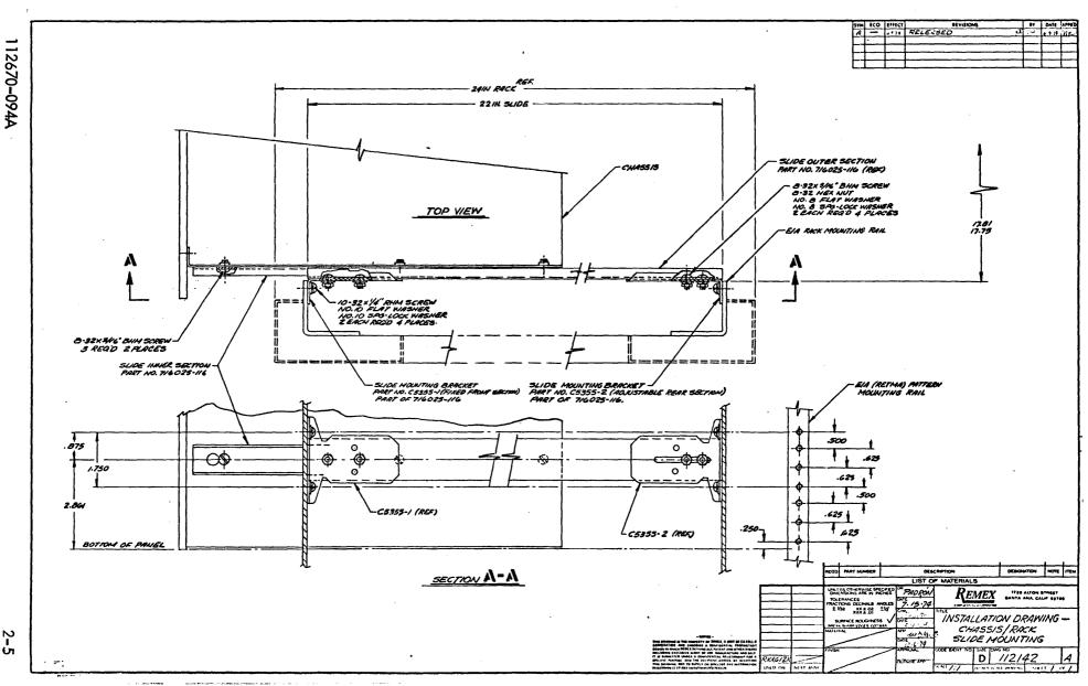
Figure 2-3. Chassis Slide Installation
