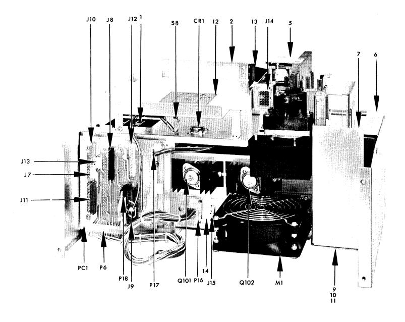
Figure 7-11. Chassis Assembly 113687-001, Inside View.
