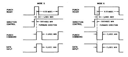
Figure 3-4. Timing Diagram, Perforator Section
