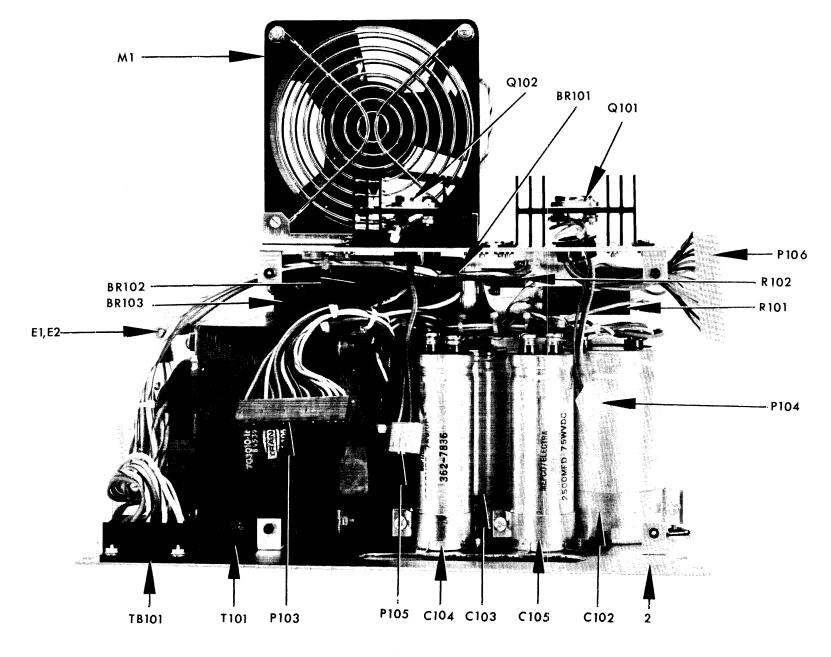
Figure 7-7. Power Supply Chassis Assembly 113680-001.
