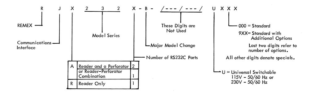
Figure 1-5. REMEX Model Number Coding.
