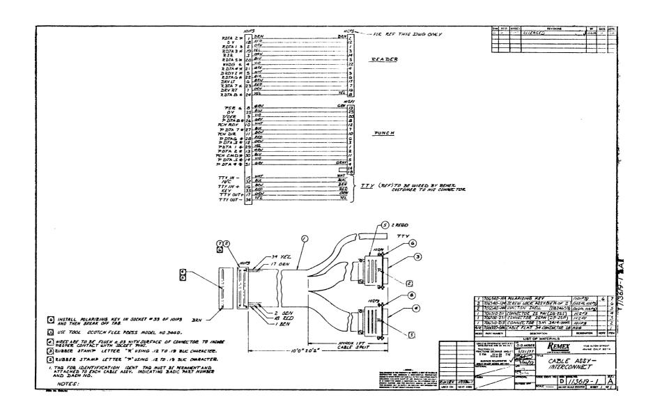
Figure 2-2. Interconnect Cable Assembly, 113619-001.
