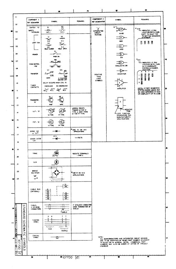
Figure 8-2. REMEX Standard Schematic Symbols, Sheet 1 of 2.
