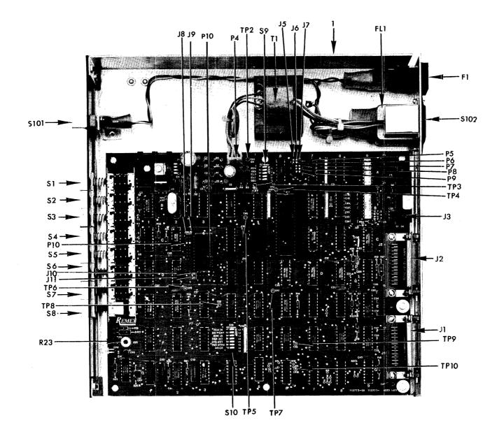
Figure 7-3. Chassis Assembly, Model RJA2322.
