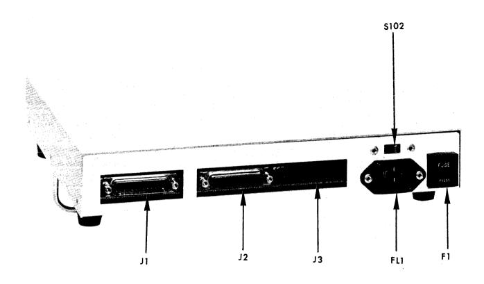
Figure 2-3. Rear View of RJA2322 Showing Location of Connectors, Fuse and A.C. Power Select Switch.
