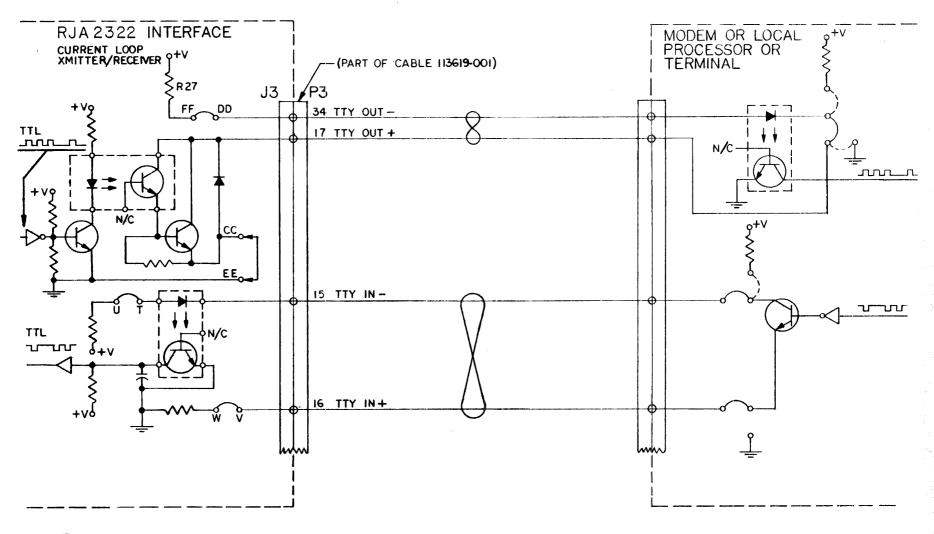
Figure 3-4. Typical Serial Connection 20 mA Current Loop.
