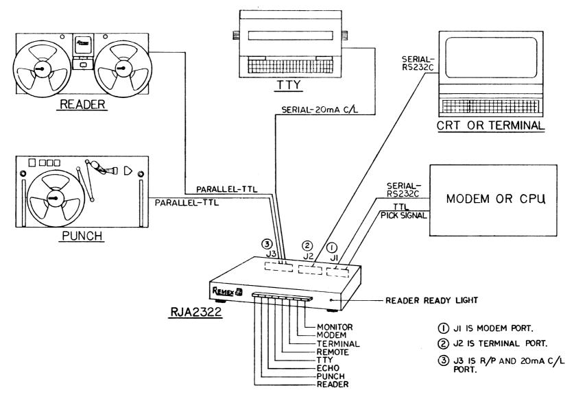
Figure 3-3. Typical Multidevice System Configuration RS - 232 - C and Current Loop Connections.
