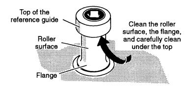
Figure 6-3 Cleaning the Tape Guides
