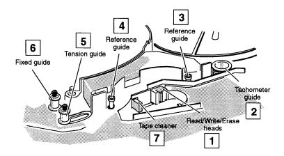
Figure 6-1 Tape Path Components That Must Be Cleaned
