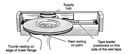
Figure 3-5 Correct Way to Insert Reel
