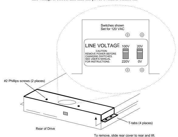
Figure 8-1 AC Power Configuration Switches
