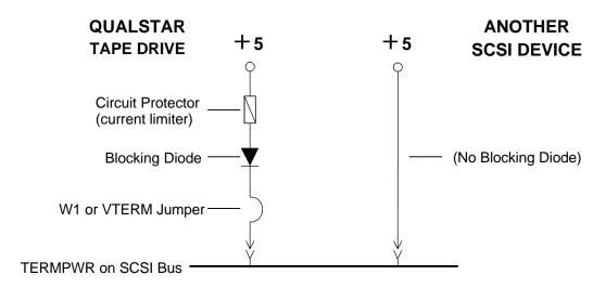
Figure 1-9 Diagram of SCSI Termination Power
