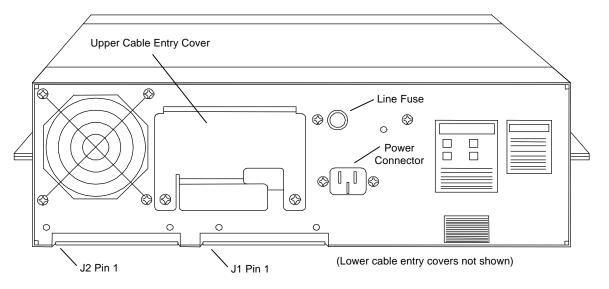
Figure 1-10 Industry Standard Interface Connector Placement
