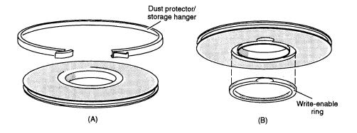
Figure 3-3 Dust Protector and Write-enable Ring
