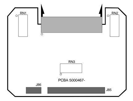
Figure 1-5 SCSI Differential Adapter PCBA
