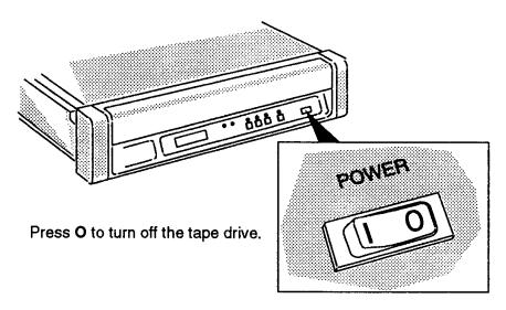
Figure 3-1 Power Switch Location
