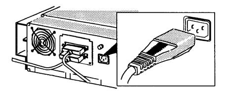
Figure 3-2 Power Connection Location
