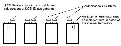
Figure 1-6 SCSI Cable Configurations
