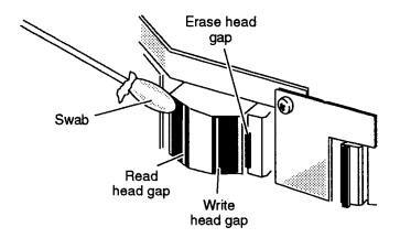
Figure 6-2 Cleaning the Read/Write Head
