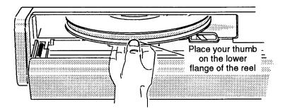
Figure 3-7 Correct Method of Removing Tape Reel
