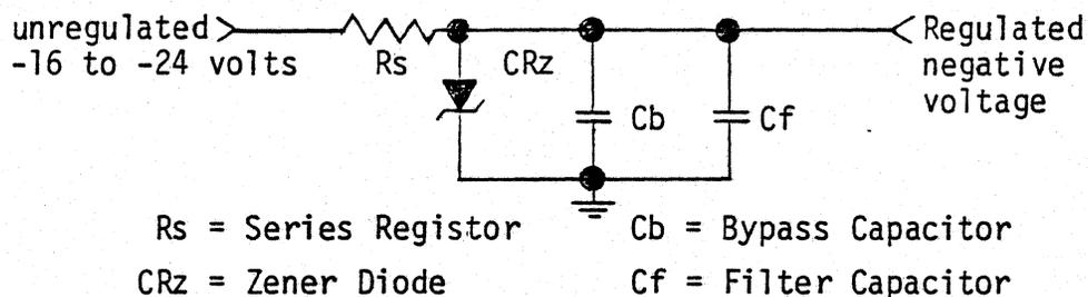
The bypass capacitor ( $C_b$ ) should be a  $0.1_{\mu}$  F or  $0.01_{\mu}$  F ceramic disc; the value is not critical. The filter capacitor ( $C_f$ ) should be a  $10_{\mu}$  F 25-35 volt tantalum with the positive lead to ground (ground is positive with respect to the negative regulated voltage).
