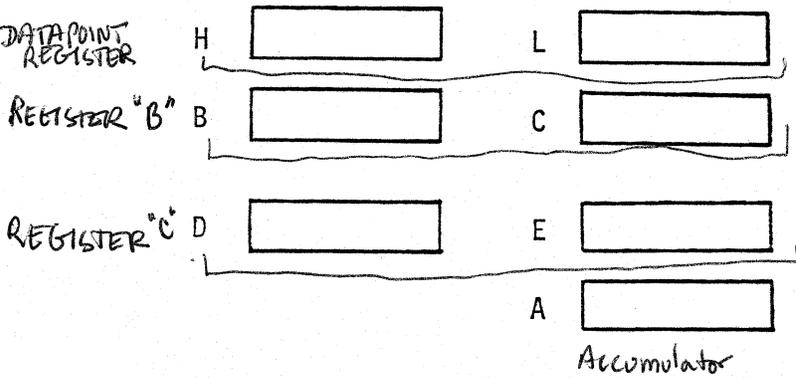
So far, we have the memory space; a data pointer register; a program counter register; working registers (two pairs, each one holding one byte); and an accumulator. Let us consider the working registers.
