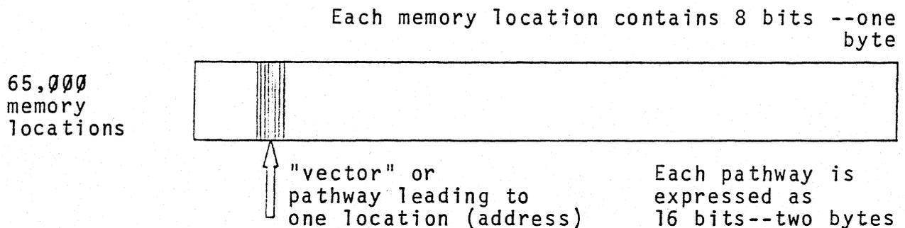
with the bar representing the bytes of 8-bit groups within the memory, and the large arrow indicating the 16-bit address that specifies the pathway leading to each memory location.
