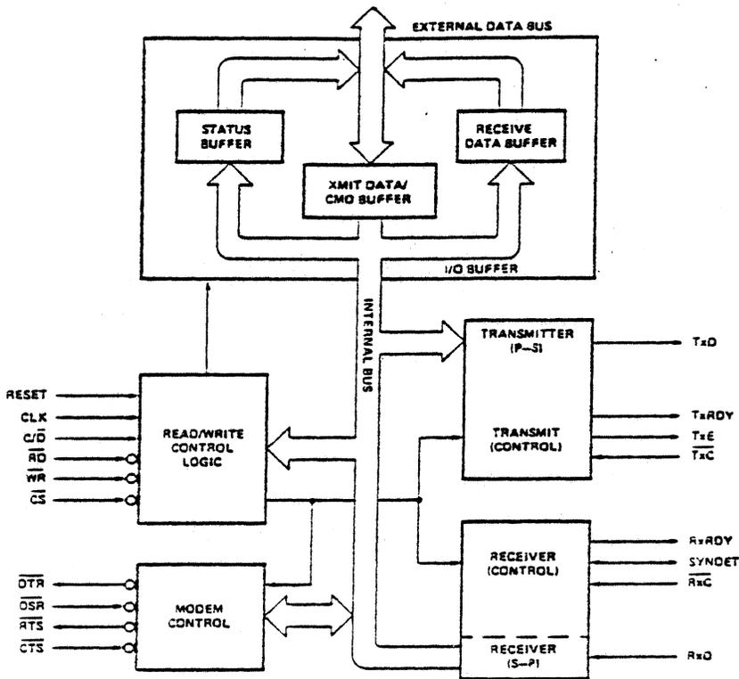
Figure 2. 8251 Block Diagram
