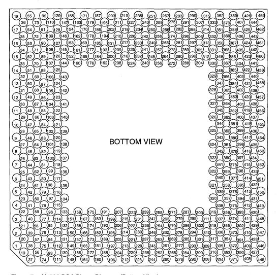
Figure 7 Nx586 PGA Pinout Diagram (Bottom View)
