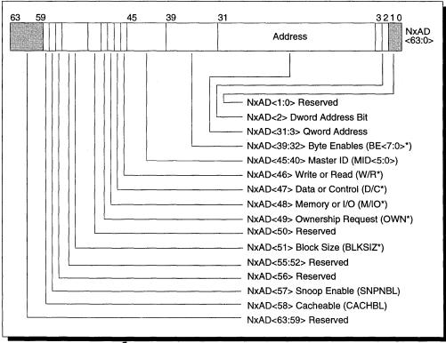
Figure 10 NexBus/NexBus<sup>5</sup> Address and Status Phase
