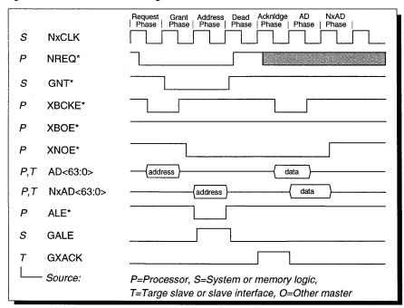
Figure 32 Fastest NexBus Single-Qword Write
