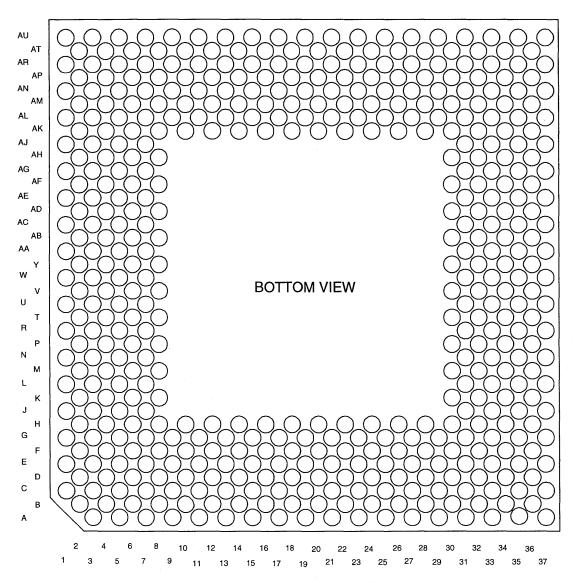
Figure 9 Nx586 JEDEC Pinout Diagram (Bottom View)
