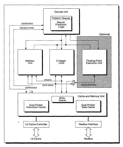
Figure 19 Nx586 Internal Architecture
