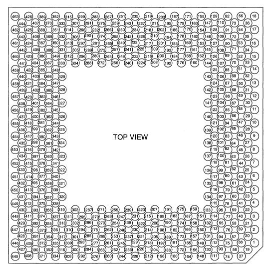
Figure 6 Nx586 PGA Pinout Diagram (Top View)
