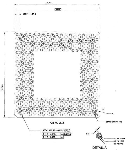
Figure 44 Nx586 Package Diagram (bottom)
