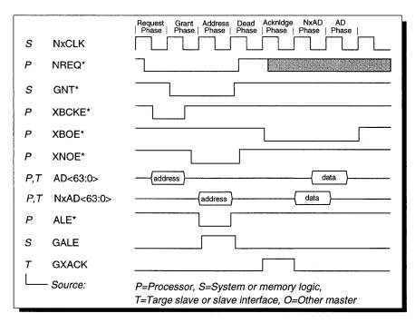
Figure 31 Fastest NexBus Single-Qword Read
