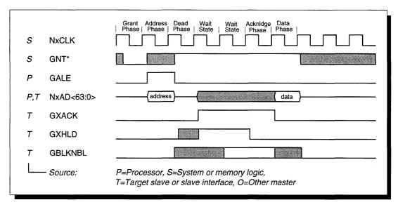
Figure 36 NexBus<sup>5</sup> Single-Qword Read with Wait States using GXHLD only
