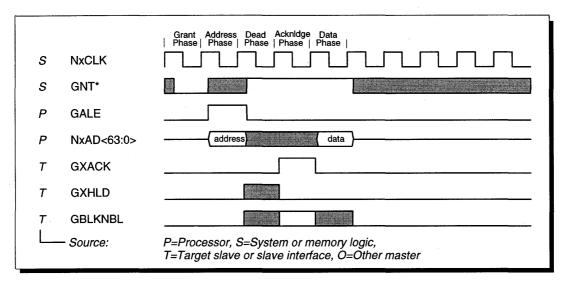
Figure 37 Fastest NexBus<sup>5</sup> Single-Qword Write
