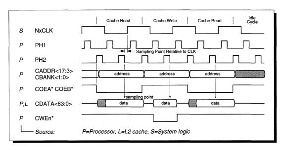
Figure 28 Level-2 Asynchronous Cache Read and Write
