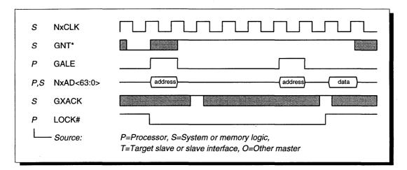
Figure 39 Interrupt Acknowledge Cycle
