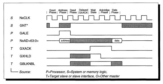
Figure 38 NexBus<sup>5</sup> Single-Qword Write With Wait States
