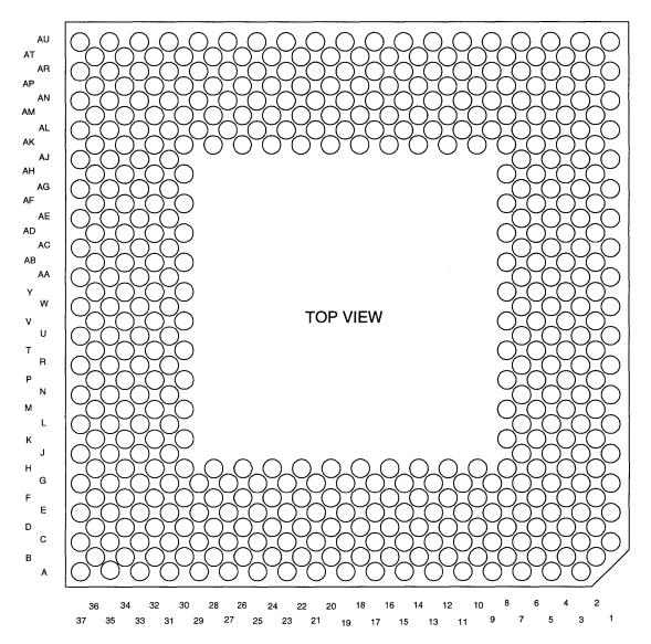
Figure 8 Nx586 JEDEC Pinout Diagram (Top View)
