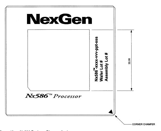
Figure 42 Nx586 Package Diagram (top)
