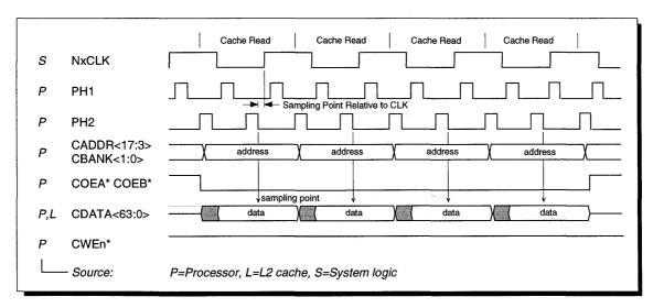
Figure 29 Level-2 to Level-1 Asynchronous Cache Line Fill.
