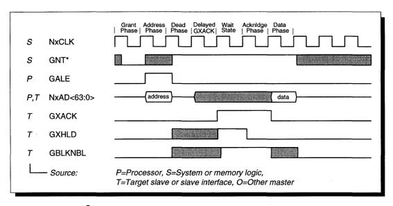
Figure 35 NexBus<sup>5</sup> Single-Qword Read with Wait States using a delayed GXACK
