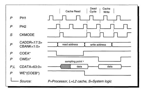
Figure 30 Level-2 Synchronous Cache Read and Write cycles
