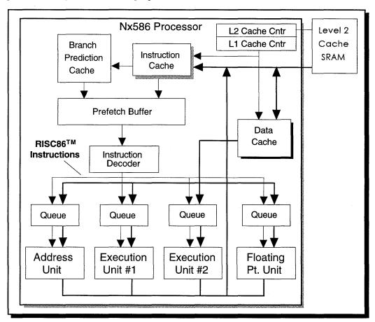
Figure 1 Nx586 Functional Block Diagram
