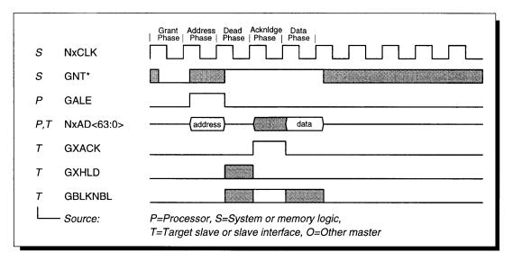
Figure 33 Fastest NexBus<sup>5</sup> Single-Qword Read
