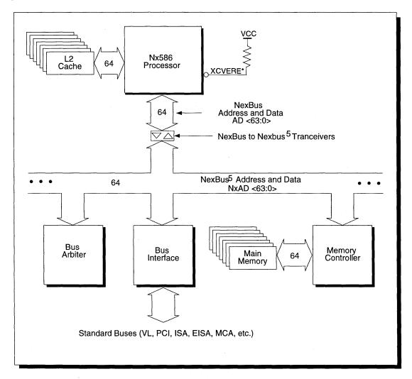
Figure 15 Nx586 Basic System Diagram
