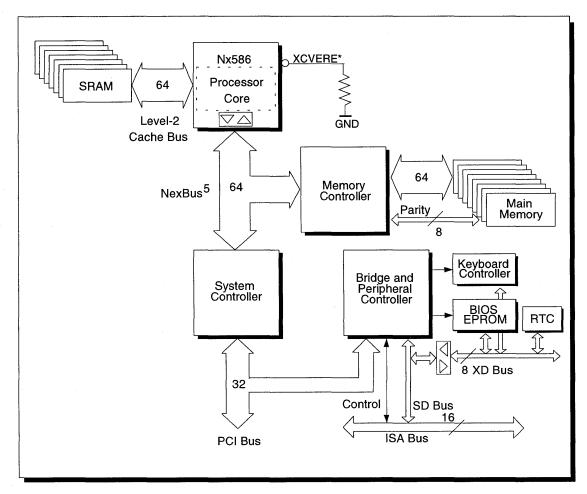
Figure 17 Example System with the Nx586 and NexBus<sup>5</sup>.
