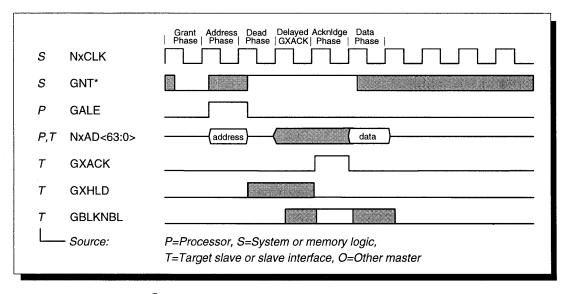
Figure 34 Fast NexBus<sup>5</sup> Single-Qword Read with a delayed GXACK
