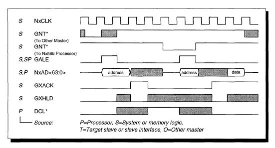
Figure 41 NexBus<sup>5</sup> Single-Qword Read Hits Modified Cache Block
