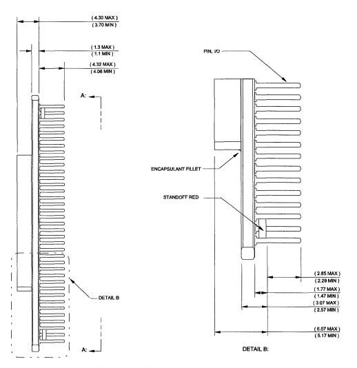
Figure 43 Nx586 Package Diagram (side)
