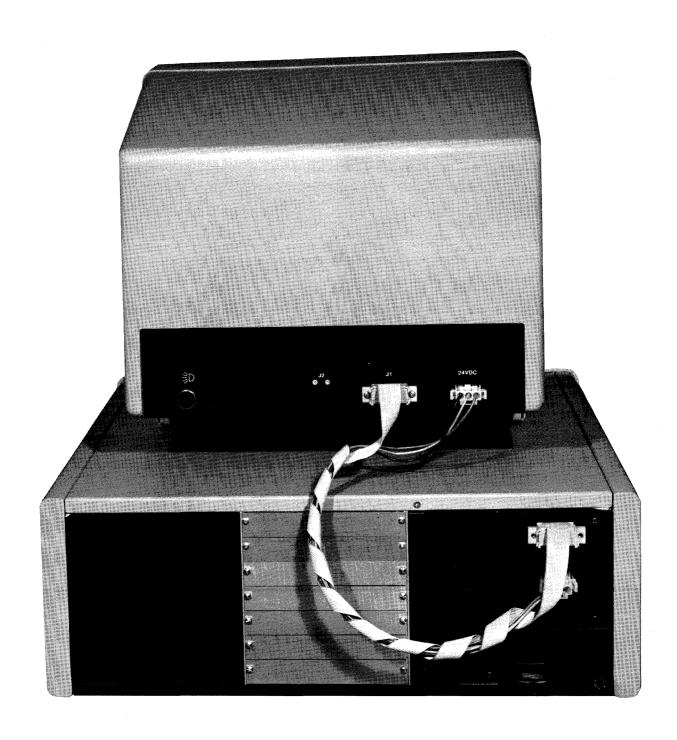
FIGURE 3-1. VME/10 with I/Omodule Expansion Card Cage
