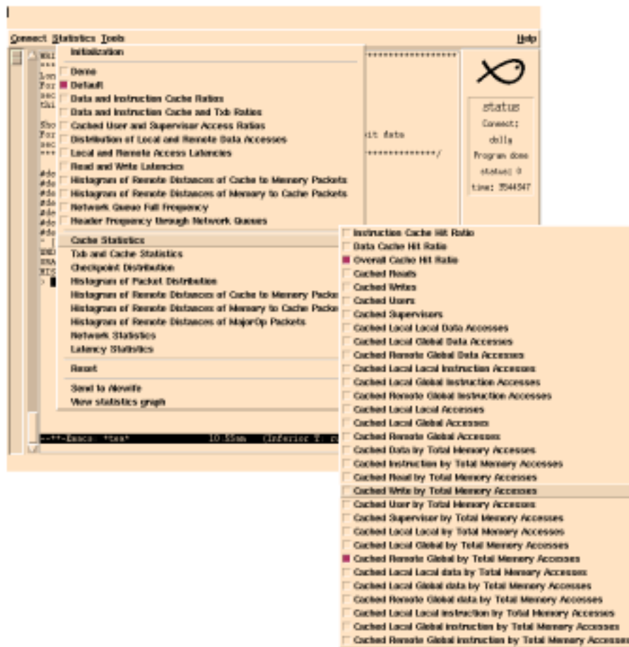
Figure 2.1: The Alewife user interface with pull-down menus for selecting the different statistics to be monitored.
