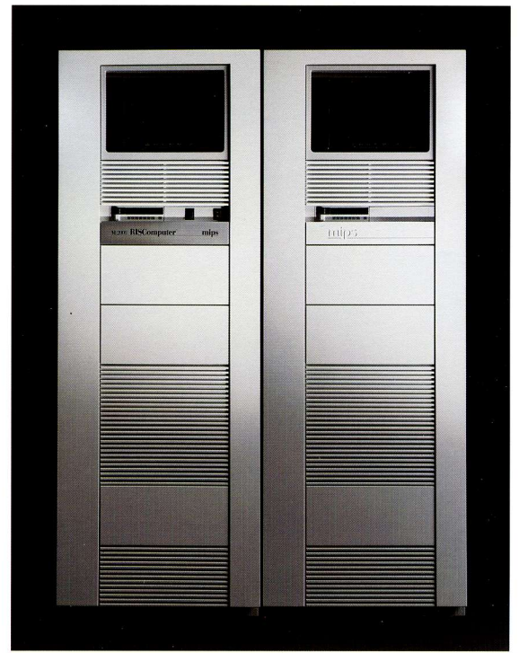
Expansion cabinets may be added to the M/2000 system cabinet for expanded tape and disk capacity.
