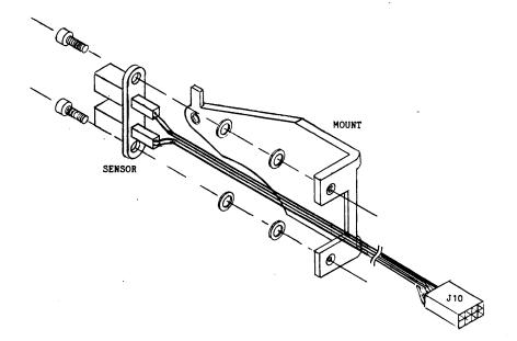
Figure 6-13. Track Zero Sensor
