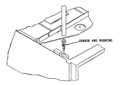
Figure 6-21. Write Protect Sensor Assembly
