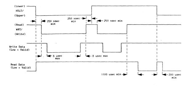
Figure 3-10. Head Select and Read/Write Control Timing
