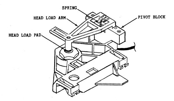
Figure 6-5. Head Load Arm and Pad
