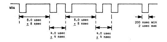
Write Data Timing for MFM @ 250 Kbits/sec
