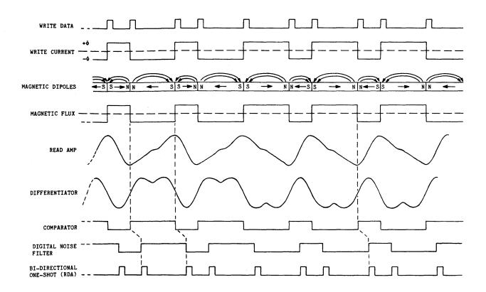
Figure 3-14. Recording Process - Detailed
