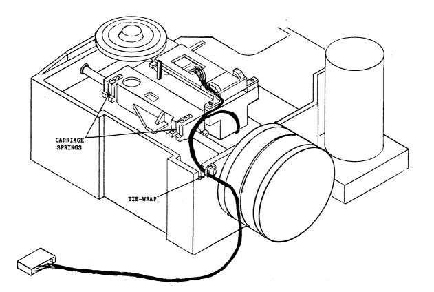
Figure 6-6. Head Carriage Assembly
