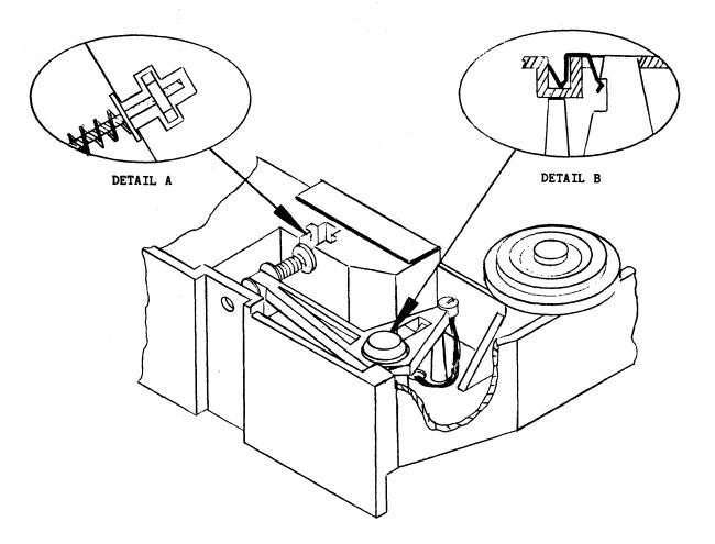
Figure 6-16. Index Sensor Assembly Placement
