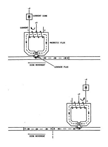
Figure 3-13. The Magnetic Recording Process
