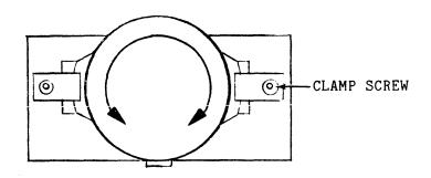
Figure 4-6. Stepper Motor Adjustment
