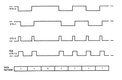
Figure 3-18. Bidirectional One-Shot Timing Diagram
