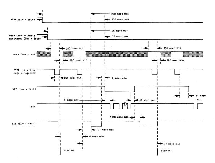
Figure 3-6. Conventional Mode Stepper Timing
