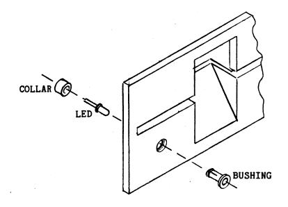
Figure 6-22. In-Use LED Assembly
