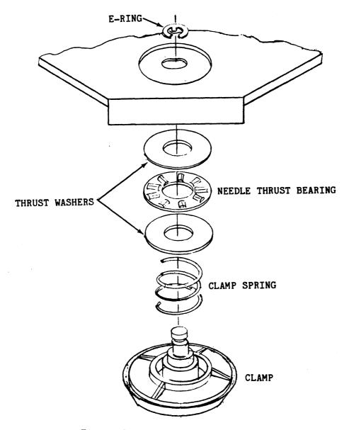
Figure 6-17. Disk Clamp Assembly
