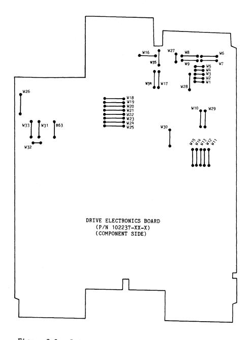
Figure 3-3. Drive Electronics Board Jumper Locations
