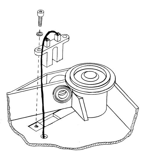
Figure 6-14. Tach Sensor Placement
