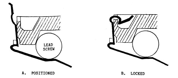
Figure 6-9. Carriage Spring Placement
