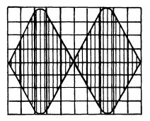
Figure 4-5. Cat's Eye Pattern for Radial Alignment
