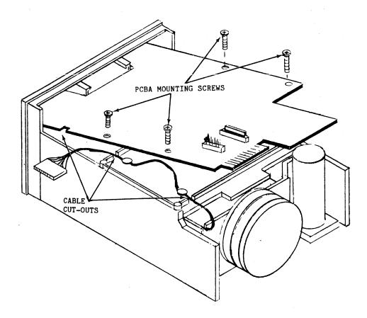
Figure 6-1. PCBA Mounting Details
