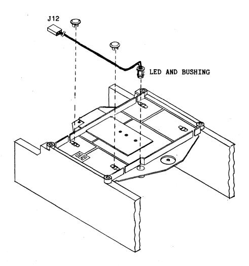
Figure 6-20. Index LED Assembly
