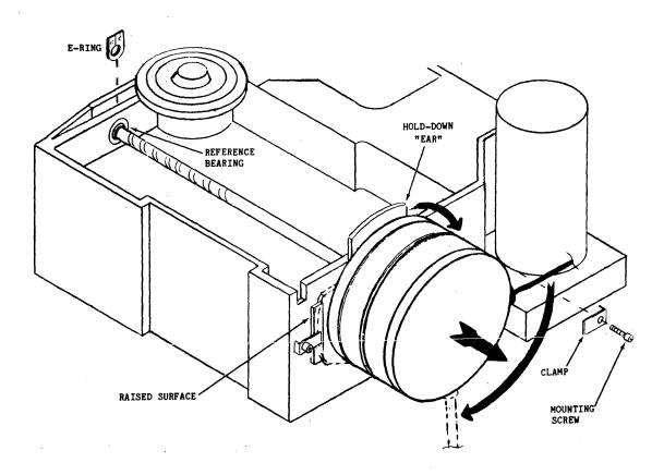
Figure 6-10. Step Motor Assembly
