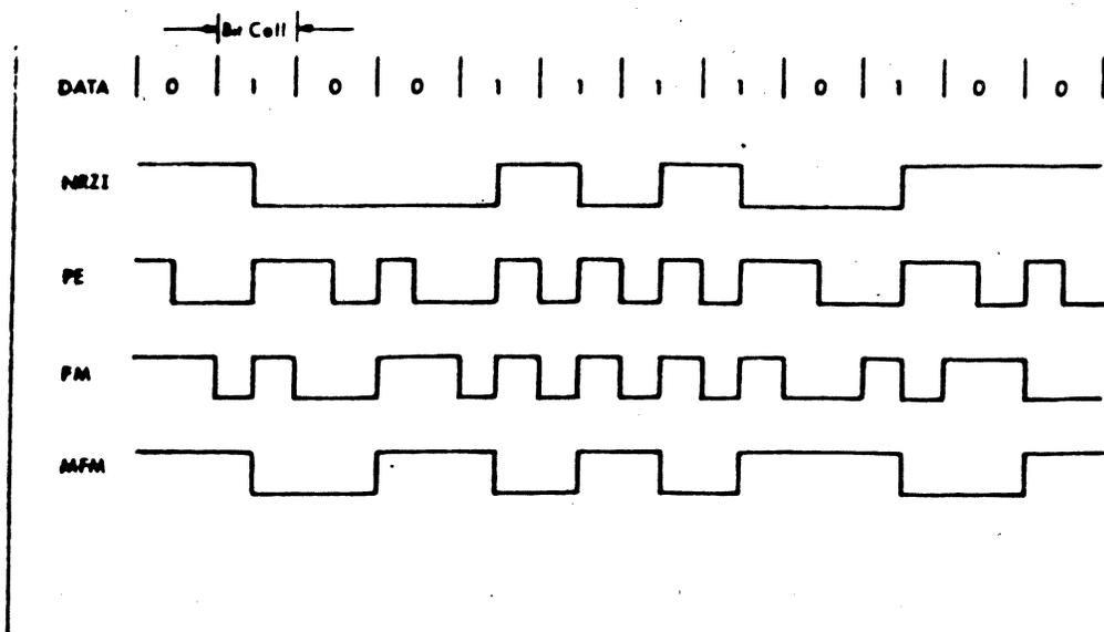
Fig. 1 Conventional waveforms. NRZI is the simplest waveform, but requires a wideband amplifier for processing, since it has a substantial dc component. This and other difficulties are overcome with PE and FM encoding, at the cost of high transition density—up to two transitions per bit. Variations on FM reduce number of transitions, but reintroduce the dc component
