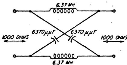
FIG. 17.24. Lattice network for Example 17.5.
