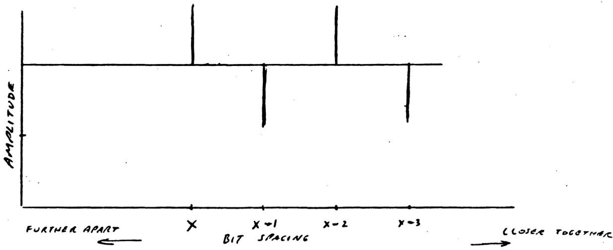
FIG 4-16 A AMPLITUDE VS BIT SPACING, LOW DENSITY
