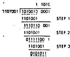
Fig. 1 Manual calculation of  $1 + x^3 + x^5 + x^{10}$  divided by  $1 + x^3 + x^5 + x^6$
