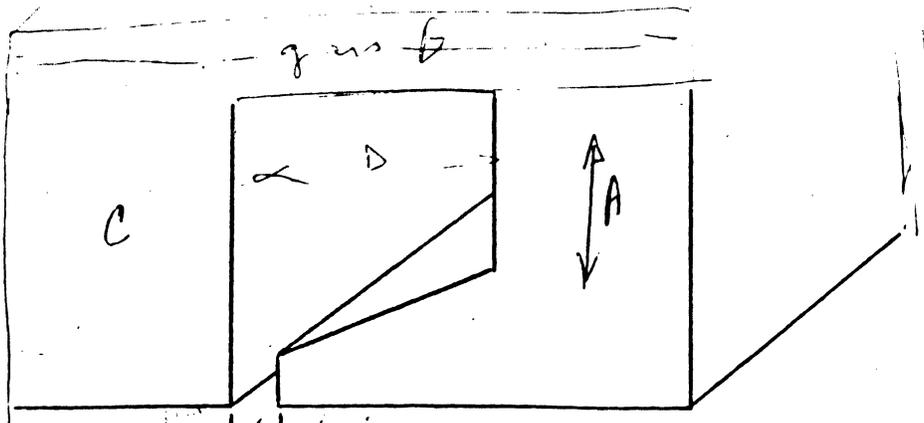
FIG 3.9 CORE AREA REDUCTION AT GAP
