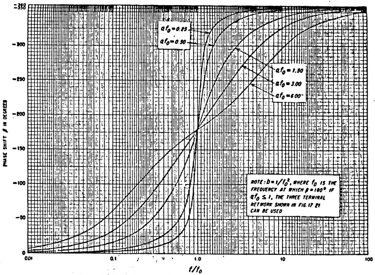
FIG. 17.23. Phase shift in an all-pass filter of the type shown in Fig. 17.21.
