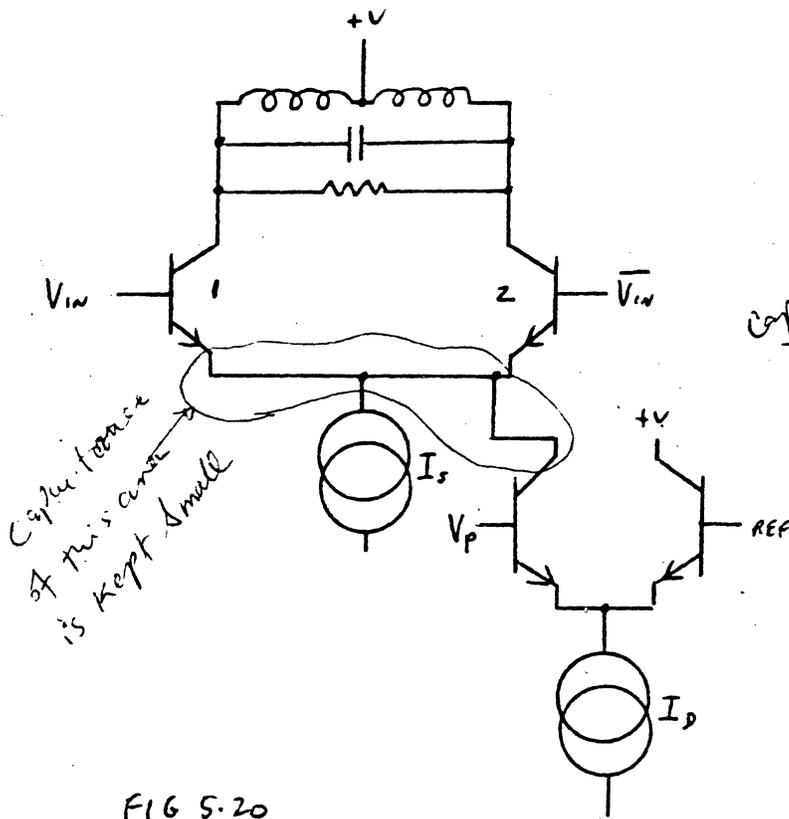
Capacitor voltage of this sense is kept small
