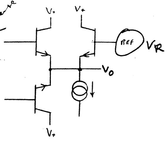
FIG 9.8 BIASED TRANSISTOR CLIPPING FULL WAVE RECTIFIER
