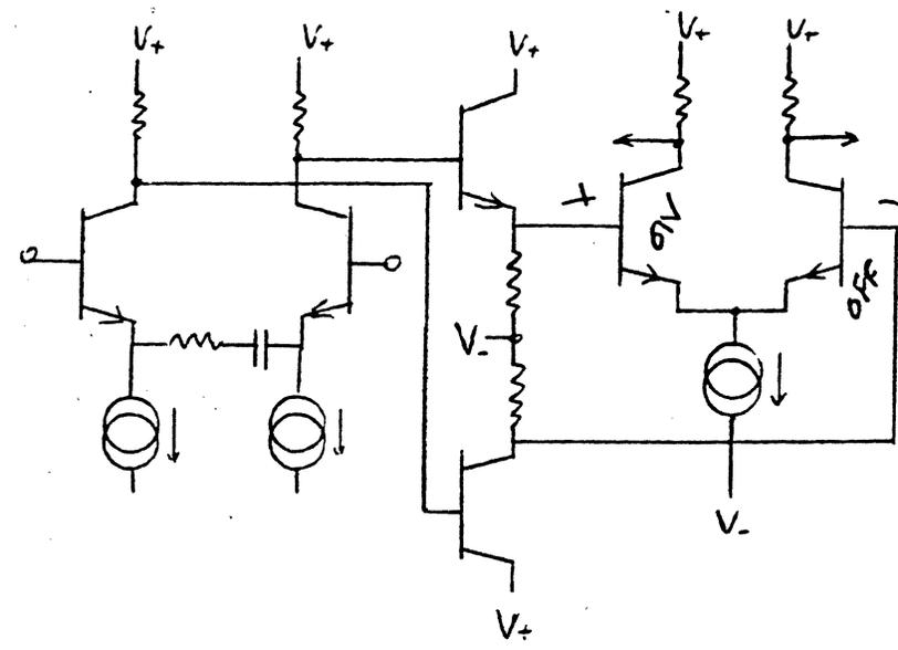
gain:  $\frac{R_L}{R_m + R_E} = \frac{R_L}{R_m + \frac{26}{I_S}}$
