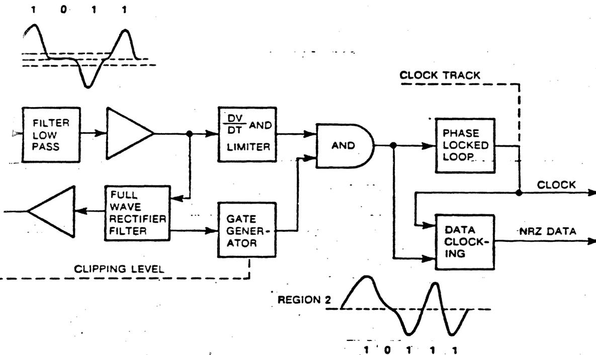
Fig. 2. Traditional Detector, Region 1 used only for high resolution recording
