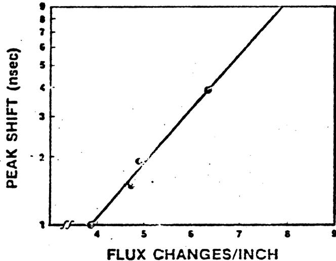
Fig. 3 Peak Shift as a Function of Linear Density for the Experimental System
