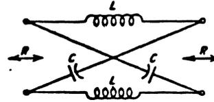
$$L = \frac{R}{2\pi f_0} \quad \text{WHERE } f_0 \text{ IS THE FREQUENCY AT WHICH NETWORK PHASE SHIFT IS } -90^\circ$$
