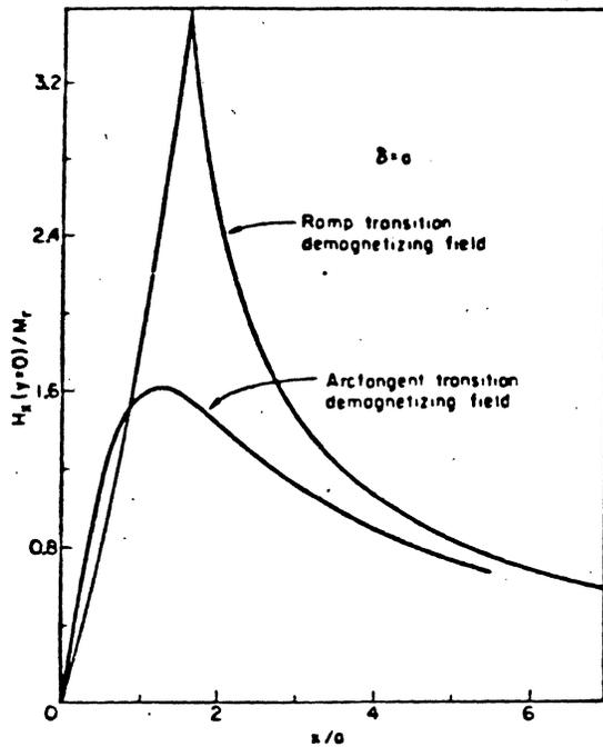
FIG. 1. A comparison of the demagnetizing fields for arctangent and ramp transitions of equal length.
