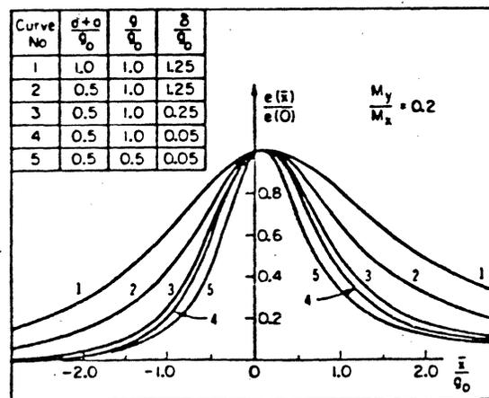
FIG. 3. Readback voltage for several values of  $d+a$ ,  $\delta$ , and  $g$ ; and for  $M_y/M_x = 0.2$ . All dimensions are normalized to an arbitrary gap length  $g_0$ .
