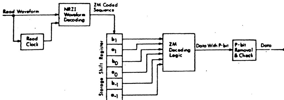
Fig. 5 ZM decoder. Data bits are defined in terms of pairs of code bits, taking into account preceding and following pair along with current pair. Hence the key element is a 6-bit shift register that shifts two bits at a time and feeds code information to decoding logic
