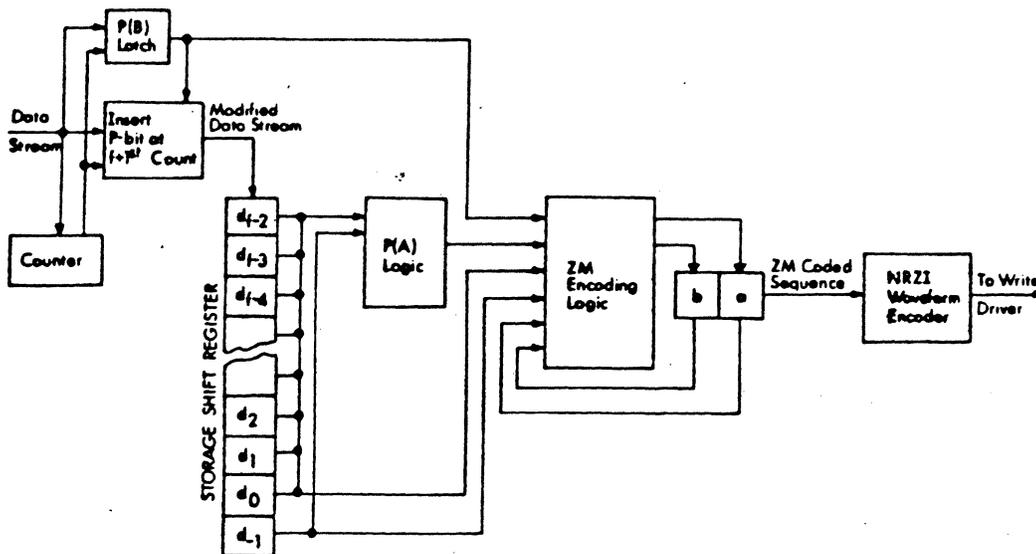
Fig. 4 ZM encoder. Principal feature is a shift register from which data bits are fed to encoding logic, which is straightforward implementation of equations in text
