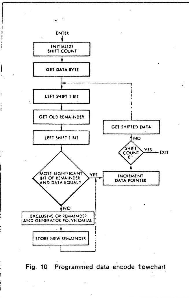
Fig. 10 Programmed data encode flowchart
