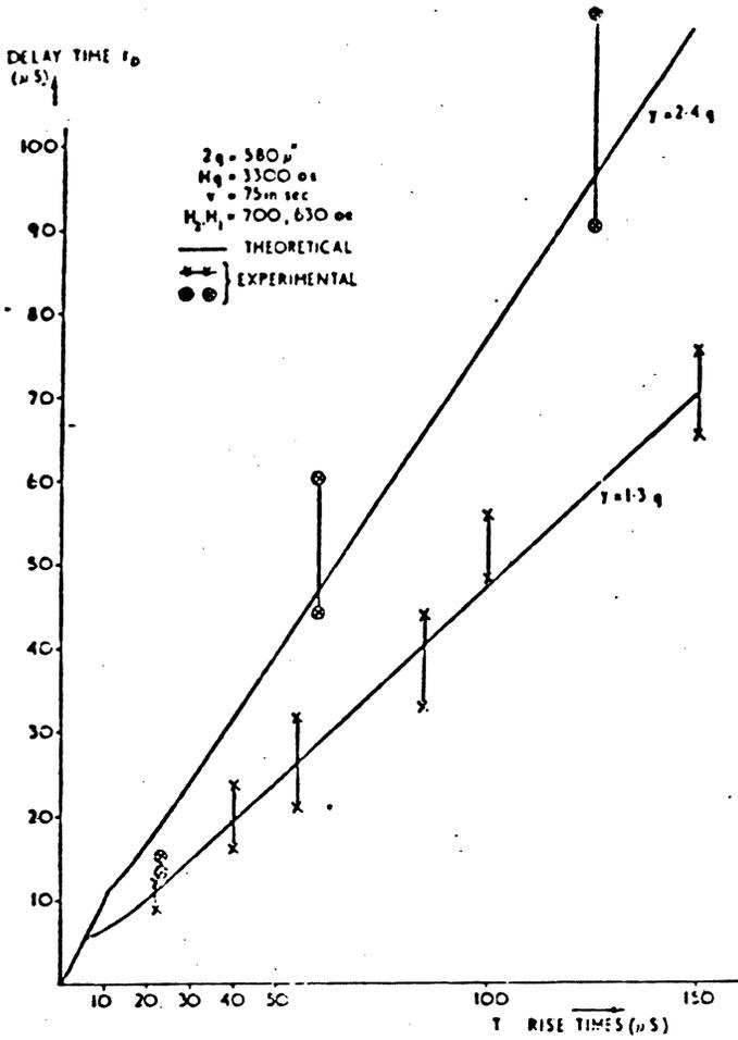
Fig. 3. Comparison of experimental with theoretical results for delay time versus rise time.
