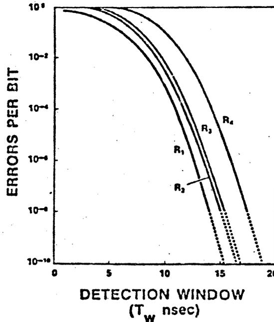
Fig. 1 MVFO Curves of Errors per Bit vs.  $1/2$  Detection Window at Four Radii
