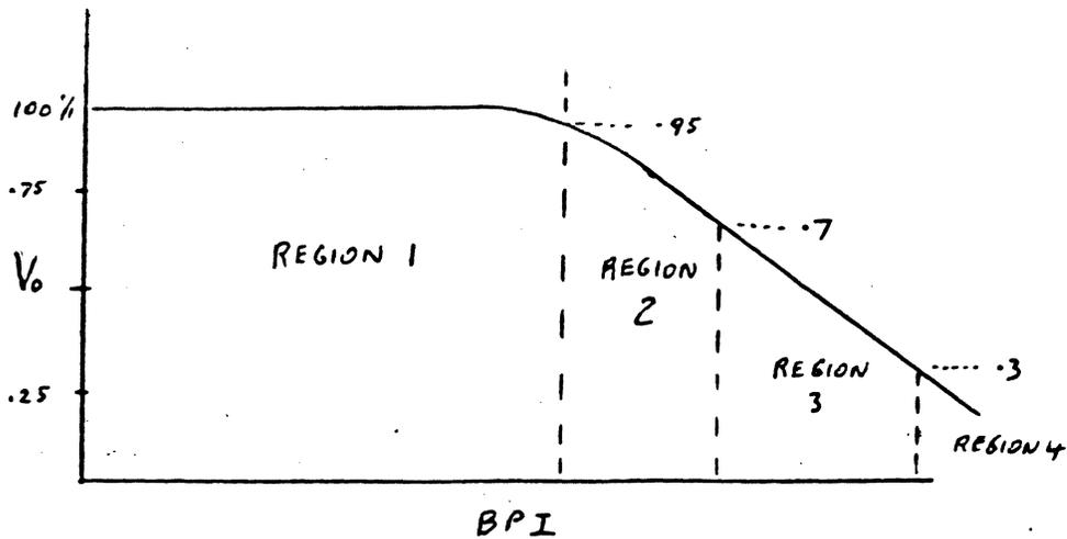
FIG 9.1 BIT DENSITY CURVE, DETECTOR REGIONS DIVISIONS NOT FIRM.
