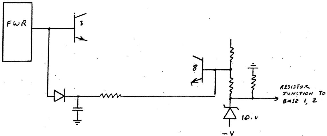
FIG 10.2 SIGNAL AMPLITUDE CONTROL OF THE CLIPPING LEVEL. (SEE FIG 9.19 FOR THE REST OF THE CIRCUIT)
