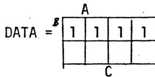
The decode is clocks =  $\bar{A} \bar{B}$ , data = B. Therefore, we can delete the C FF or "future" and deal only with the past and present. The sequence is shift, clock, data, shift. The implementation is given in Fig. 12.20. Note that the set up and timing paths prevent unequal logic delays from hurting bit timing. To add precompensation, we require a four level truth table (Table 12.10). We will shift-data-clock-shift.
