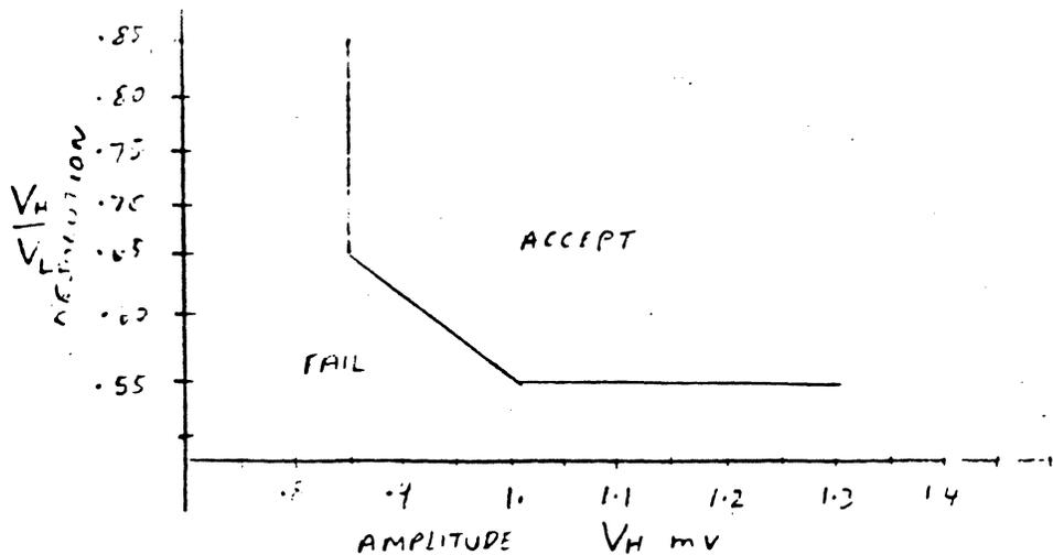
Fig. 13.4 Acceptable Amplitude and Resolution Combinations
