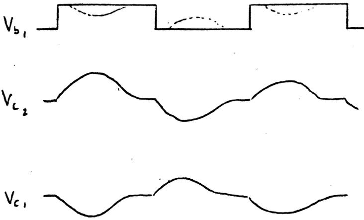
FIG 5.18 MILLER FEEDBACK FROM HEAD TRANSIENT
