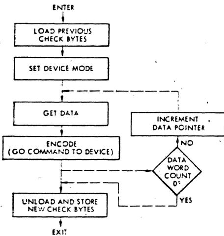
Fig. 9 Device data encode flowchart
