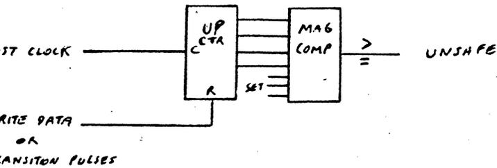
FIG 8.28 CODE RELATED TRANSITIONS UNSAFE CIRCUIT
