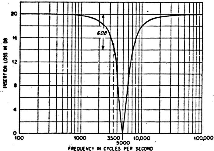
FIG. 17.18. Insertion-loss characteristics of network shown in Fig. 17.17.
