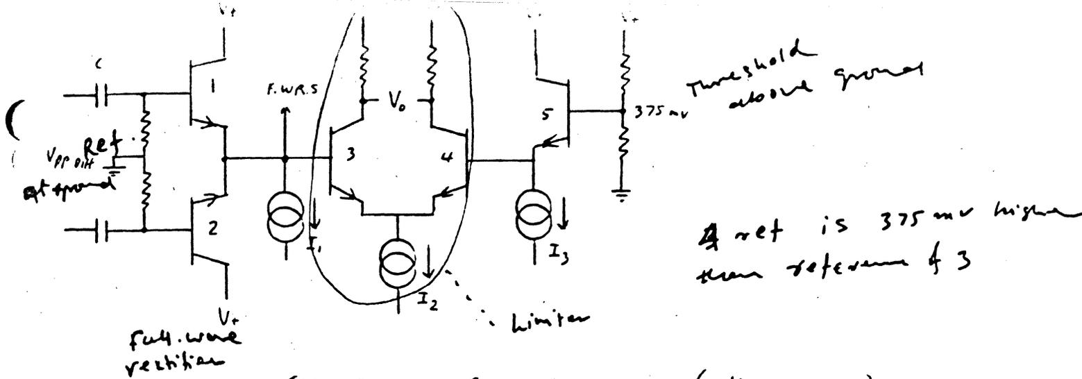
FIG 9.10 GATE GENERATOR (15% CLIPPING)
