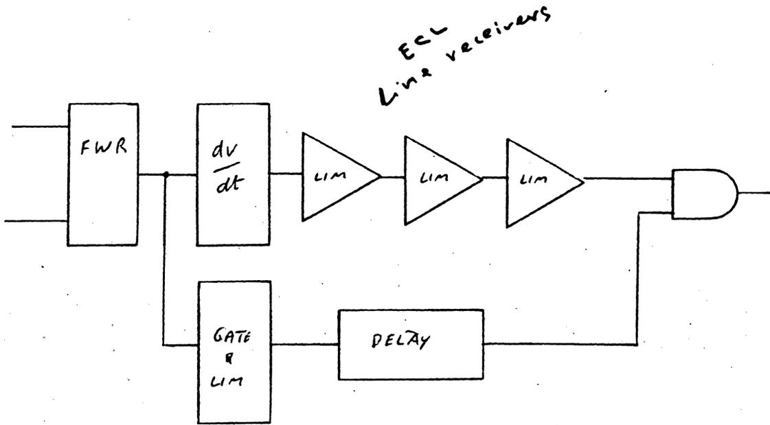
FIG 9-18 BLOCK DIAGRAM SHOWING DELAY USED TO CENTER LEADING EDGE OF DATA IN GATE (AT MINIMUM INPUT AMPLITUDE)
