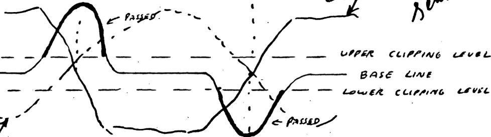
FIG 9.2 REGION 1 HEAD SIGNAL SHOWING CLIPPING LEVELS FOR NOISE REDUCED AMPLITUDE SENSITIVITY
