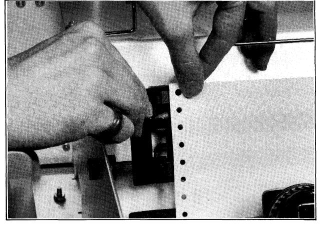
7. Lay the paper back over the top of the tractors (open). The front of the paper should face you (Figure 3-6).
