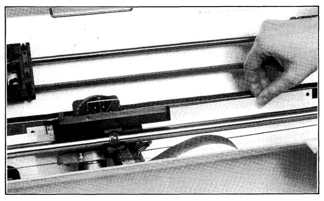
Figure 3-5. Inserting Paper
