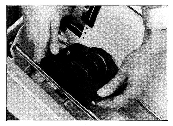
Figure 4-2. Removing The Old Cartridge
