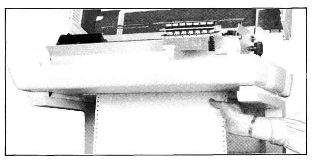
Figure 3-4. Inserting Paper From Below
