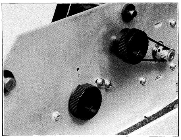
Figure 3-11. Adjusting for Forms of Different Thickness — Lower Knob
