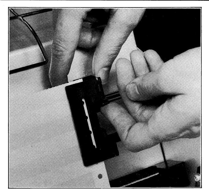
Figure 3-8. Adjusting for Paper Width
