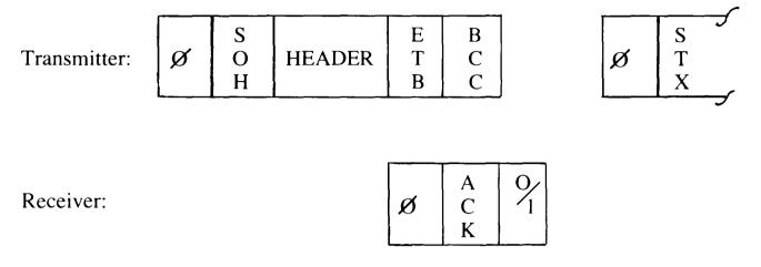
Figure 2. Header Terminated by ETB for Error Checking Purposes
