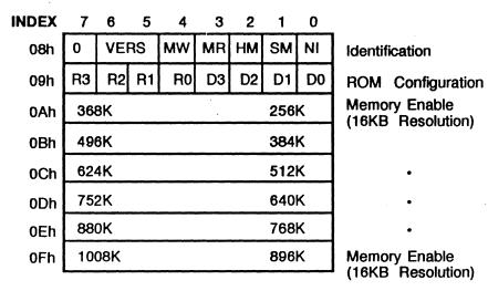
Figure 2-27. Control and Address Space Map Registers
