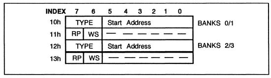
Figure 2-28. DRAM Configuration/Timing Register Summary
