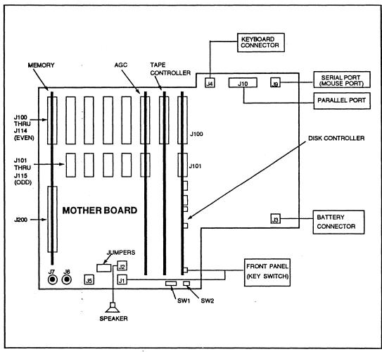
Figure 2-78. Motherboard Component Locations
