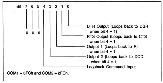
Figure 2-75. Modem Control Register
