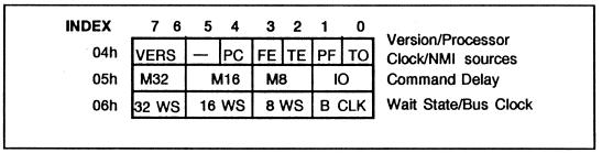
Figure 2-25. 82C301 Bus Controller Configuration Registers.
