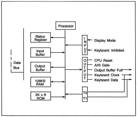
Figure 4-1. Keyboard Controller Block Diagram.
