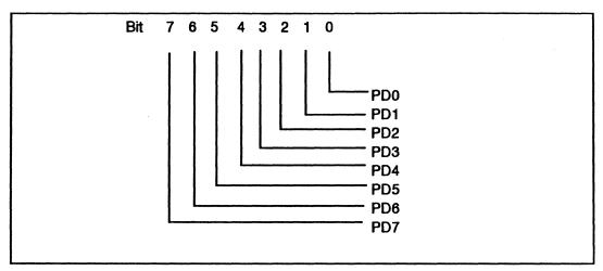
Figure 2-68. Parallel Port Data Register
