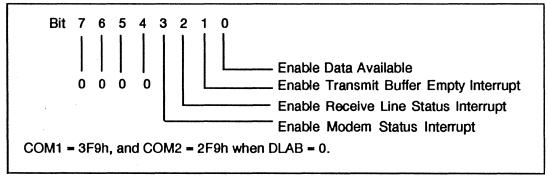
Figure 2-72. Interrupt Enable Register
