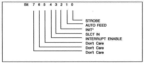
Figure 2-67. Parallel Port Control Register
