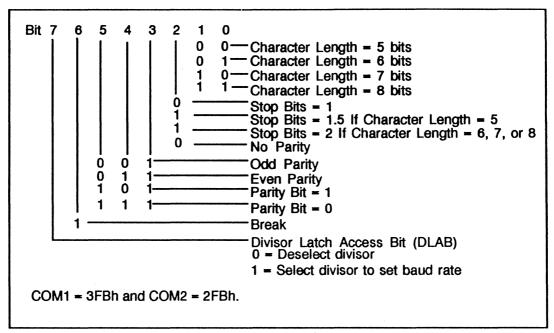
Figure 2-74. Line Control Register
