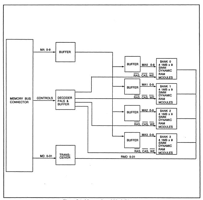
Figure 5-1. Memory Board Block Diagram
