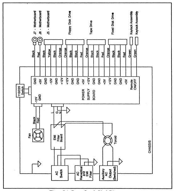
Figure 7-1. Power Supply Block Diagram
