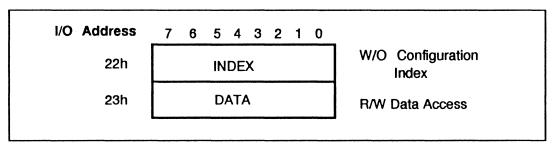
Figure 2-21. Configuration Register Access Ports
