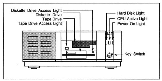
Figure 1-1. Typical System Unit
