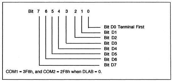
Figure 2-71. Transmit/Receive Buffer Register
