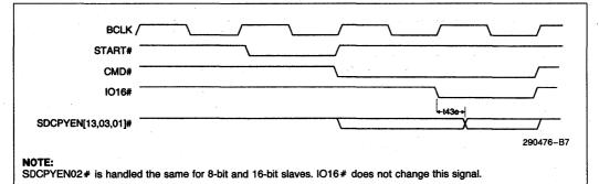
Figure 12-24. EISA or DMA Master Read from 16-Bit ISA I/O
