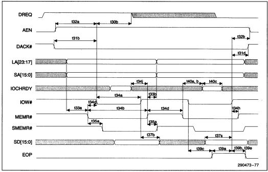
Figure 6-14. DMA Compatible Timing (Memory Read)
