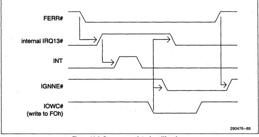
Figure 11-2. Coprocessor Interface Waveform
