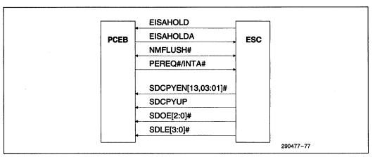
Figure 10-1. PCEB/ESC Interface Signals
