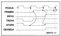
Figure 5-13. Target-Initiated Termination - Disconnect
