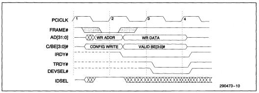
Figure 5-6. Configuration Write Cycle
