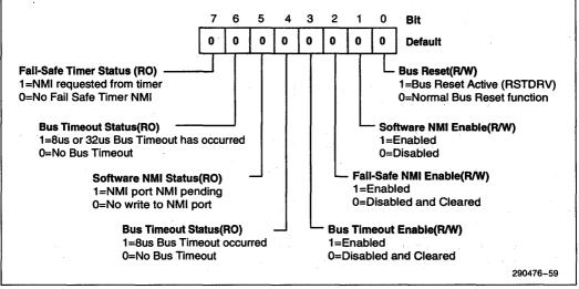
Figure 3-57. NMI Extended Status and Control Register
