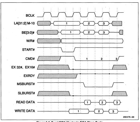
Figure 5-3. Burst EISA Master to EISA Slave Cycle
