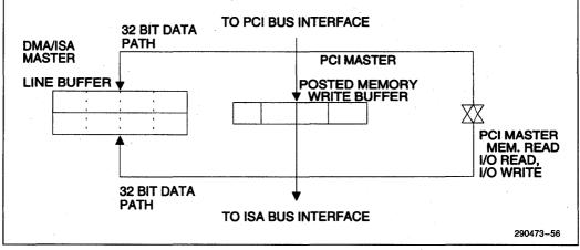
Figure 5-52. SIO Buffer Diagram
