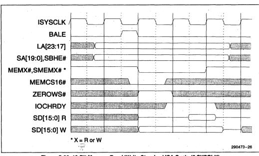
Figure 5-22. 16-Bit Memory Read/Write Standard ISA Cycle (3 SYSCLK)
