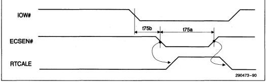
Figure 6-27. Real Time Clock Timing (RTCALE Generation)
