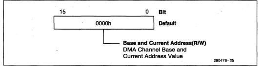
Figure 3-23. DMA Base and Current Address Register
