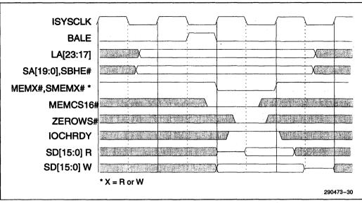
Figure 5-26. 16-Bit Memory Read/Write Compressed Cycle (2 SYSCLK)
