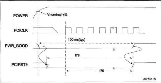
Figure 6-30. PCIRST # A.C. Timing Wave Form
