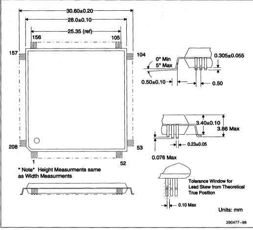
Figure 12-2. 208 Pin Plastic Quad Flat Pack (PQFP) Dimensions
