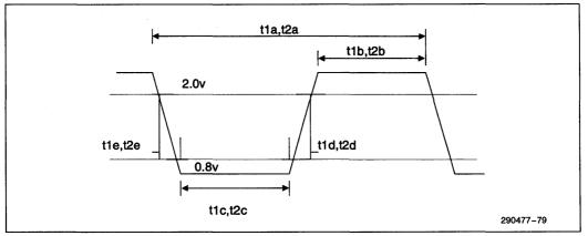
Figure 11-1. PCICLK, BCLK Timing
