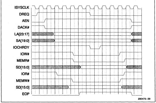
Figure 5-35. Compatible DMA Transfer (with 1 Wait State)
