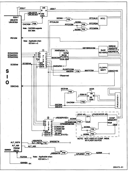
Figure 5-57. Utility Bus External Support Logic
