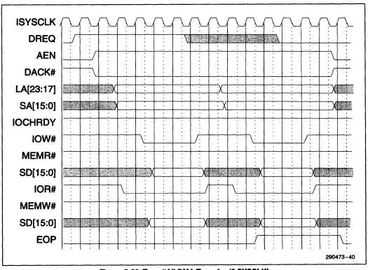
Figure 5-36. Type "A" DMA Transfer (6 SYSCLK)
