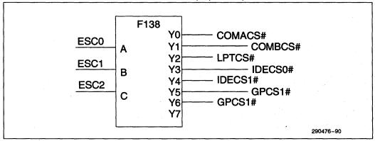
Figure 11-3. Encoded Chip Select Decoder Logic
