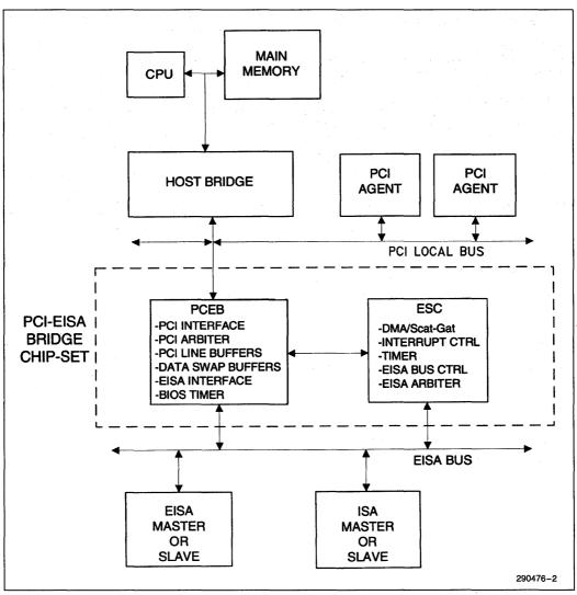
Figure 1-1. PCI-EISA Chip Set System Block Diagram
