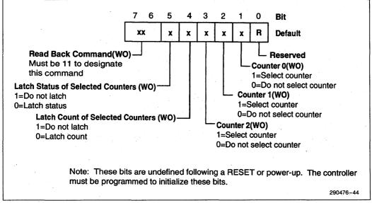
Figure 3-42. Timer Read Back Command Register
