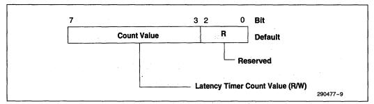
Figure 3-6. Master Latency Timer Register
