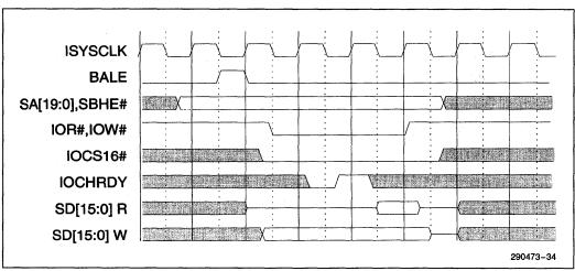
Figure 5-30. 16-Bit I/O Read/Write Extended ISA Cycle (4 SYSCLK shown)
