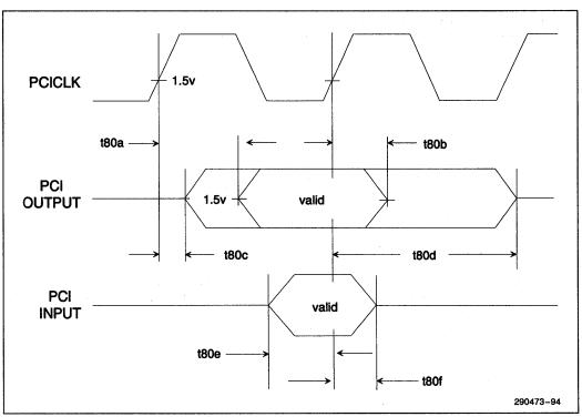
Figure 6-31. Shared Signals A.C. Timing Wave Form
