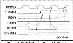
Figure 5-12. SIO Master, Target-Initiated Termination - Abort
