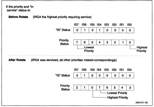
Figure 5-55. Automatic Rotation Mode Example
