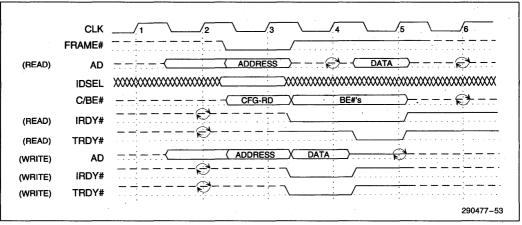
Figure 5-5. Configuration Cycle
