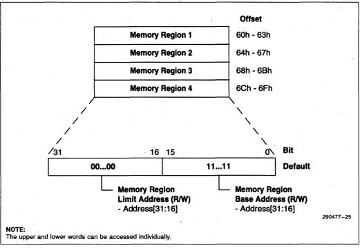
Figure 3-22. EISA-to-PCI Memory Region Address Register
