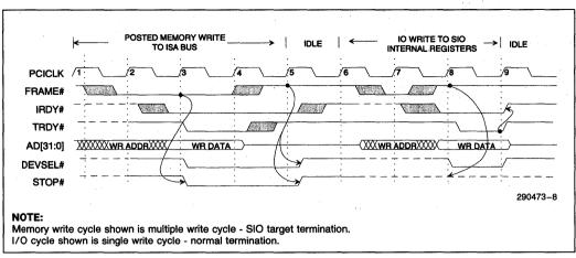
Figure 5-4. PCI Write to SIO - Posted Write, Register Write (SIO as Slave)
