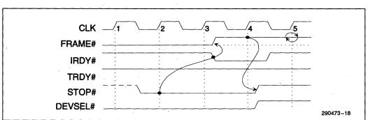
Figure 5-14. Target-initiated Termination - Retry
