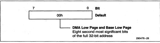
Figure 3-26. DMA Memory Low Page and Base Low Page Register
