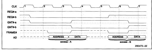
Figure 5-18. Basic PCI Arbitration
