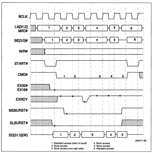
Figure 7-2. EISA Memory Write Burst Cycle
