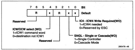
Figure 3-46. Initialization Command Word 1 Register
