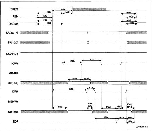
Figure 6-18. DMA Type "B" Timing
