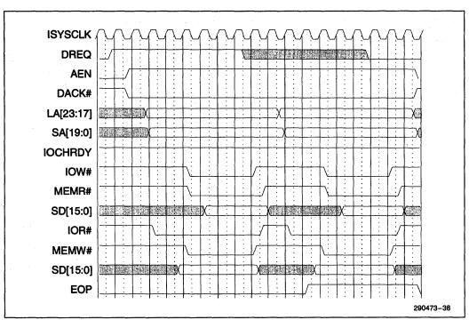
Figure 5-34. Compatible DMA Transfer (8 SYSCLK)
