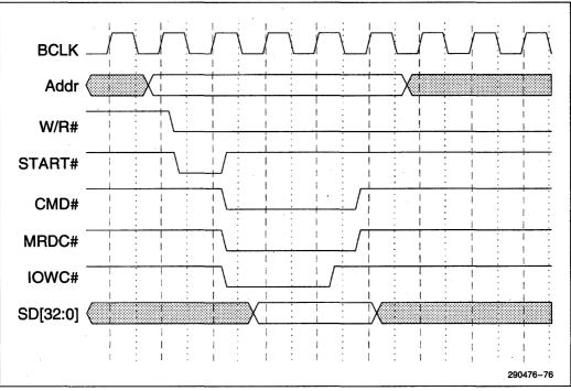
Figure 6-4a. Type "B" DMA Read Transfer (4 BCLKS)
