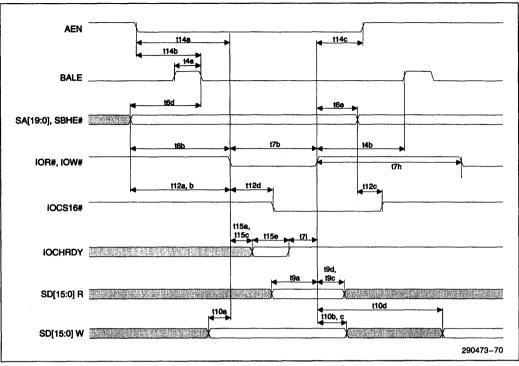
Figure 6-7. 16-Bit I/O Slave Timing (SIO as Master)
