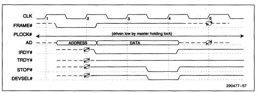
Figure 5-9. Access to Locked Target with PLOCK# Asserted During Address Phase
