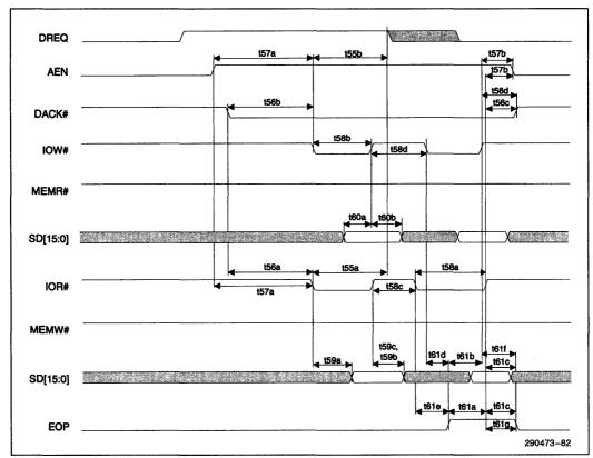
Figure 6-19. DMA Type "F" Timing
