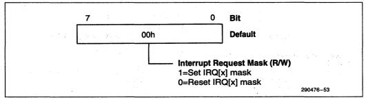
Figure 3-51. Operation Control Word 1 Register
