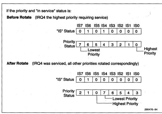
Figure 9-3. Automatic Rotation Mode Example
