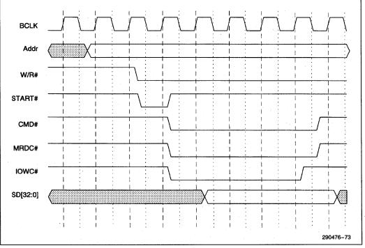
Figure 6-2a. Compatible DMA Read Transfer (8 BCLKs)
