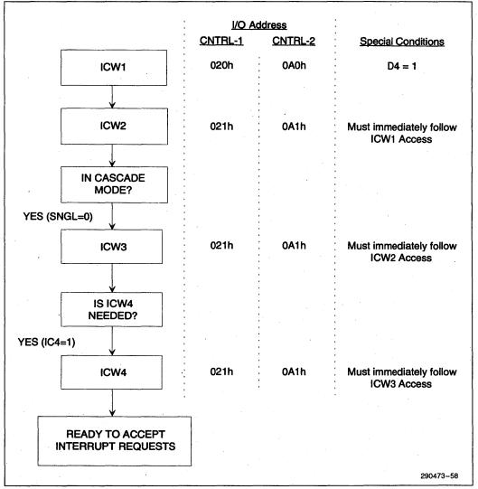
Figure 5-54. Initialization Sequence for SIO Initialization Command Words (ICWs)
