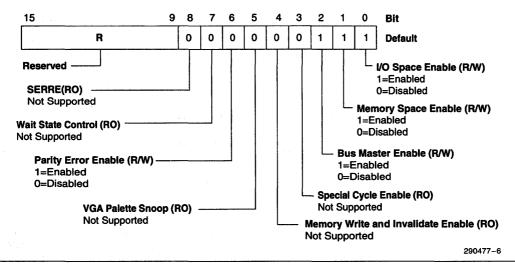
Figure 3-3. PCI Command Register
