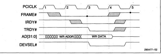
Figure 5-4. Fastest PCI Write to PCEB
