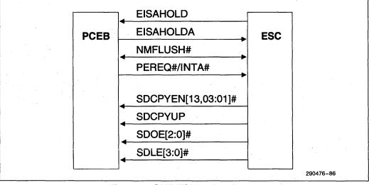
Figure 10-1. PCEB/ESC Interface Signals
