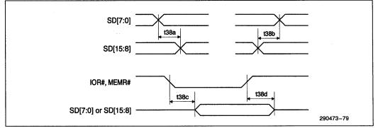
Figure 6-16. DMA Compatible Timing (Data Swap)
