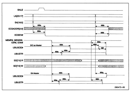
Figure 6-22. PCI and ISA Master Access to Utility Bus Timing
