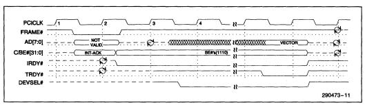
Figure 5-7. Interrupt Acknowledge Cycle
