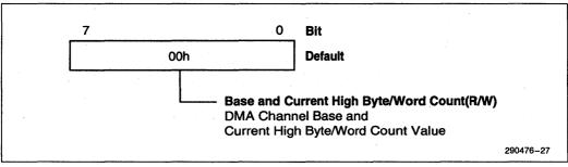
Figure 3-25. DMA Base and Current High Byte/Word Count Register
