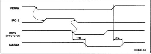
Figure 6-25. Coprocessor Error Support Timing
