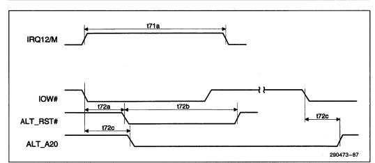
Figure 6-24. Mouse and Port 92 Timing
