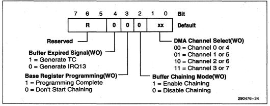
Figure 3-32. Chaining Mode Register
