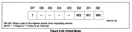
This mode is useful if there is a routine command common to several levels so that the INTA# sequence is not needed (saves ROM space).
