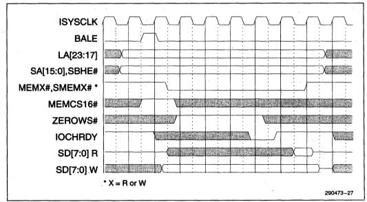
Figure 5-23. 8-Bit Memory Read/Write Extended Cycle (7 SYSCLK shown)
