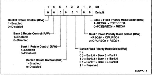
Figure 3-9. PCI Arbiter Priority Control Register
