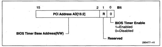
Figure 3-24. BIOS Timer Base Address Register
