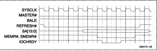
Figure 5-44. Bus Master-initiated Extended Refresh Cycle
