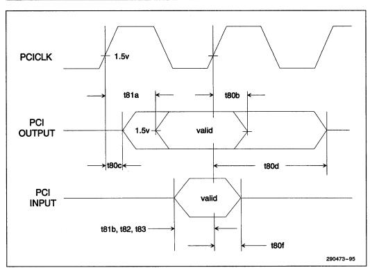
Figure 6-32. Sideband Signals A.C. Timing Wave Form
