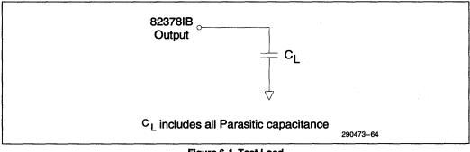
Figure 6-1. Test Load
