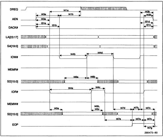
Figure 6-17. DMA Type "A" Timing
