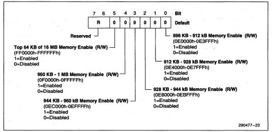
Figure 3-20. EISA Address Decoder Control Extension Register
