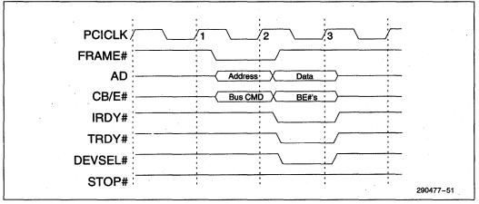
Figure 5-3. PCEB Write to PCI Memory
