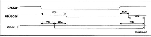
Figure 6-23. DMA Access to Utility Bus Timing
