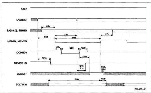
Figure 6-8. ISA Master Accessing PCI Memory Timing
