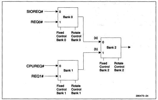
Figure 5-20. Arbiter Configuration Diagram
