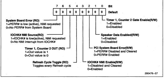
Figure 3-55. NMI Status and Control Register
