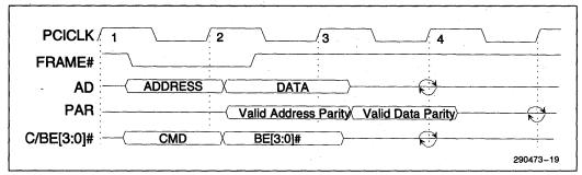
Figure 5-15. SIO Master Write Cycle Parity Operation
