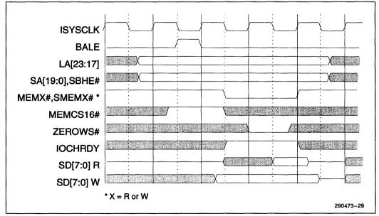
Figure 5-25. 8-Bit Memory Read/Write Compressed Cycle (3 SYSCLK)
