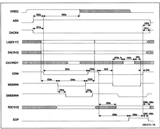
Figure 6-15. DMA Compatible Timing (Memory Write)
