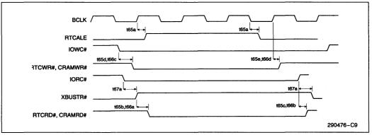
Figure 12-36. Real Time Clock and Configuration RAM Signals
