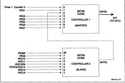
Figure 5-53. Block Diagram Of The Interrupt Controller
