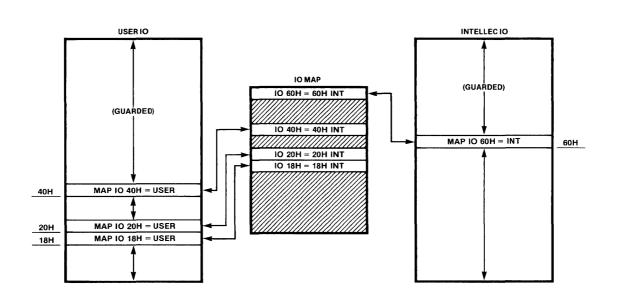
Figure 5-7. IO Port Segments Mapped to User and Intellec 463-23
