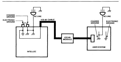
Figure 2-3. System Grounding for Intellec Series I 463-11
