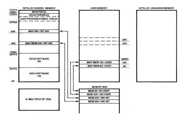
Figure 5-5. Mapping Into User and Shared Intellec Memory 463-21
