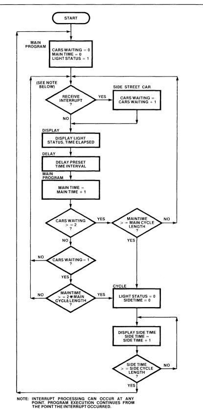
Figure 3-1. Traffic Light Controller Program Flow Chart
