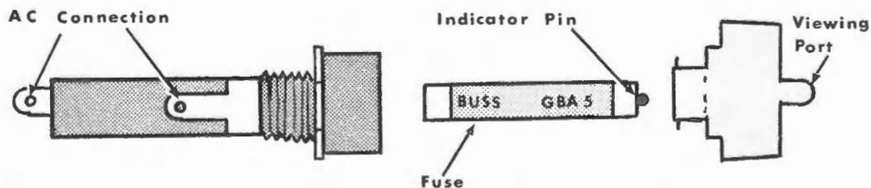
Figure 1. Indicating Fuse, Install Pin Toward Viewing Port
