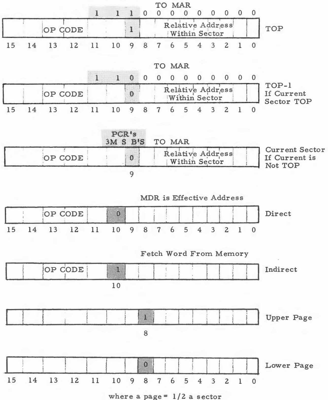
Figure 4-4. Effective Address Calculation Illustrated
