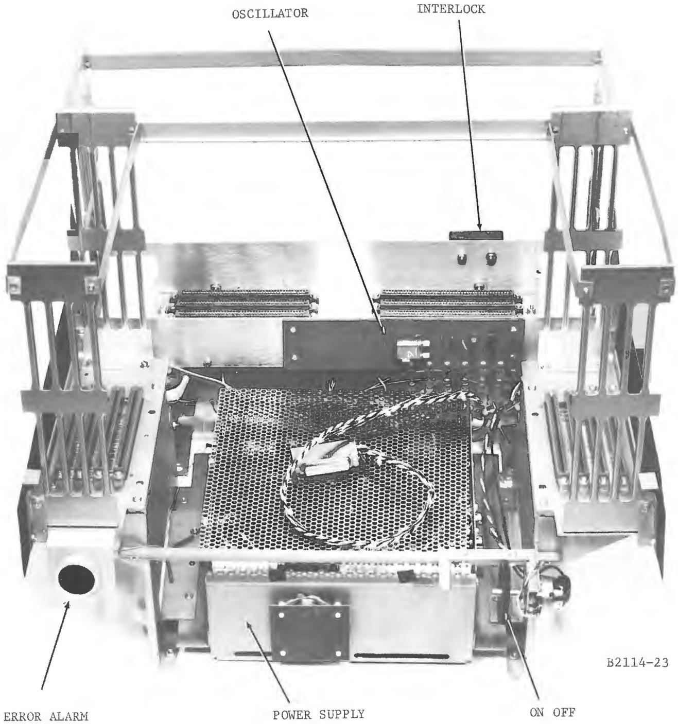
Figure 2-5. TPU Wired Chassis with Power Supply
