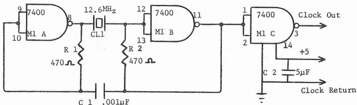
Figure 5-16. Line Lock Oscillator Schematic
