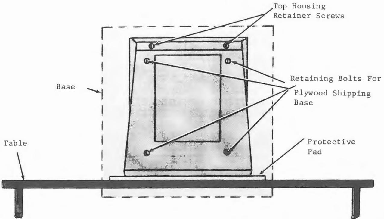
Figure 2-2. Removal of Plywood Base
