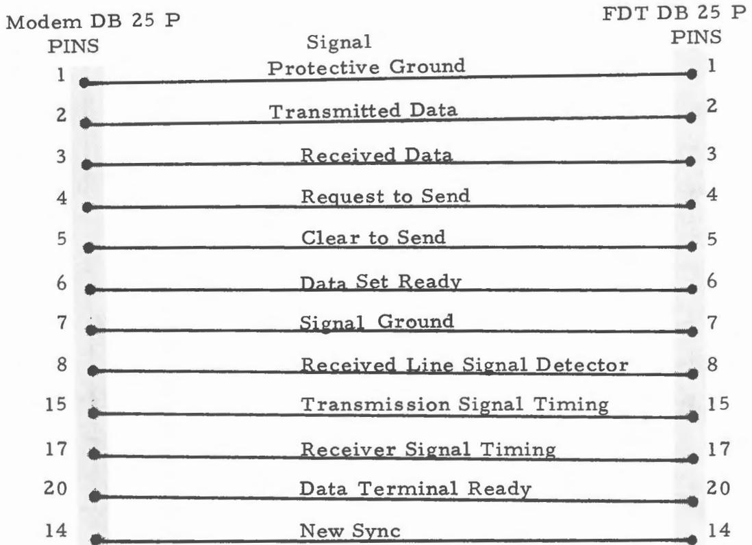
Modem to synchronous or asynchronous controllers full duplex operation.
