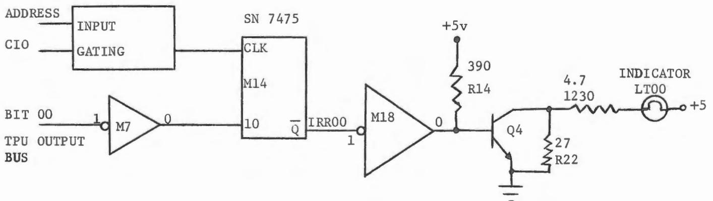
Figure 6-4. Typical Keyboard Lamp Driver Circuit (One Bit Shown)
