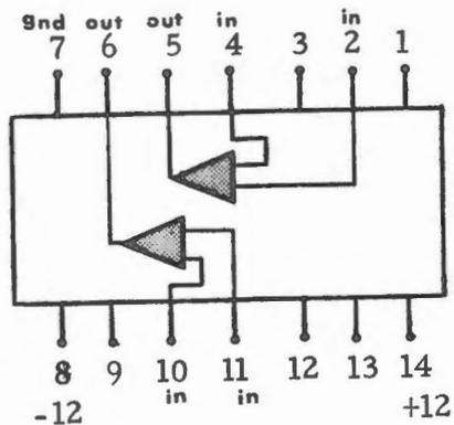
Figure 2. Connection Diagram
