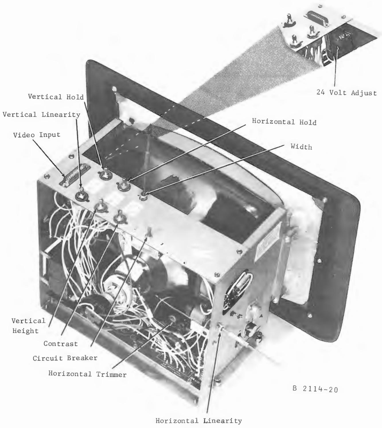
Figure 7-6. T. V. Monitor Adjustments
