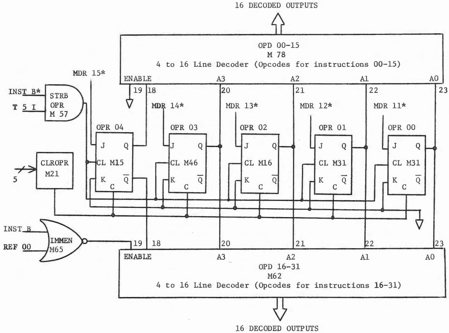
Figure 5-6. Detailed Block Diagram of Instruction Register and Decoder
