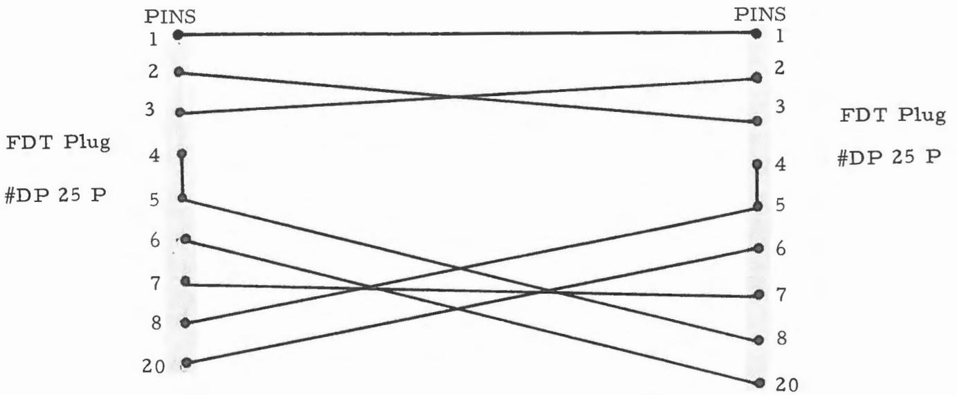
Freestanding Display Terminal cabling diagram. Reference drawing number 011-10-07.
