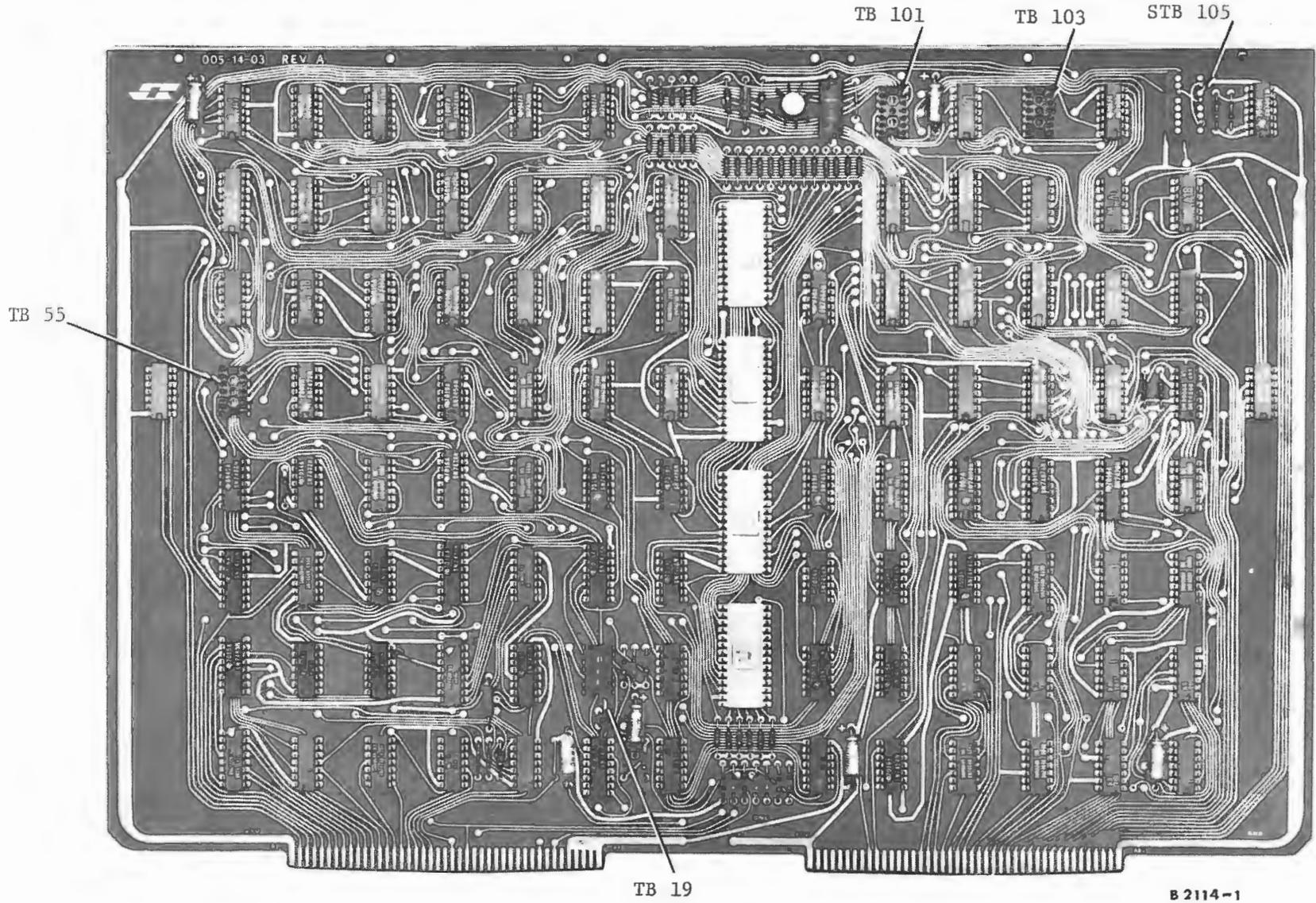
Figure 5-12. Refresh Module Timing Unit
