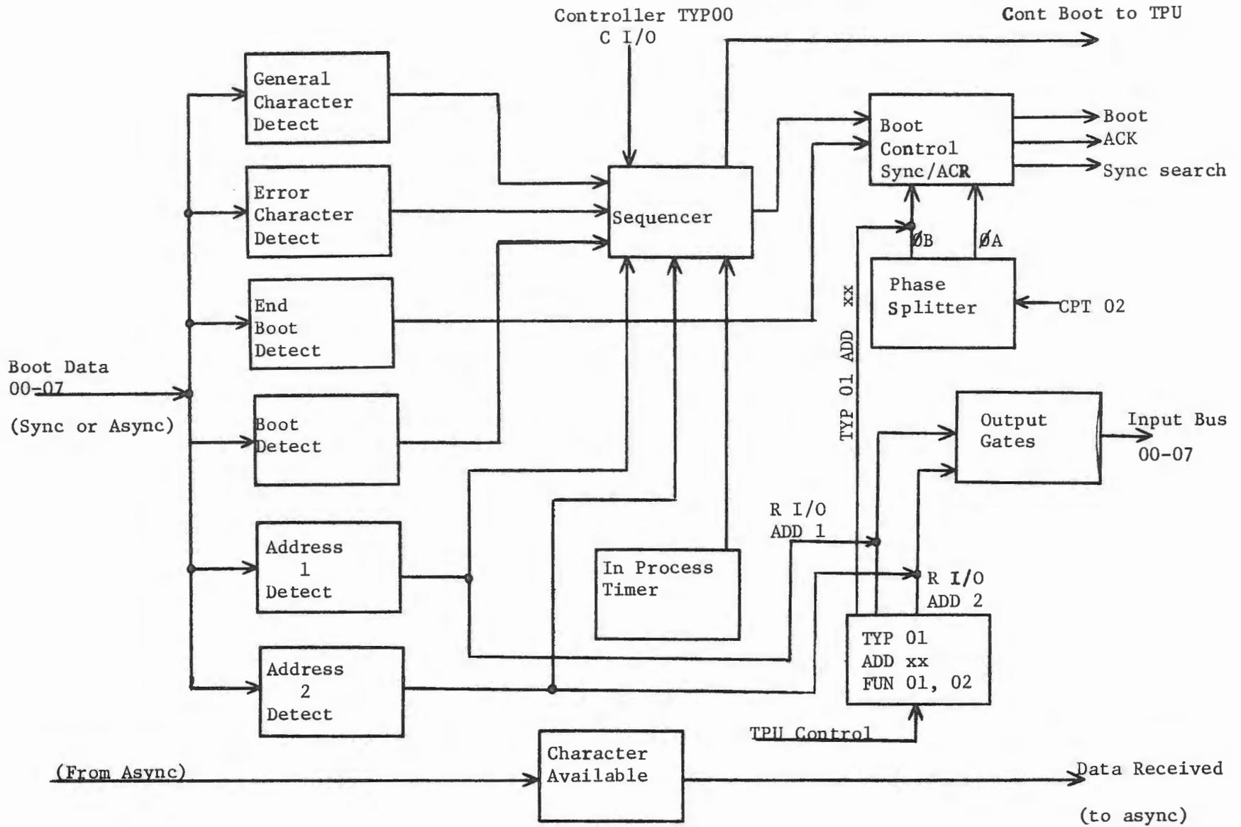
Figure 6-11. Simplified Diagram Boot Controller
