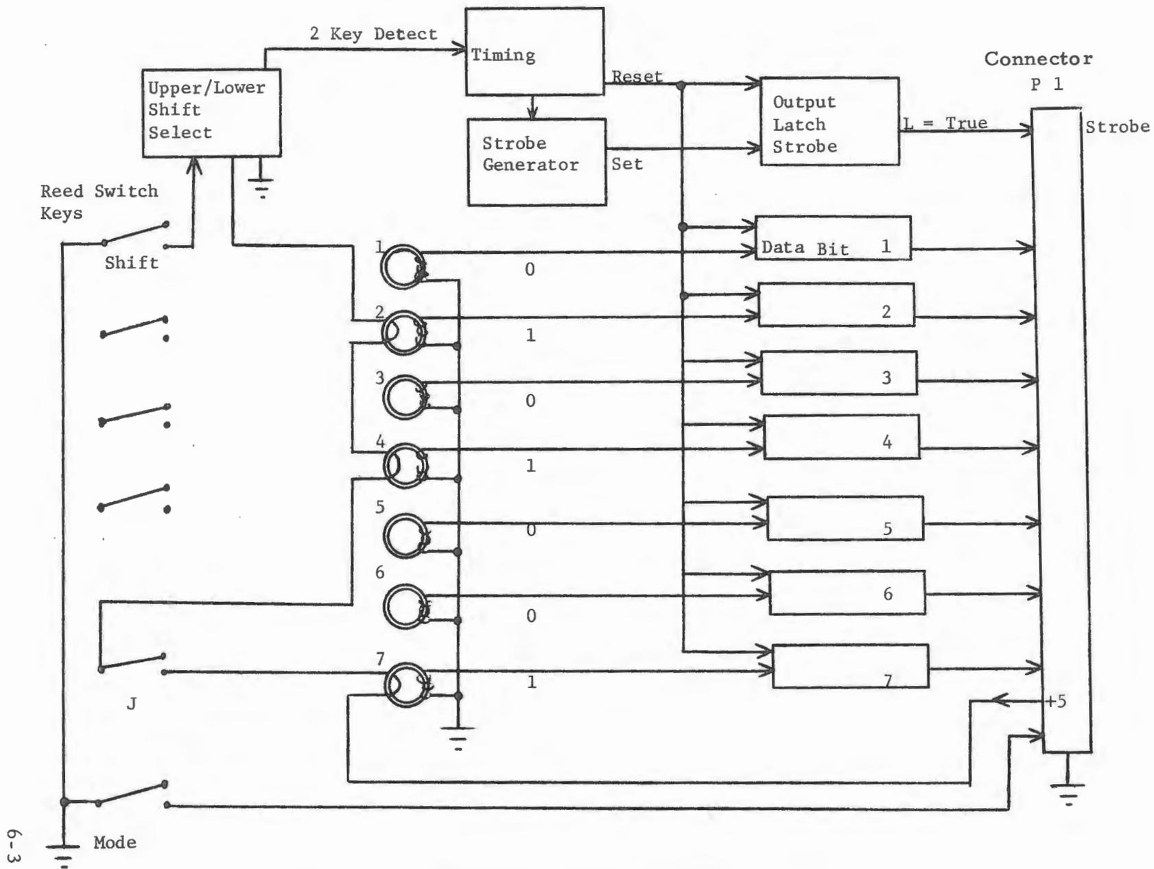
Figure 6-2. Simplified Keyboard Block Diagram Current Path Illustrated for J Key
