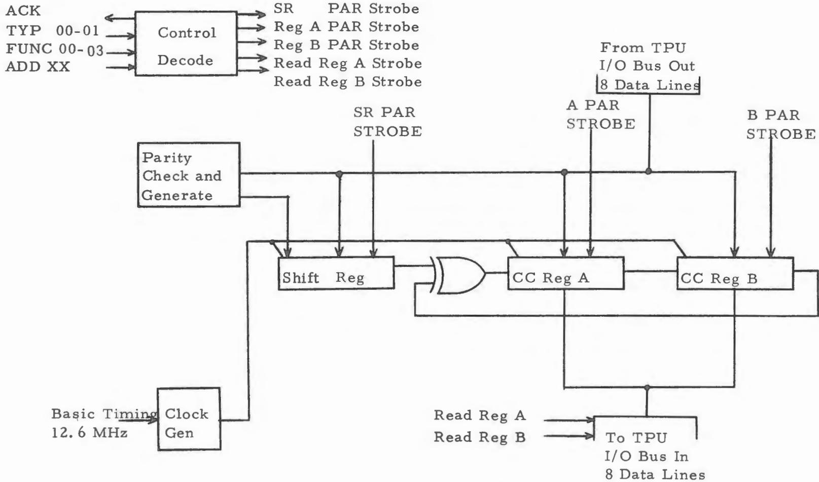
Figure 2. Block Diagram, Cyclic Check Controller
