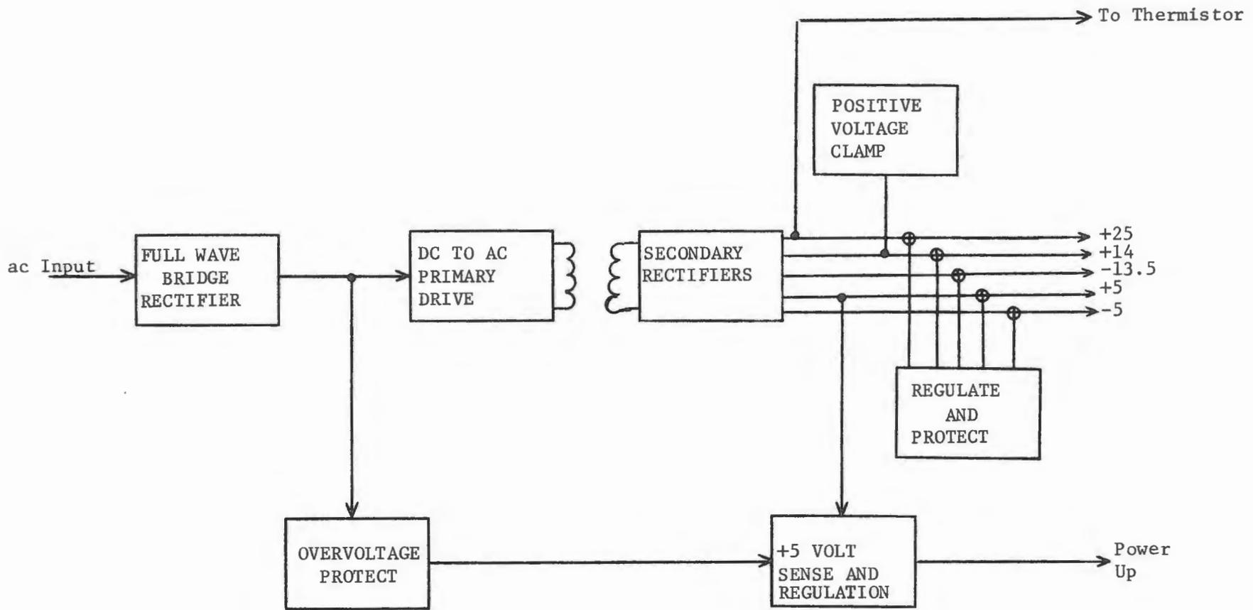
Figure 5-15. Simplified Block Diagram Power Supply
