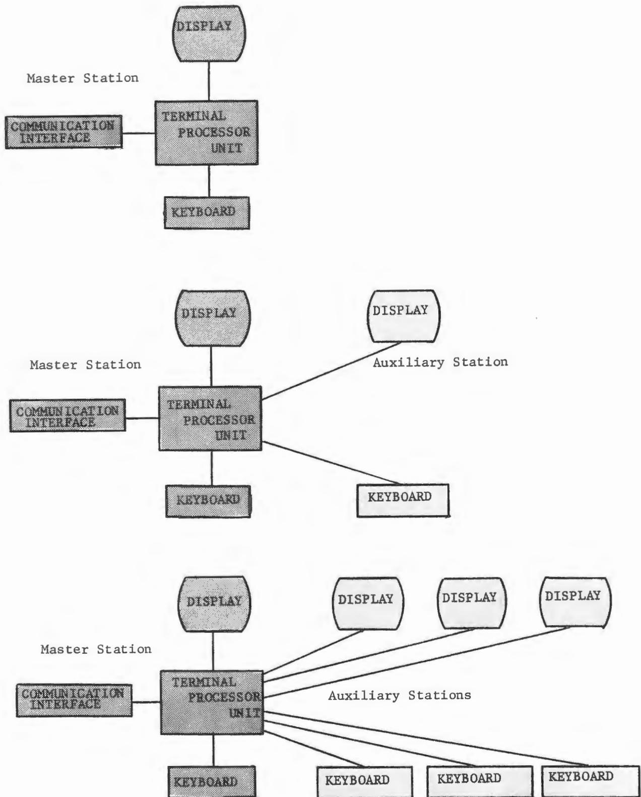
Figure 1-1. Minimum Terminal Configurations
