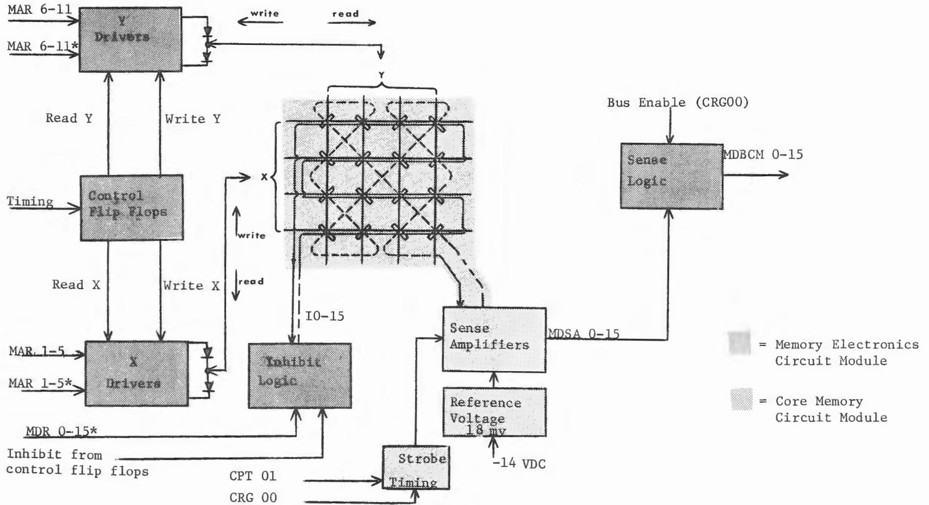
Figure 5-9. Simplified Block Diagram, Memory System
