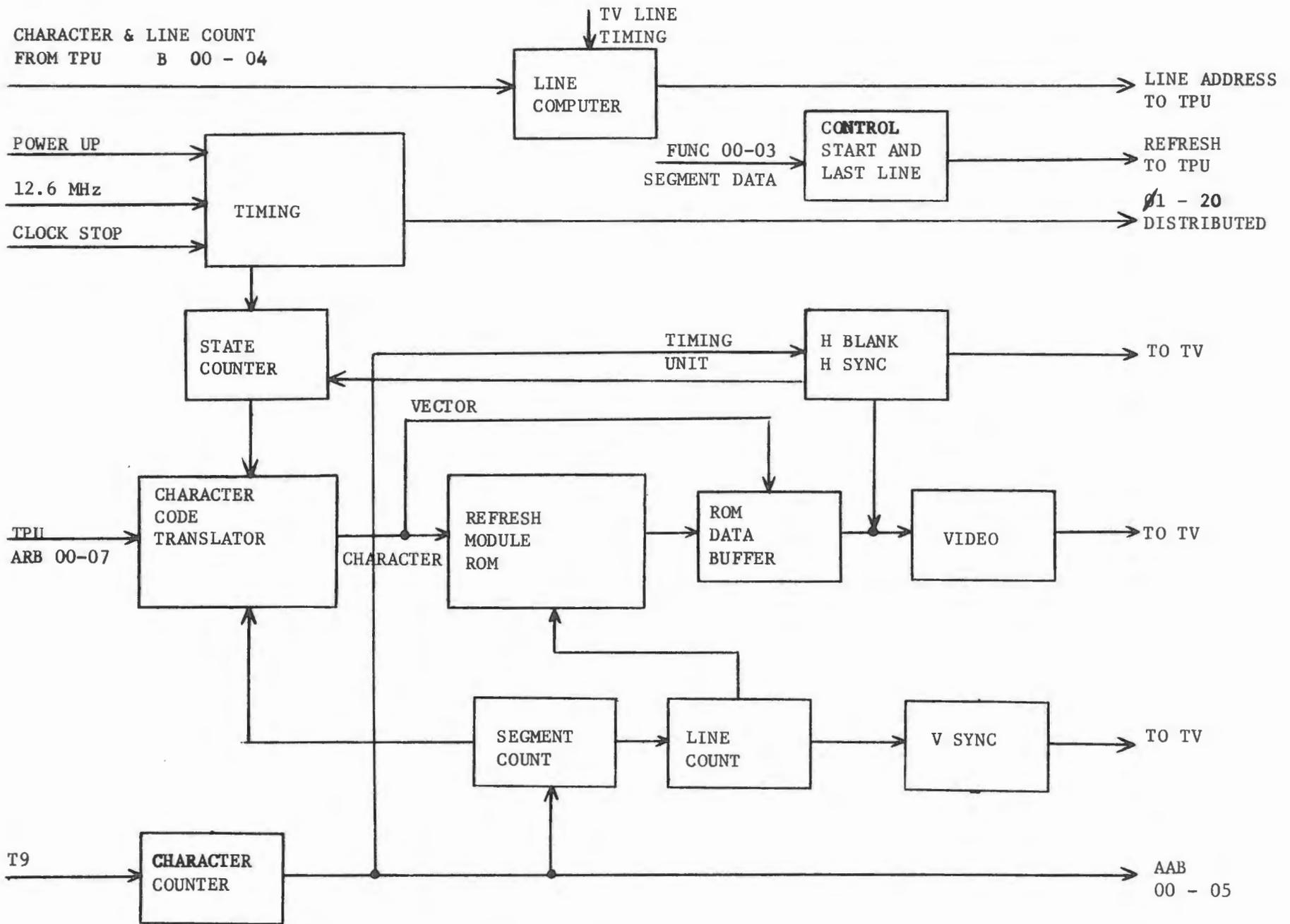
Figure 5-13. Simplified Block Diagram Refresh Module Timing Unit
