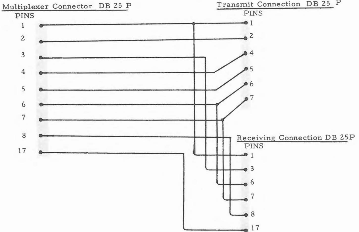
Multiplexer to FDT synchronous or asynchronous controller, HALF Duplex operation.
