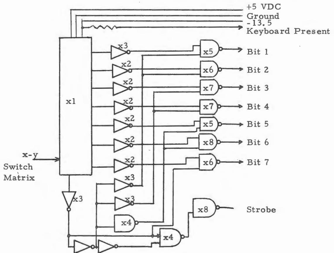
Figure 3. Simplified Block Diagram
