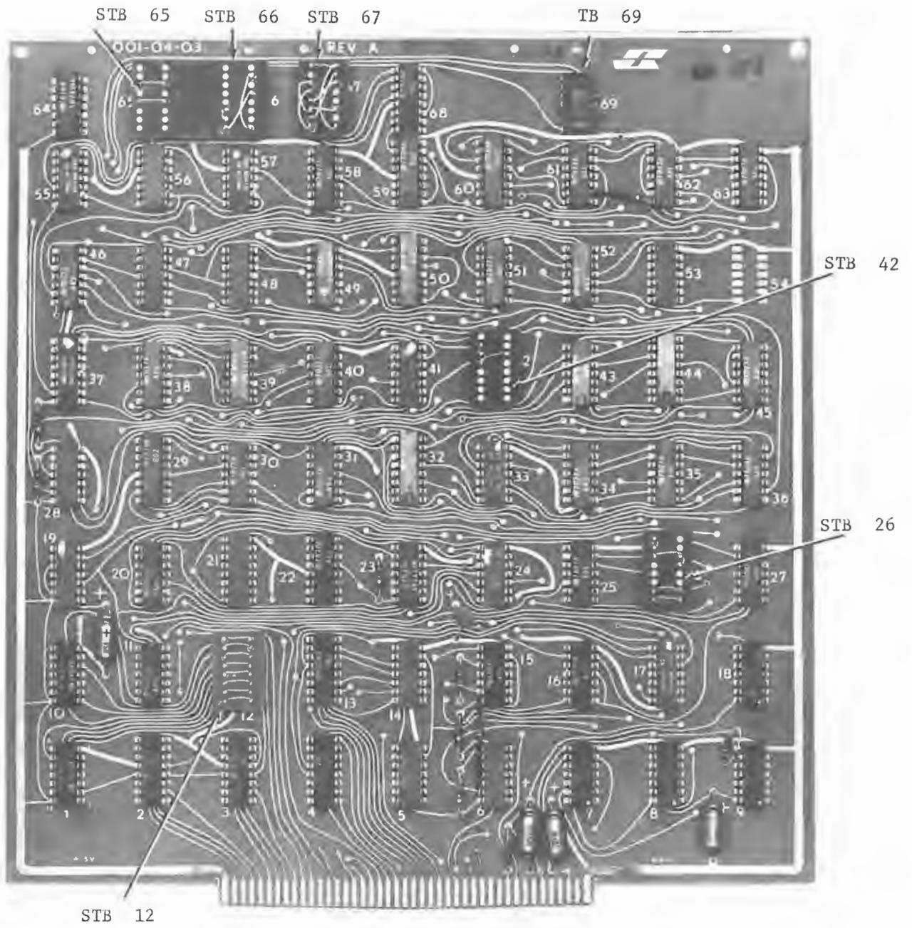
Figure 6-5. Asynchronous Controller
