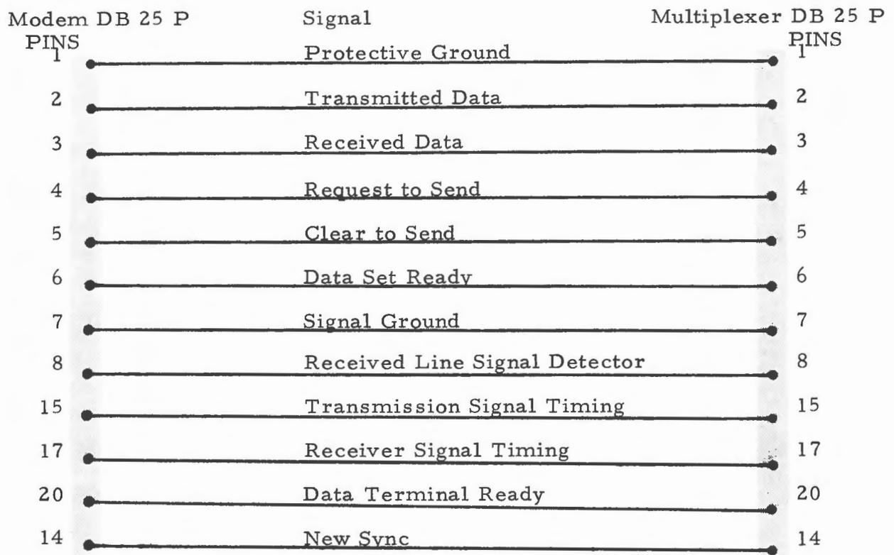
Multiplexer to FDT synchronous or asynchronous controllers. Full duplex operation.
