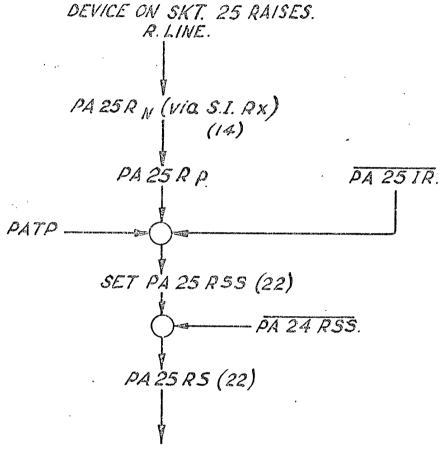
THIS SIGNAL ENABLES ALL CONTROL LEVELS RELEVANT TO THIS PERIPHERAL SOCKET & FROM THIS INFORMATION THE NEXT STEP TO BE PERFORMED IS SELECTED.
