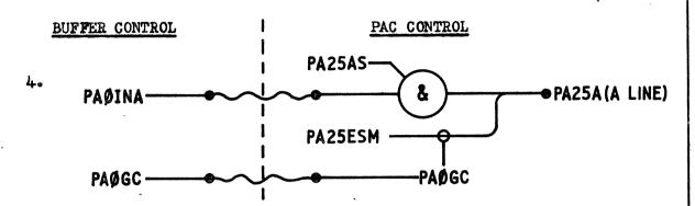
When a command sent to a peri, all 'A' lines of peris connected to a buffer are inhibitted except the 'A' line of the peri receiving the command.
