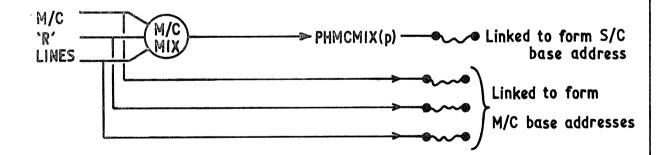
If any M/C 'R' line active, PHMCMIXp active inhibitting S/C Base address of 256. The 'R' line raised via linkwiring generates the desired base address.
