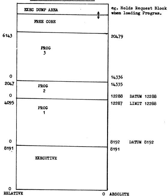
To protect program areas a DATUM & LIMIT system is used. Any object program must address within its prog. area. Any address must be ≥ DATUM & <LIMIT.
