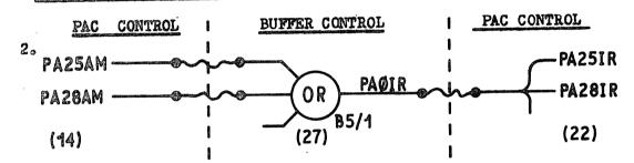
When any peri of a group connected to BUFFER 'Y' is addressed, the 'R' lines of ALL peri's in the group inhibited.
