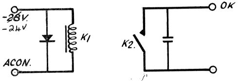
K1.- CONTACTS CLOSE IMMEDIATELY ON ENERGISING OPEN AFTER 5~180 SECS ON DE-ENERGISING.
