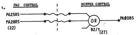
Peri RS levels connected into relevant Buffer control.
