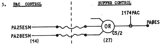
When command sent to device, address decoder gives PAxxESM. This signal passed to relevant BUFFER control.
